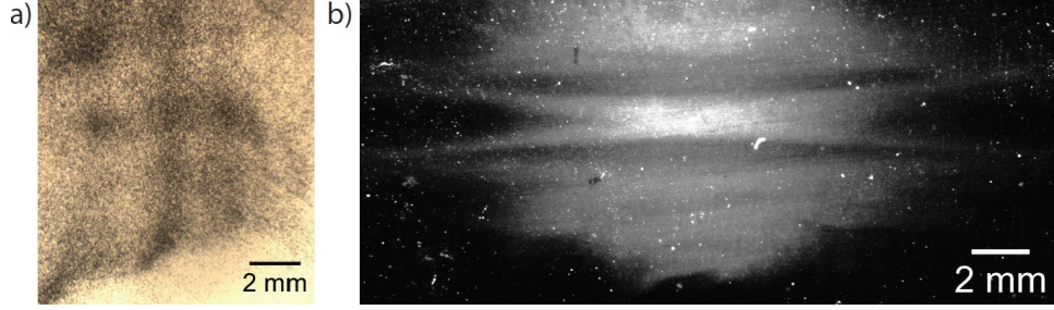
Figure 5.4: Microscope image of CR-39 located 1 cm from a mesh target (a) showing mesh pattern in the proton distribution. Scan of CR-39 from a wire target (b) showing a line focusing feature in the proton distribution 1 cm behind the target. The orientation of the focused line was perpendicular to the orientation of the wire target. This feature was also observed 5 cm behind the target with the same angular divergence.
