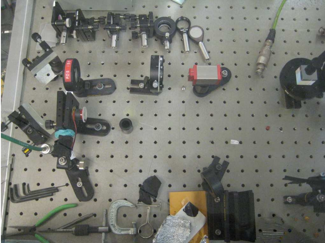
Figure 2.10: Optical table layout with Fabry-Perot cavity and Pound-Drever-Hall locking for phase camera. Faraday isolator and polarizing beam-splitter at upper right; piezo-electrically-actuated mirror at center left. Difficulties with stability, despite a plexi-glass enclosure and floated table, meant that locks were fractions of a second at most, hampering efforts.
