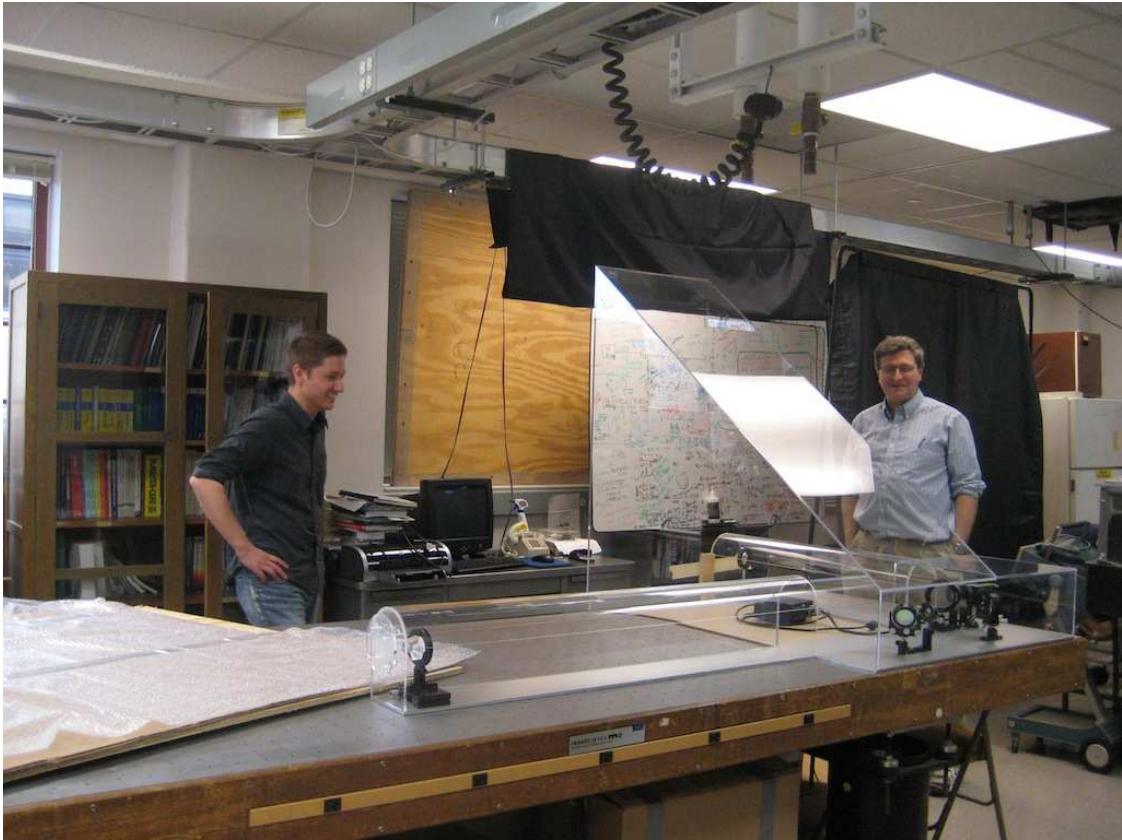
Figure 7.6: Interferometer assembly in Ann Arbor, Michigan. Projection screen not yet installed. Note the outer end of the Y-arm (bottom left of photo), with perforated-and-covered plexiglass to allow sound passage. Humans ( e.g. , Evan Goetz at left, Keith Riles at right) can be protected during alignment processes by laser safety curtains, seen in back.
