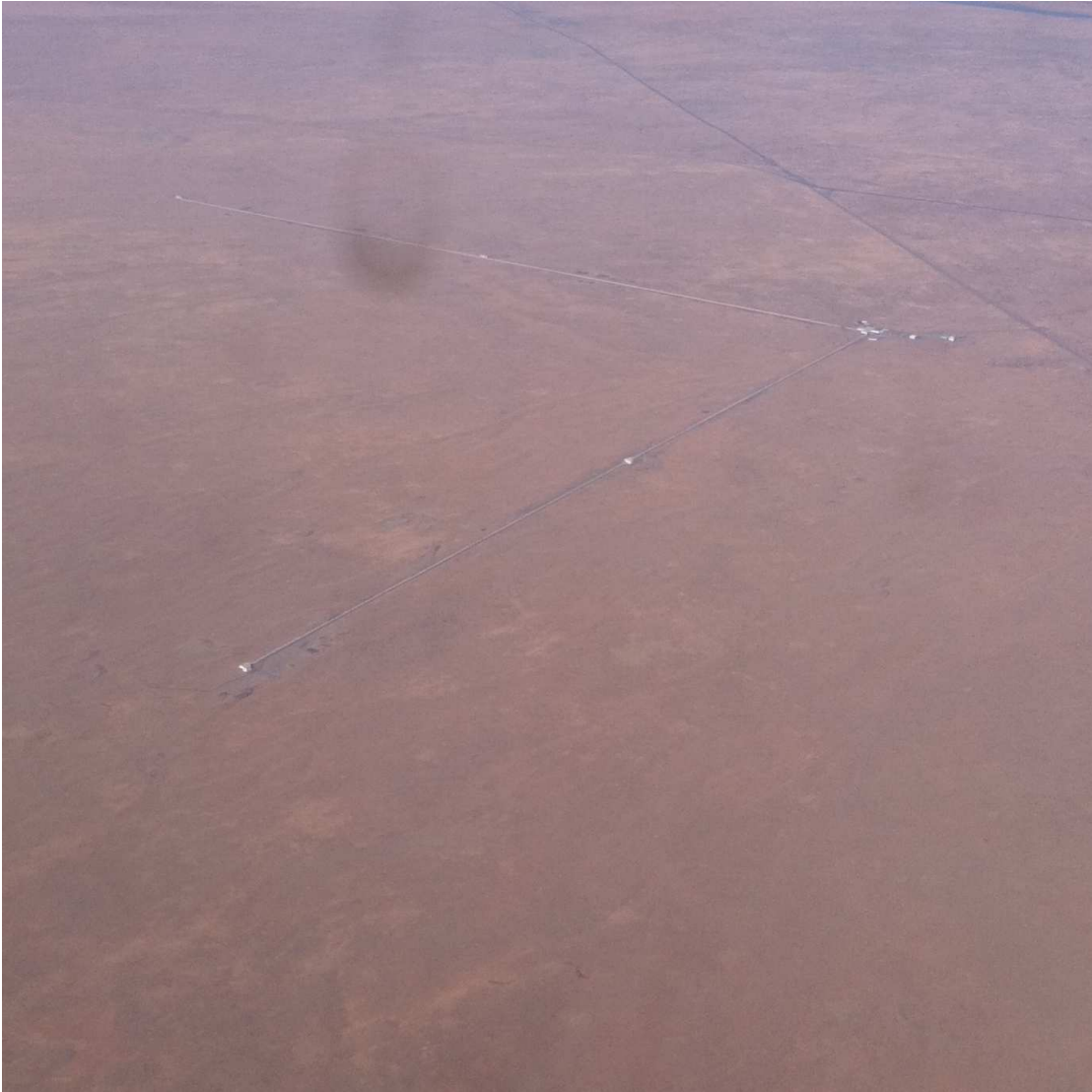
Figure 1.2: View closer to LIGO Hanford Observatory. Ripples in the plain catch wind. The corner station connects the X and Y arms, 4 kilometers long, which each have a mid- and end-station. The corner station also contains the laser, beam-splitter, and photo-detector of the gravitational wave interferometer.
