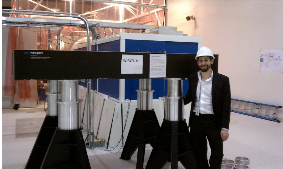
Figure 4.3: Table legs testing. The squeezer table is raised to its final height by the leg extensions. From top to bottom: table (WISCT10), existing leg extensions (with flanges), new leg extensions (flangeless), triangular high table legs. This assemblage provided the squeezer a serendipitously-stable (as measured by Sheila Dwyer, Sheon Chua, and Robert Schofield) platform at low cost. Photo in temporary location; the actual squeezer table was anchored to these table legs, grouted, by HAM4.
