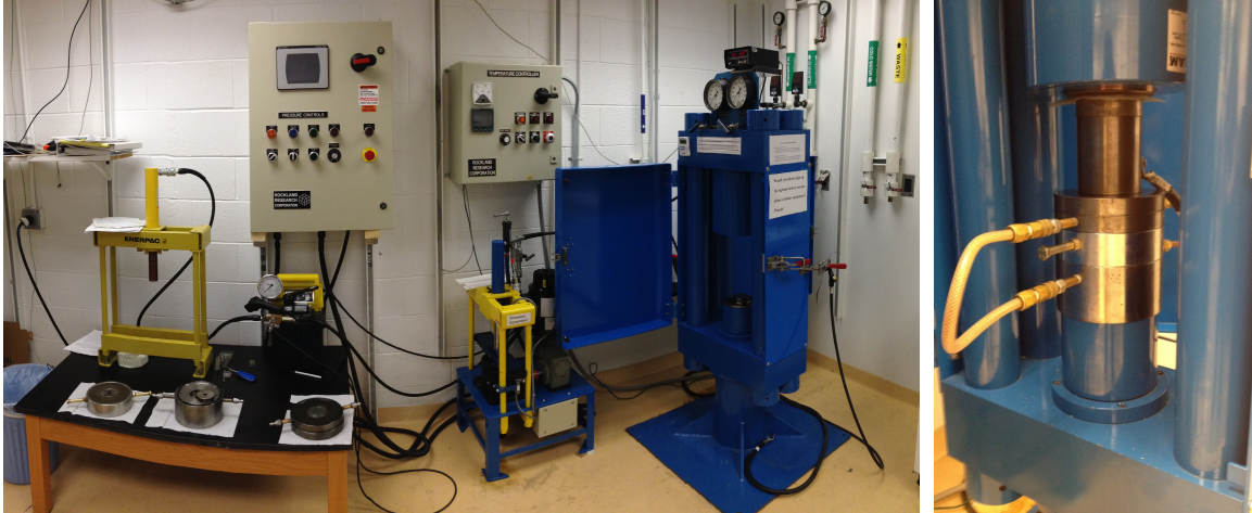
Figure B.7: (Left) Piston cylinder lab. (Right) Close up of piston cylinder assembled.
