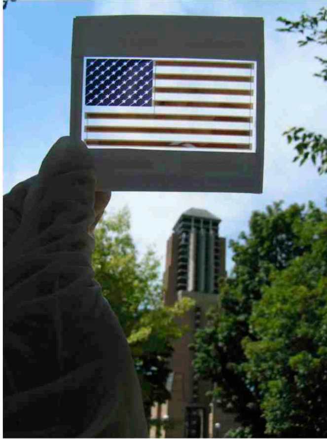
Figure 4.8. The demonstration of the electric power-generating national flag of the United States of America (U.S. flag): Photograph of the U.S. flag taken at the University of Michigan campus shows distinct blue (6 nm) and red (31 nm) color patterns.
