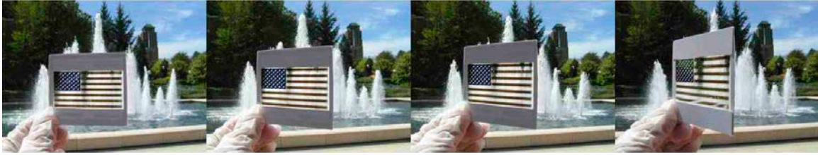
Figure 4.9. The demonstration of the electric power-generating national flag of the United States of America (U.S. flag): According to angle insensitive property, the U.S. flag maintains its colors at oblique angles of incidence up to about 60^\circ , manually controlled.
