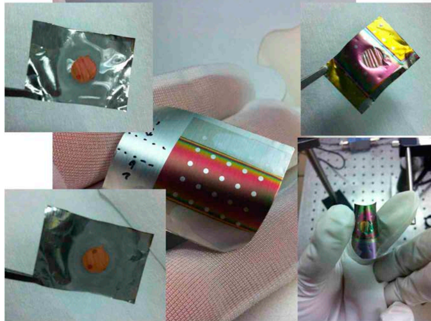
Figure 5.16. The images of Al-foil substrate based undoped a-Si hybrid photovoltaic devices: The random light scattering surface morphology of Al-foil is used after etching of the Al-foil substrate (shown as round shaped on the Al-foil in the images).
