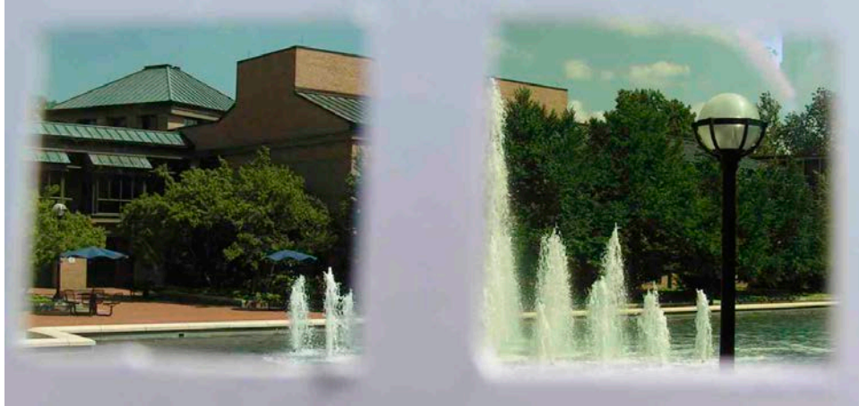
Figure 6.14. The images of the left window-1 (Ag 12 nm) and the right window-2 (Ag 16 nm): The window-2 shows a little yellowish transparency compared to window-1.
