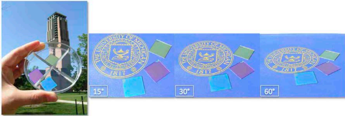
Figure 4.14. Light incident angle behaviors for reflective colors: Images of the fabricated devices showing obvious CMY colors. The colored cells clearly demonstrate the angle insensitive performance at large angles of incidence ( 15^\circ , 30^\circ , and 60^\circ ).
