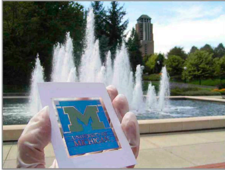
Figure 4.19. The demonstration of the electric power-generating U of M logo: Photograph of the U of M logo panel consisting of maize and blue colors, which is successfully realized with generating electric power.
