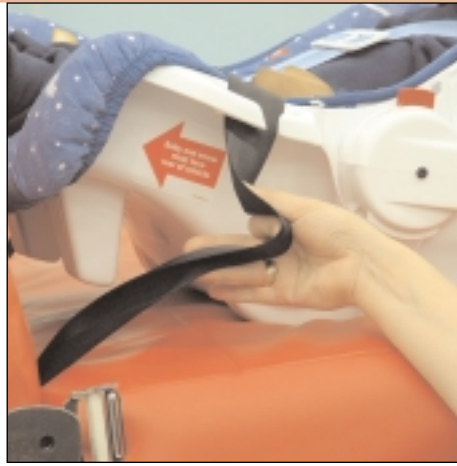
The car seat is too loose. When properly installed, there should be only one inch of side-to-side movement of the child restraints, relative to the vehicle.
