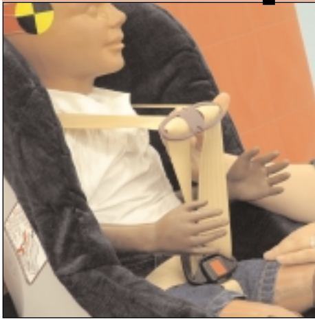
The harness is too loose. In order to prevent ejection, the harness should be tightened snugly on the child's body.
