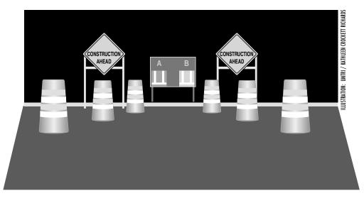
FIGURE 2. A diagram of the cluttered condition for evaluating the selection of retroreflective materials used in roadworker safety vests.
