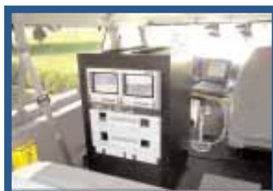
above left: Lightweight profiler used for assessment of new construction roughness, Dynatest/KJL6400.
