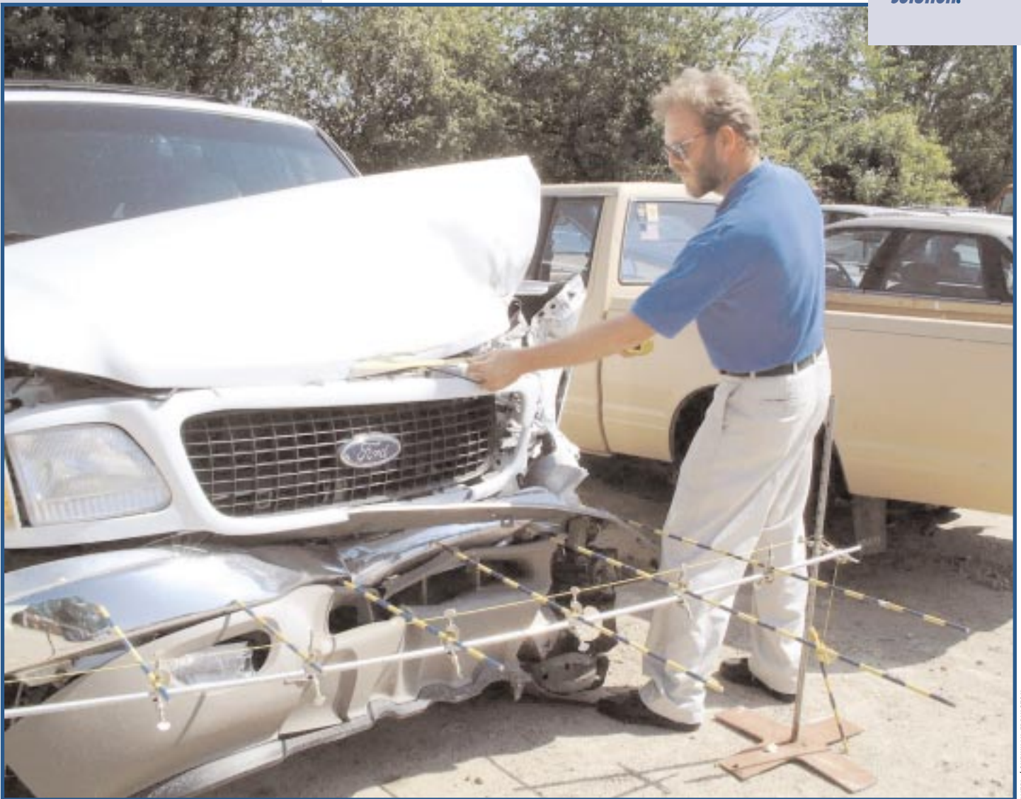
Joel MacWilliams takes measurements of a frontal collision.
