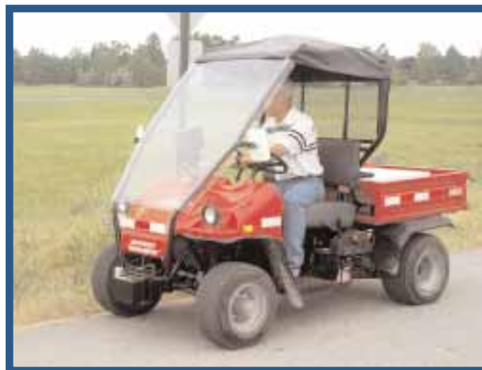
above left: Lightweight profiler used for assessment of new construction roughness, Dynatest/KJL6400.
