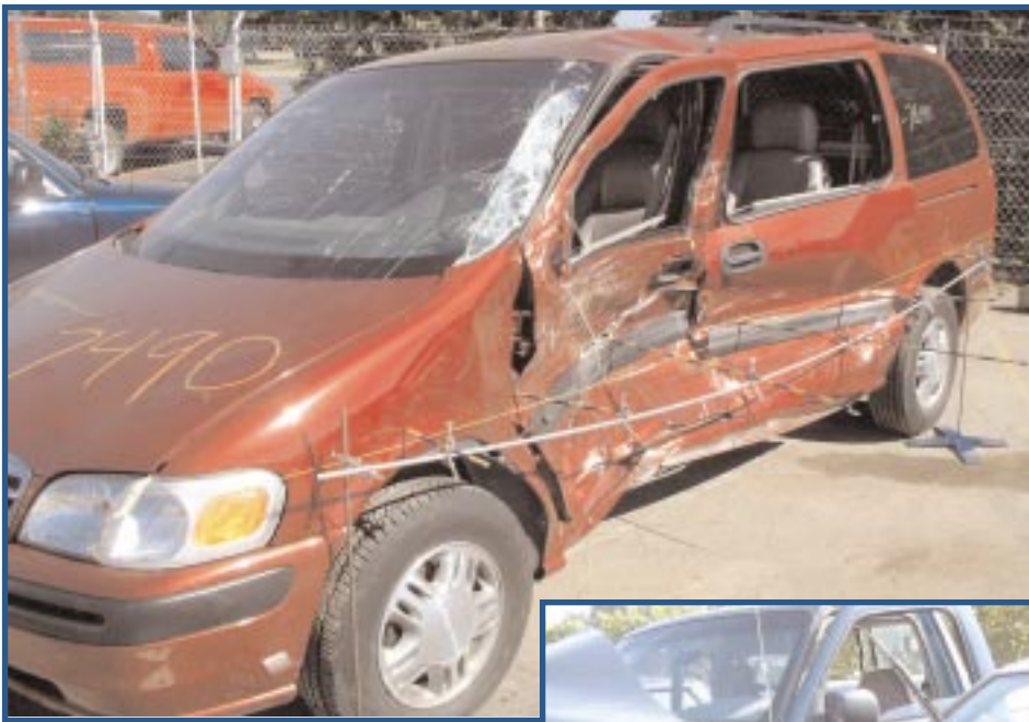
Left: A real-world side impact that typically causes moderate to severe injuries for the near-side occupants.
