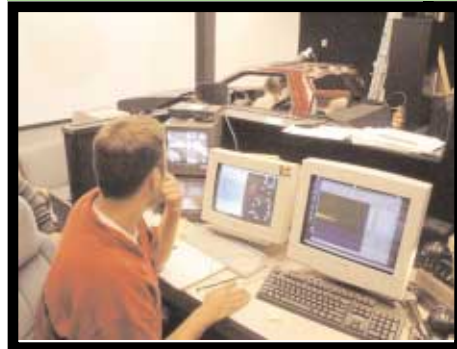
During the test runs, researchers monitor and record driver reactions, speed, location of the vehicle on the road, and many other factors.
