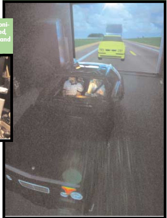
The back screen shows the view the driver sees in the rearview mirrors.
