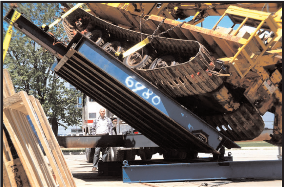
UMTRI researchers conducted a tilt test on a GoTract, a device that installs telephone utility poles, to help validate a software model.
