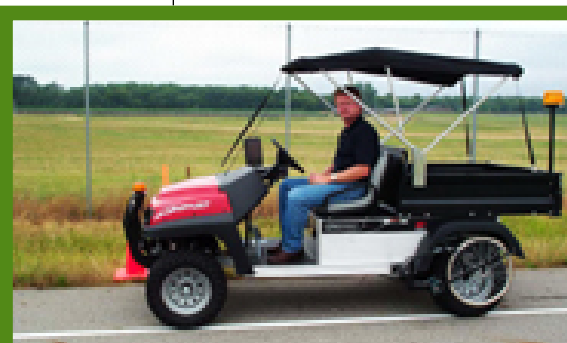
A lightweight profiler manufactured by Surface System Instruments is tested at a site in Lansing, Michigan.
