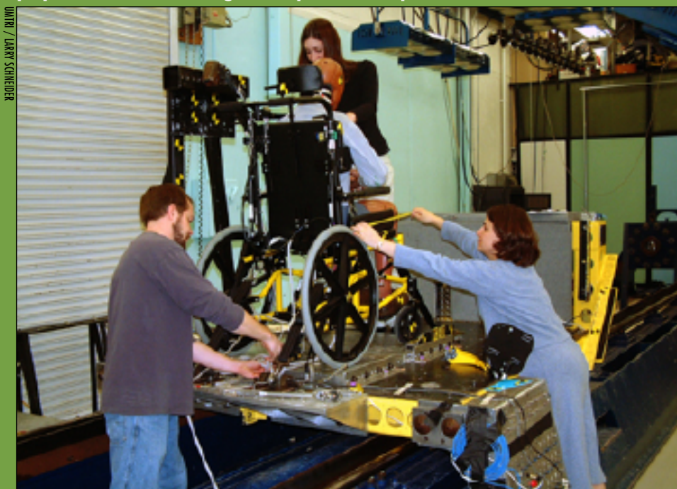
Left to right: Charlie Bradley, Amy Klinkenberger, and Miriam Manary make final preparations for conducting a 30-mph frontal-impact test of a wheelchair.
