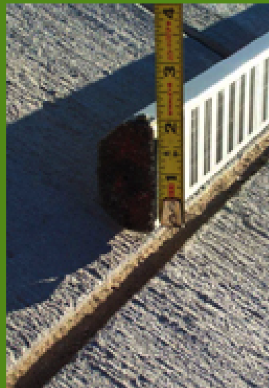
A rod used in the rod and level method of pavement measurement at a site in Bay City, Michigan.
