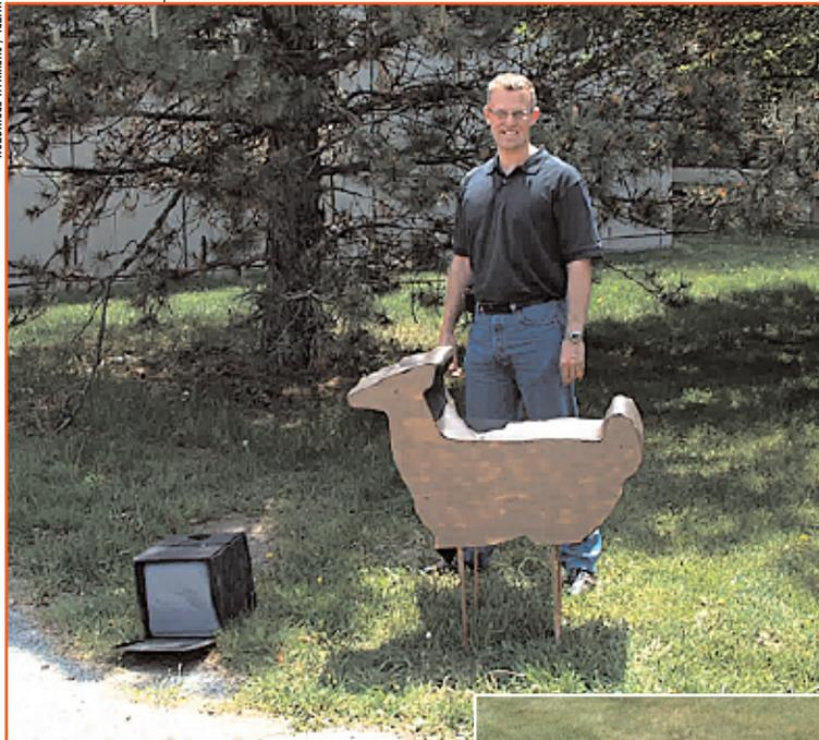
**Jonas Bärgrman poses with the deer target and the final version of the small animal target, which consists of a gray plastic container filled with warm water, enclosed in a three-sided black box. This view shows the box and its concealing shroud.**
