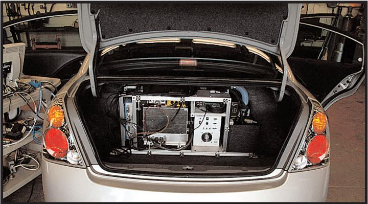
Much of the hardware needed for the lateral drift and curve warning systems is housed in the trunk of the test vehicles. The equipment is hidden behind a panel that subjects are asked not to remove.
