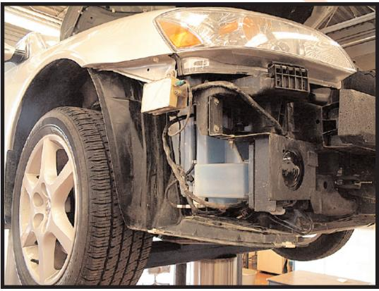
The forward radar detects road-side objects ahead of the vehicle that may constrain the maneuverability room available along its projected future path. The side radar detects shoulder-width-reducing objects at the moment that they are adjacent to the vehicle. It also refines the location of objects that were detected moments earlier by the front radar and designates them as permanent or temporary objects.
