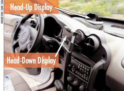
Locations of the head-up and head-down night vision displays in the test vehicle.
