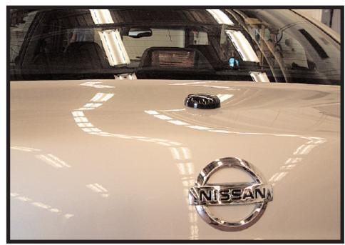
The curve speed warning system uses global positioning system (GPS) data and a precise, on-board map database to determine the current vehicle position, the most likely future path, and the geometry of the road along that path. The GPS antenna is visible on the test vehicle's trunk.
