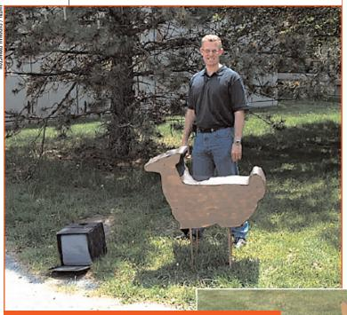
Jonas Bärgman poses with the deer target and the final version of the small animal target, which consists of a gray plastic container filled with warm water, enclosed in a three-sided black box. This view shows the box and its concealing shroud.
