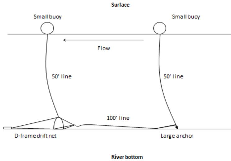
Fig. 2 – Sampling design for conical net sets used to capture larval lake sturgeon, from D'Amours et al. 2001
