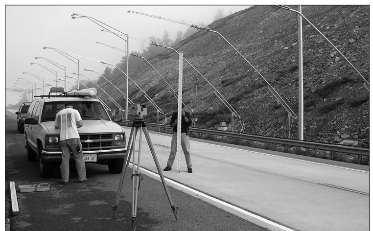
Digital level used for reference measurements.
