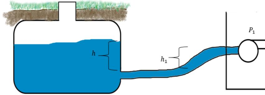
**Figure 6.** Figure showing the fluid flow from cistern to pump used to determine the governing equation of the pressure sensor.
