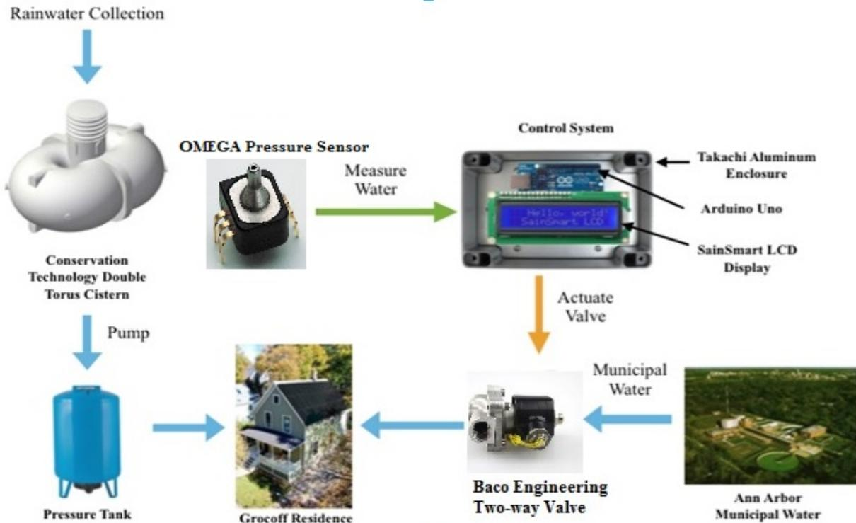
**Figure 4.** Final concept mock-up detailing sensor, control system, and valve components and function of each component to switch water sources.
