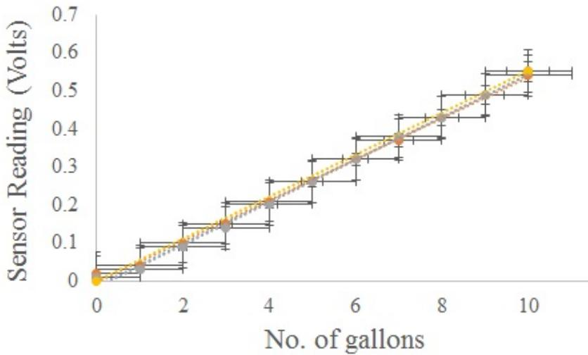
**Figure 8.** The calibration curve for the 10-gallon water tank resulted in 55.2 mV per gallon.
