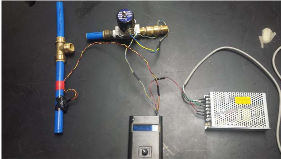
**Figure 5.** A photograph of our final prototype. The Arduino, LCD, H-Bridge, and Rotary Encoder are all in the enclosure. The pressure sensor is attached to a length of pipe for testing. Additional pictures can be found in appendix E.
