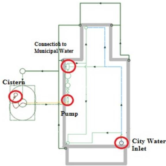
**Figure 2.** The LBC team has drawn a schematic of the home with pertinent components. Our control system will have to function in four main areas of the net-positive system: monitoring the water level in the cistern; switching the pump on/off; actuating a valve to change the water source; directing water flow from the inlet of municipal water.
