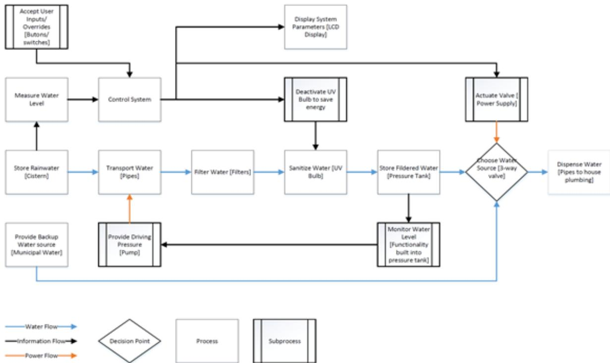
**Figure 3.** Our functional decomposition includes the flow of water (blue lines), the flow of power (orange lines), and the flow of information (black lines). Each block represents a specific function that our control system should be able to complete.
