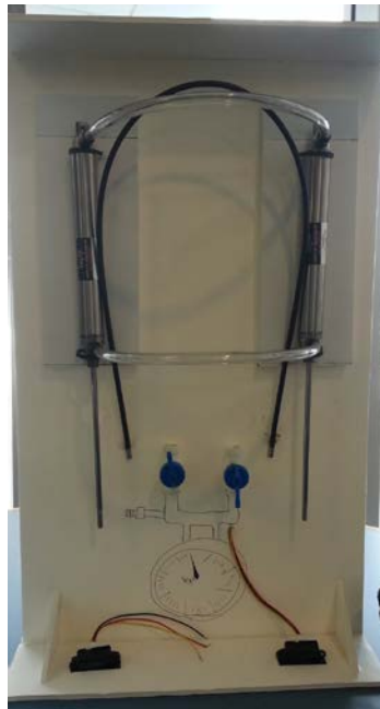
Figure 12: Foamcore mockup of our proposed test rig incorporating cylinder, a Bowden cable conduit, and sensors.
