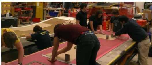
Figure 47: Carbon fiber being cut to proper size and orientation using stencils (25).
