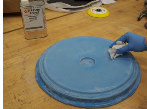
Figure 24: Application of no-sand primer to test mold.
