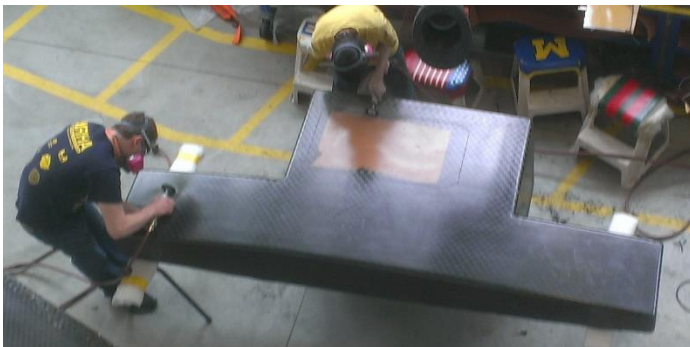
Figure 49: Cured carbon fiber component being rough trimmed with hand tools (25).
