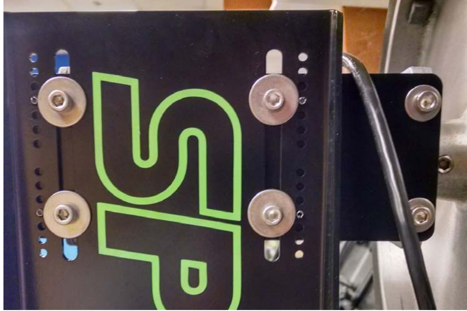
Fig. 20: Notches allow wheel spacing to be adjusted to accommodate balls of various sizes.
