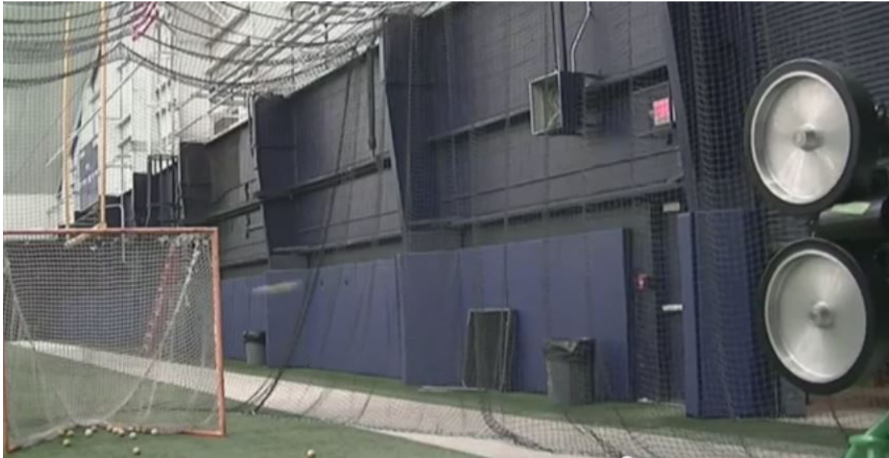
Fig. 19: Launcher test setup. Goal is approx. ten yards from launcher, both enclosed in batting cage net.
