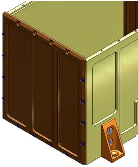
Figure 7B. Attachment of Front Plate (orange)
