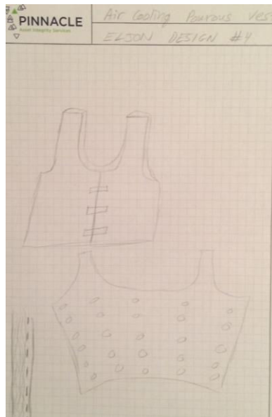
Figure A.4: E4 – Internal-suit air-based porous cooling.
