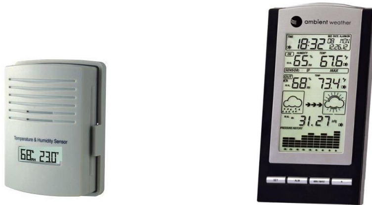
Figure 36: Chest mounted, remote thermometer & humidity sensor (left) and WS-1173A Wireless Advanced Weather Station apparatus (right) used for measurement purposes throughout the duration of the experiment.
