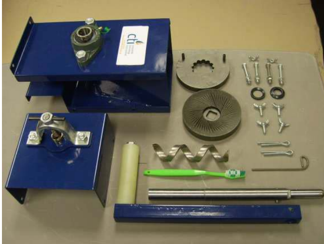
Figure 5: Disassembled view of grinder shows all of the parts included in product.
