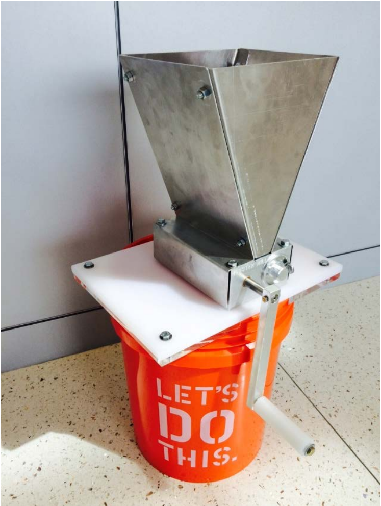
Figure 25: Final Breadfruit Grinder prototype
