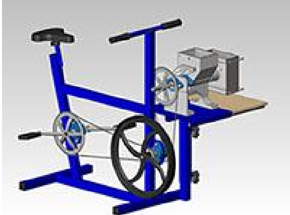
Figure 3: CAD model of CTI's breadfruit grinder. The foot-pedals are geared to the grinder on the right.
