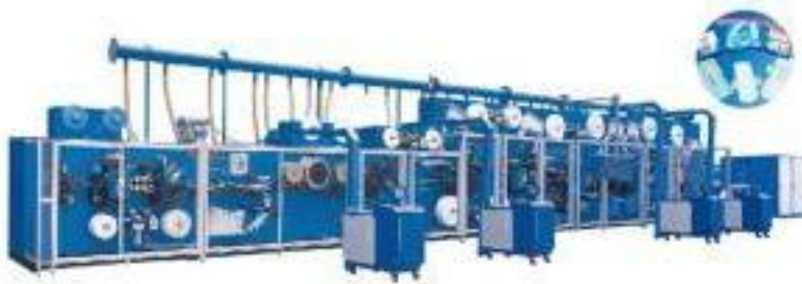
Figure 3: Diagram of Large Scale Production Sanitary Pad Machine DC-SN-500
