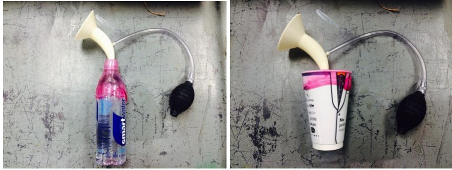
Figure B-4. Left figure is the smallest bottle cap size (regular water bottle) that the cover could fit, which is 1.1 inch; right figure is the largest bottle cap size (the coffee cap) the cover could fit, which is 3.5 inch.
