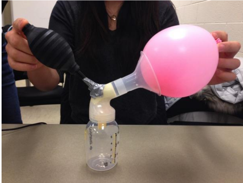
Figure 22. Experimental setup for empirical testing of the suction mechanism
