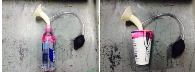
Figure 30. Left figure is the smallest bottle cap size (regular water bottle) that the cover could fit, which is 1.1 inch; right figure is the largest bottle cap size (the coffee cap) the cover could fit, which is 3.5 inch.
