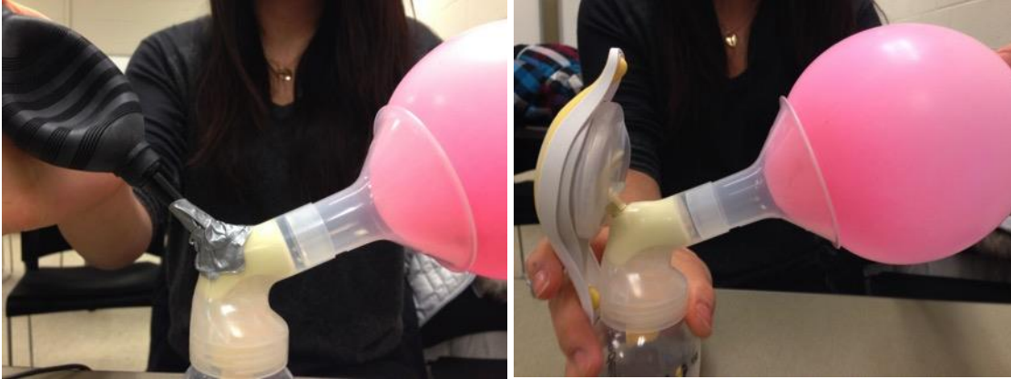
Figure 23. The left figure shows that the squeeze pump generated suction inside the suction cup, in comparison with the suction generated using the Medela pump on the right figure.
