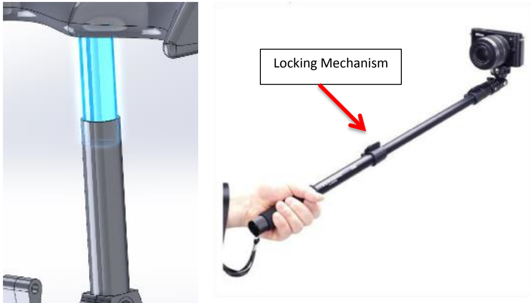
Figure 18: SolidWorks rendering of our telescoping bar component (left) and purchased component to perform this function (right). This component will be able to telescope to adjust the length of the restraint to fit the child better.
