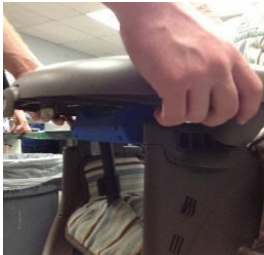
Figure F1: The lap bar in the upright position prevents the tray from being attached. This promotes the use of the restraint while the high chair is being used.
