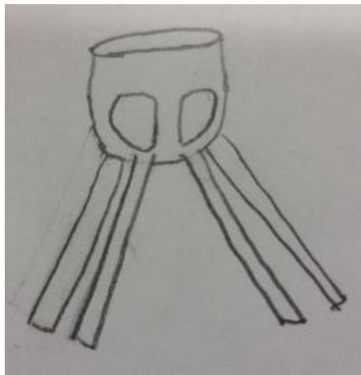
Figure A15: Leg holes in chair with a deep seat making it difficult for the child to achieve enough leverage to raise itself out of the chair by itself
