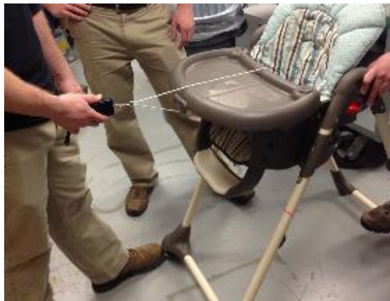
Figure F7: Demonstrates the tray integrity test
