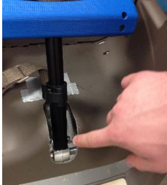
Figure F2: Manually testing our high chair for sharp points
