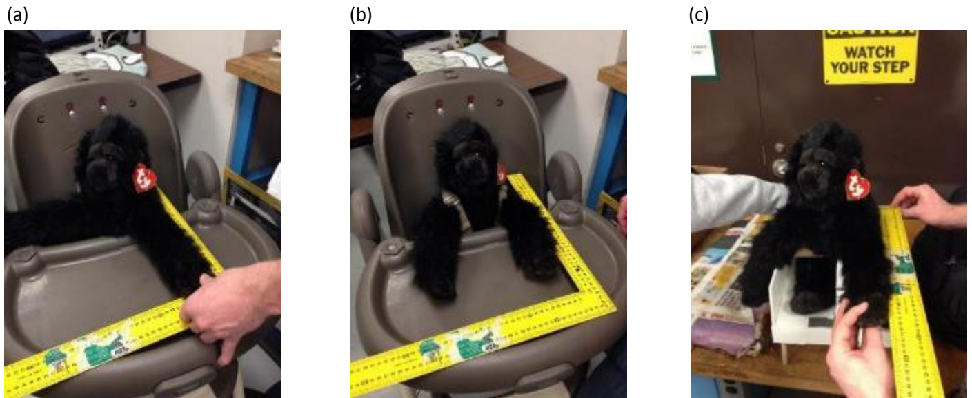
Figure 15: We used a stuffed animal gorilla as a model for a child. (a) We measured the distance from the back of the chair to the model's fingertips when the model was not restrained. (b) The model was restrained with a five point harness and the measurement was repeated. (c) The model was restrained with our mockup lap bar and the measurement was repeated.
