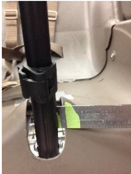
Figure F3: (a) Demonstrates our measuring of pinch points on the high chair classified by ASTM standards. (b) An example of a solution to the pinch point problem by covering the slot with a rubberlike material.
