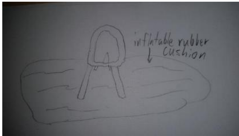
Figure A14: Inflatable mat on floor around high chair that gives the child a soft surface to land on if it falls
