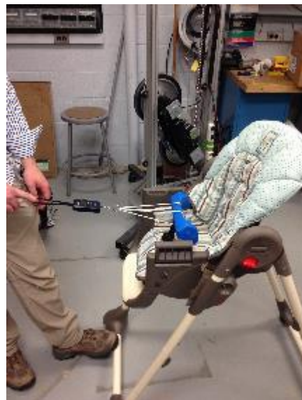
Figure F4 & F5: Figure F4 (Left) demonstrates the vertical pull test. Figure F5 (Right) demonstrates the horizontal pull test.
