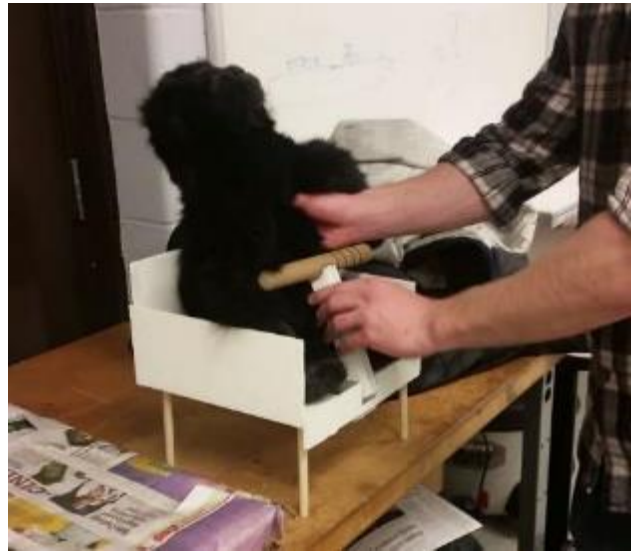
Figure 16: We used a stuffed animal gorilla as a model for a child. (a) We measured the time it took to restrain the model using a five point harness. (b) We then measured the time it took to restrain the model using our mockup of our lap bar restraint.
