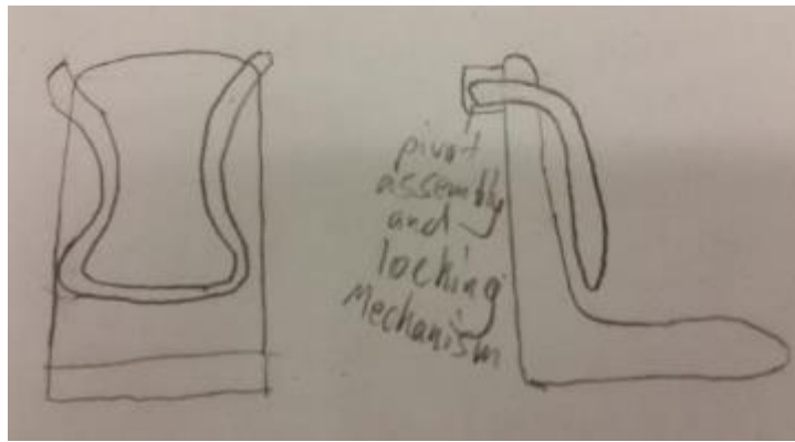
Figure A6: Overhead Roller Coaster-like Restraint that pivots from the top back of the chair and will restrain at waist and shoulders while leaving the arms free.
