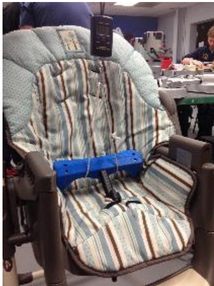
Figure F4 & F5: Figure F4 (Left) demonstrates the vertical pull test. Figure F5 (Right) demonstrates the horizontal pull test.
