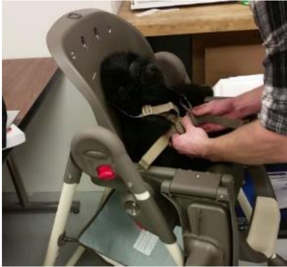
Figure 16: We used a stuffed animal gorilla as a model for a child. (a) We measured the time it took to restrain the model using a five point harness. (b) We then measured the time it took to restrain the model using our mockup of our lap bar restraint.
