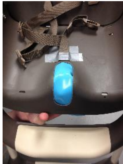
Figure F3: (a) Demonstrates our measuring of pinch points on the high chair classified by ASTM standards. (b) An example of a solution to the pinch point problem by covering the slot with a rubberlike material.
