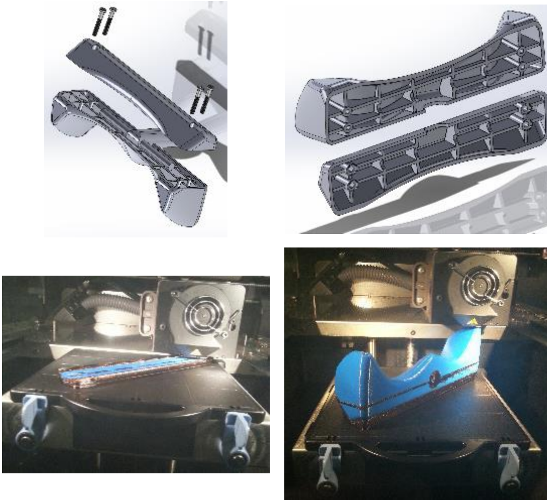
Figure 17: SolidWorks rendering of our lap bar component assembly (top left) and inside (top right). The lap bar is highly contoured to comfortably fit children of ages ranging from four months to two years. The bottom two pictures show the progress of the lap bar being 3D printed.
