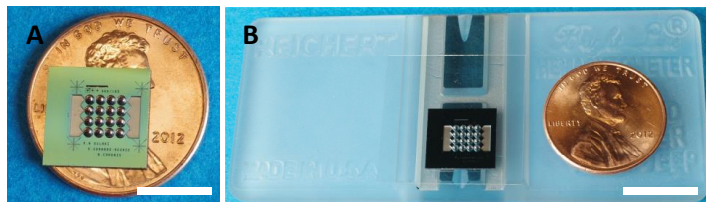
Figure 5.2: \mu OIL chip (1 cm x 1.2 cm) on US penny (A) and the \mu OIL chip/ haemocytometer assembly (B). Scale bars, 1 cm in A,B.
