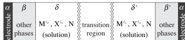
Figure 3.1: Schematic drawing of a general electrolytic cell containing a simple binary electrolyte. M, X, and N are the chemical symbols of cations, anions, and solvent, respectively, and z_+ and z_- are the ionic equivalent charges.
