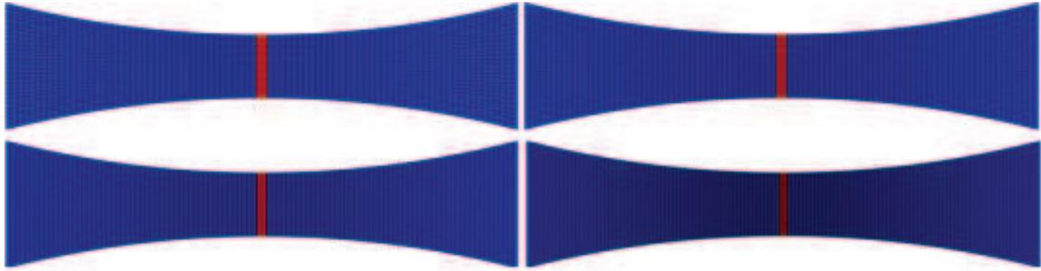
Figure 3.12: Crack path of dogbone shape model of four distinct mesh sizes
