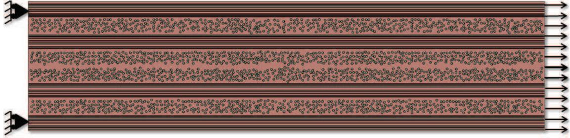
Figure 3.28: Large micromechanics model ( $[0/90]_{2S}$ ) and boundary conditions
