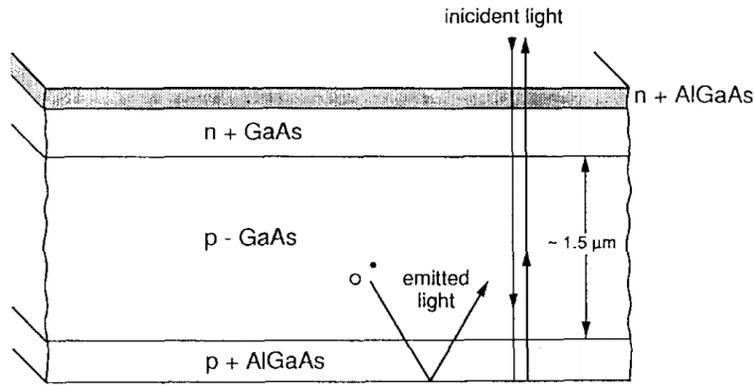
**Fig. 2.15:** GaAs solar cell structure for enhanced photon recycling. Reproduced from ref. 44.
