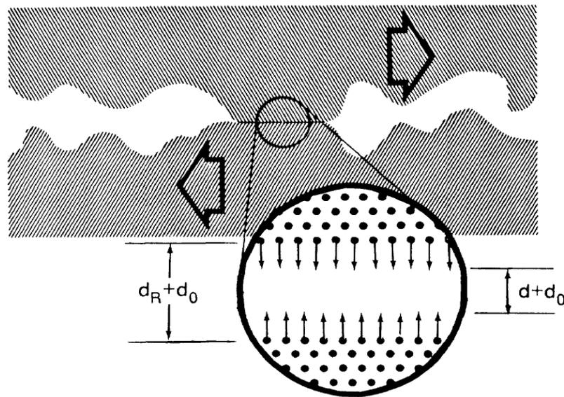
**Fig. 2.10:** Schematic of cold-welding process. When the interfacial separation is below the critical thickness, two metallic surface can collapse together. Reproduced from ref. 31.
