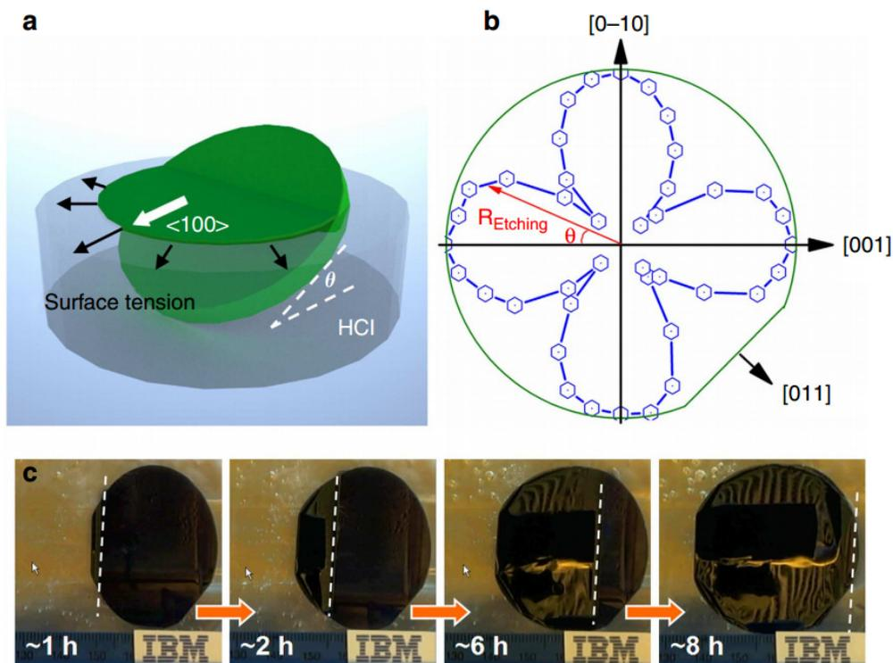
**Fig. 2.37:** Surface tension-assisted ELO process. (a) Schematic of surface tension-assisted ELO process. (b) Crystallographic direction dependent etch rate of AlInP in HCl. (c) Photographs of the surface tension-assisted ELO process. The average lateral etching rate of 5.9 mm/h is achieved. Reproduced from ref. 34.
