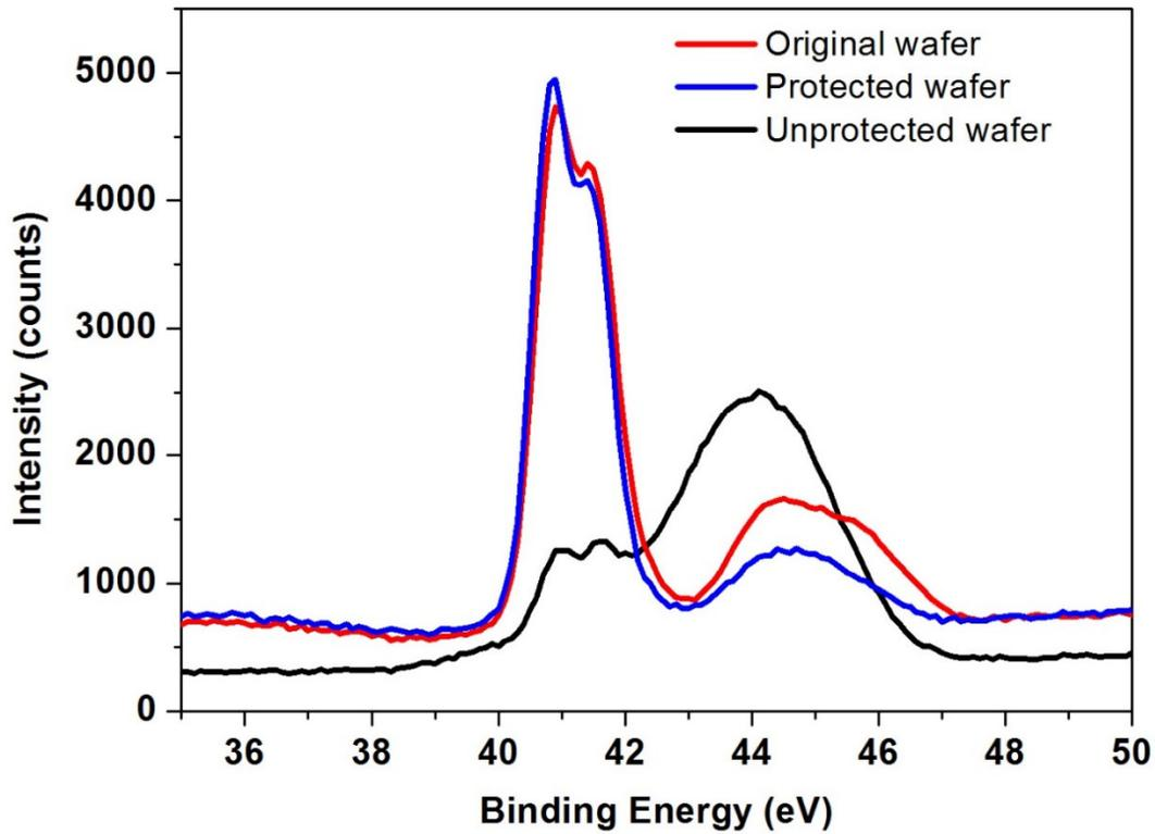
**Figure 6.8:** X-ray photoelectron emission spectra of the samples in Fig. 2 measured using energy dispersive spectrometry (EDS).
