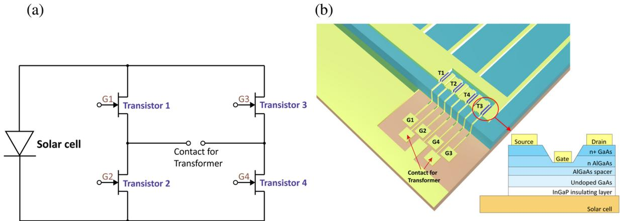
**Fig. 9.6:** (a) H-Inverter circuit plus solar cell array. (b) Monolithic integration scheme of a GaAs HEMT transistor plus solar cell cold-weld bonded to a flexible substrate.
