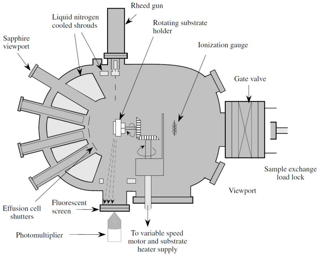
**Fig 1.7:** Schematic of MBE chamber. Reproduced from reference 3.
