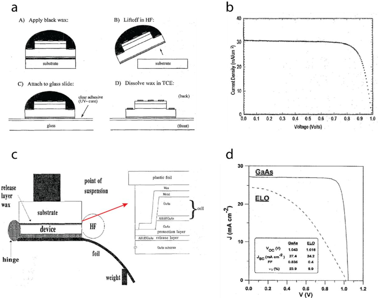
**Fig. 2.20:** ELO processed GaAs thin-film solar cells. (a) ELO process using black wax. Photovoltaic cells were first fabricated, then transferred onto glass substrate. (b)  $J$ - $V$  characteristic under 1 sun (simulated AM1.0) illumination. (c) Schematic of WI-ELO process, and device structure for it. (d)  $J$ - $V$  characteristic comparison between ELO cell and substrate cell under 1 sun illumination. Inset: Summary of device performances. Reproduced from ref. 49 and 50.
