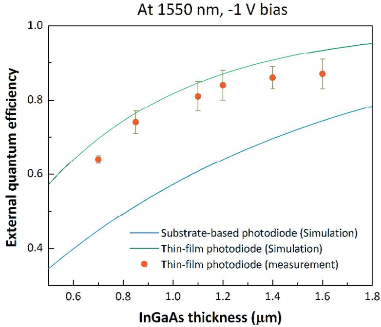
**Fig. 5.5:** Comparison of simulated and measured EQE performance at -1V bias and 1550 nm wavelength between thin-film devices (green line) and substrate devices (blue line) with different InGaAs absorption layer thicknesses, together with the measured EQE performance of fabricated photodiode devices with different InGaAs absorption layer thickness (orange dots)
