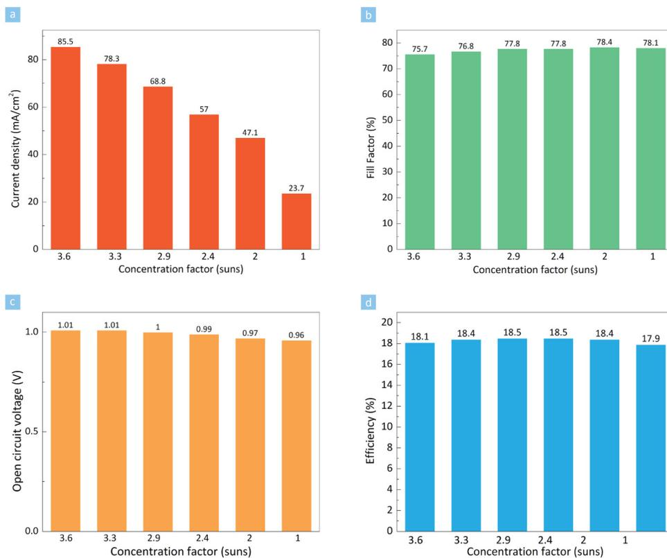
**Fig. 7.7: Performance of the thin-film GaAs solar cells under the concentrated light** (a) Short circuit current (b) open circuit voltage, (c) fill factor, and (d) power conversion efficiency of the thin-film GaAs solar cells under the various concentrated light conditions measured by their integration with the mini-CPCs.
