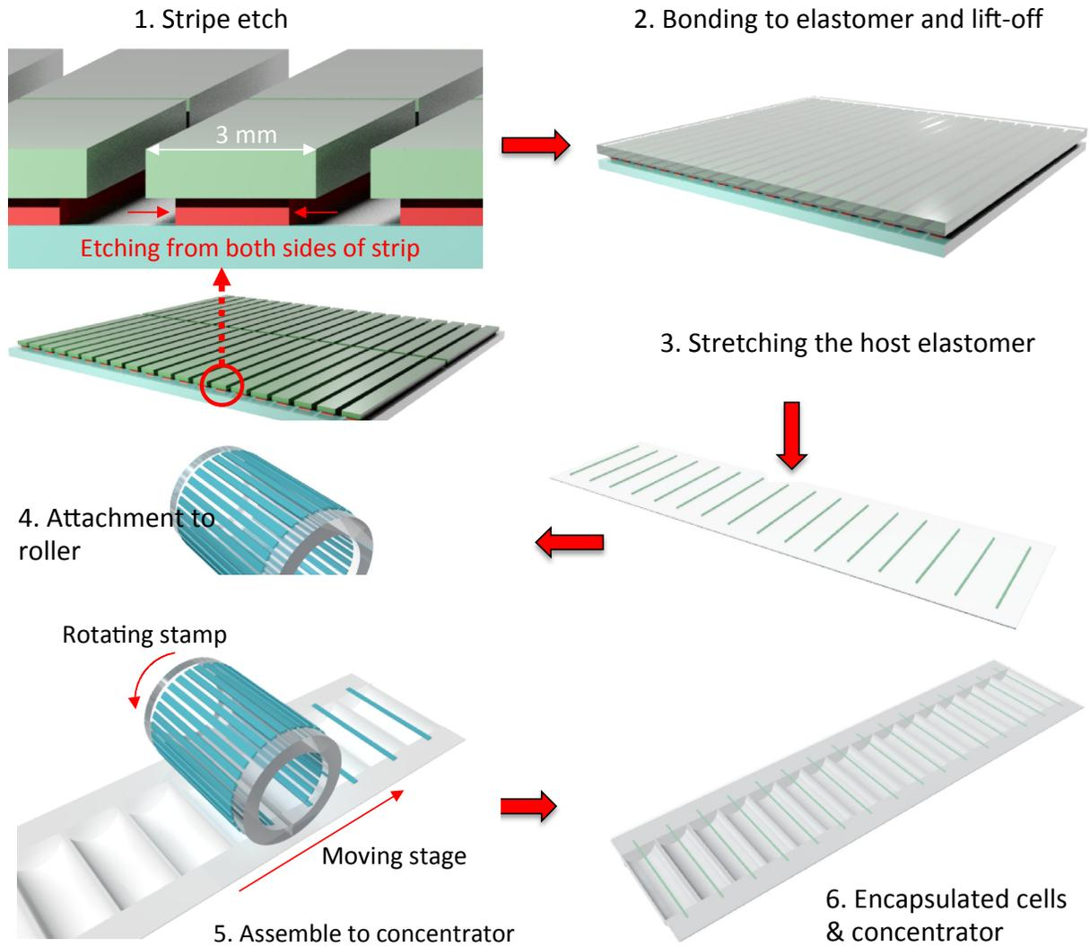
**Fig. 9.3:** Example process flow for fabricating integrated GaAs solar cell/mini-concentrator arrays. 1. Channels are patterned and etched to the sacrificial layer, defining the stripes. 2. Once patterned, the wafer is bonded epi-side to an elastomer and 3. Stretched over the surface of a 4. Roller. 5. The stripes are then cold-weld bonded to the mini-concentrator array (either the top or bottom side) to 6. Form the concentrator/solar cell arrays.
