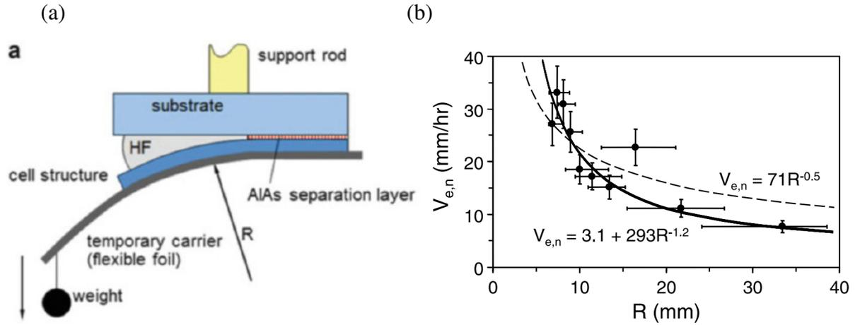
**Fig. 2.5:** Weight induced epitaxial lift-off (WI-ELO) process (a) Schematic illustration of WI-ELO process (b) Lateral etch rate depending on the curvature near the etch interface. Reproduced from ref. 7 and 26.
