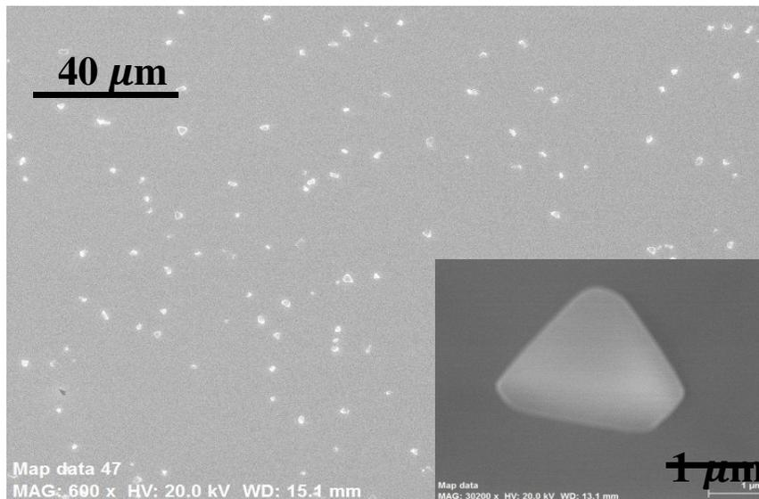
**Figure 6.3:** Scanning Electron Microscopic (SEM) image of an HF exposed wafer surface without protection layers.
