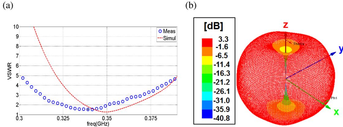
**Fig 8.4:** (a) Measured and simulated VSWR and (b) 3D radiation pattern ( $G_\theta$ ) of the solar antenna.
