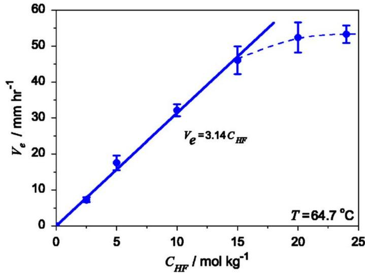
**Fig. 2.3:** Lateral etch rate depending on HF concentration. Solid line indicates the fitting of experimental data based on DR model. Reproduced from ref. 24.
