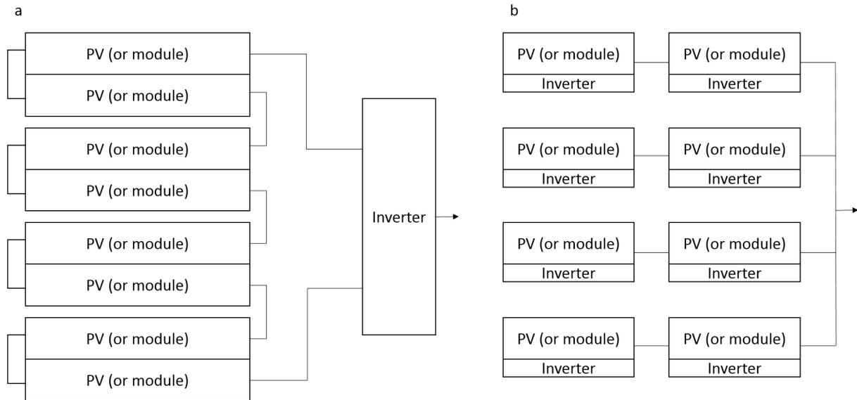
**Fig. 9.7:** Schematic illustration of solar power system (a) Large number of panels connected to a single inverter. (b) Each solar cell or module incorporates its own inverters (known as microinverter system).
