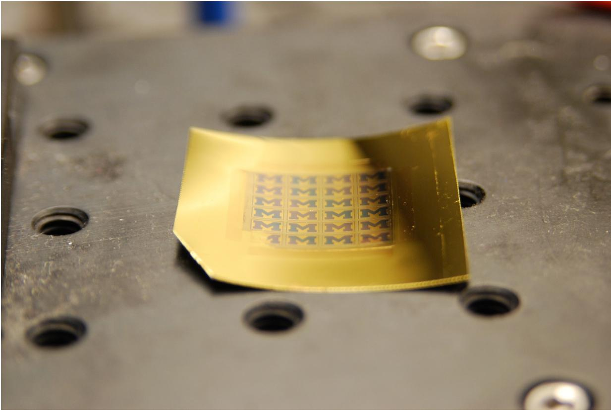
**Fig. 6.17. Thin-film LEDs.** Image of AlGaInP/ InGaP double heterostructure LEDs on a plastic substrate before the epitaxy is bent around a 1.2 cm radius.
