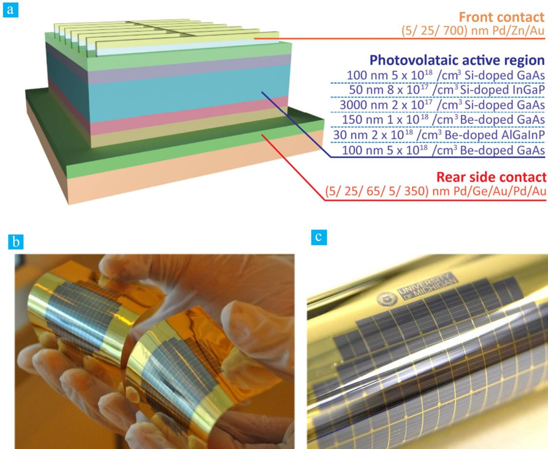
**Figure 6.11:** Thin-film GaAs single junction photovoltaic cells. (a) Device structure of the thin film GaAs *p-n* junction photovoltaic cells. (b) Fabricated GaAs thin film photovoltaic cells bonded by thermally assisted cold-welding to a plastic substrate following ND-ELO of 2 inch-diameter wafers. Both cell arrays are made from the same GaAs wafer using ND-ELO, wafer bonding, and parent wafer recycling. (c) Close-up image of the GaAs thin film photovoltaic cell array.
