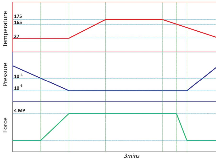
**Figure 6.2: Thermally assisted cold-weld bonding** Detailed bonding procedure including stage temperature, chamber pressure and applied force vs. time.
