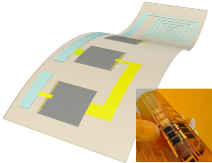
**Fig. 8.2:** The schematic of multifunctional solar cell array in series a spiral RF choke and (inset) image of fabricated GaAs thin-film solar cell array on a 50  $\mu\text{m}$ -thick Kapton® sheet
