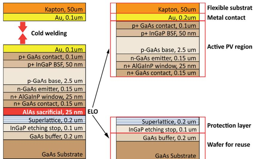
**Fig. 9.2:** Modified protection layer scheme where the top GaAs layer is replaced by a 5 period  $\text{AlGaAs}/\text{GaAs}$  superlattice (SL) that can bend defect propagation toward the wafer edges. AlAs is the sacrificial layer removed during ELO. The active solar cell epitaxial layers are grown on the SL protection layer surface.
