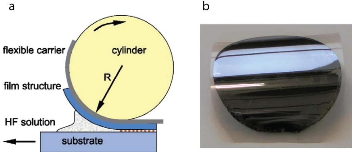
**Fig. 2.8:** Advanced WI-ELO process. (a) Schematic illustration of ELO set-up with a guiding cylinder that applies a stabilized radius of curvature near the etch interface. (b) Photograph of lifted-off 2'' GaAs thin-film on a flexible plastic carrier via WI-ELO process. Reproduced from ref. 26.
