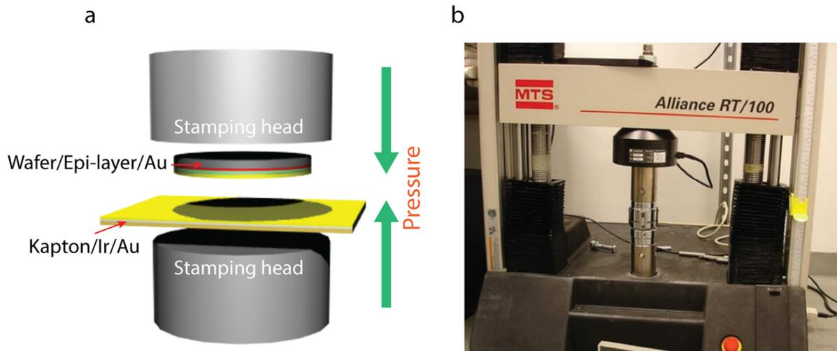
**Fig. 3.1:** Cold-welding process (a) Schematic illustration of cold-welding process to bond the between Au coated wafer and flexible substrate under the ambient condition (b) Photograph of a bonding tool (Alliance RT/100, MTS).
