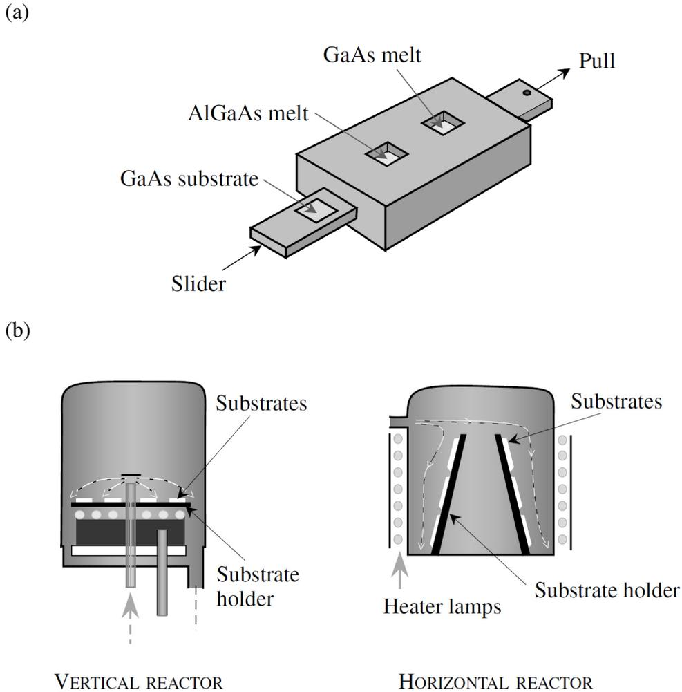
**Fig 1.6:** Schematic of LPE and VPE growths (a) The heterostructure can be grown by contacting the substrate with different melts using slider (LPE). (b) The crystal growth occurs in vertical or horizontal reactor via chemical reaction of the supplied gases with the heated substrate (VPE). Reproduced from reference 3.
