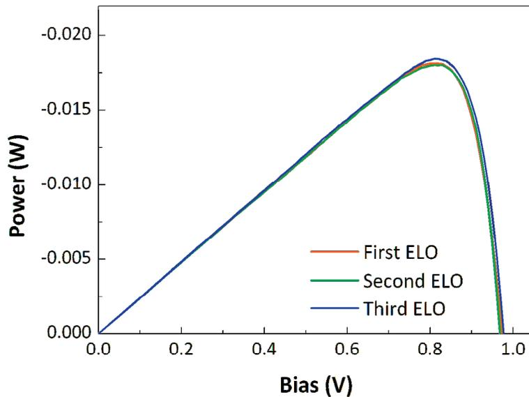
**Figure 6.14. Power generation for photovoltaic cells.** Comparison of the power output from each photovoltaic cell under forward voltage (V) under 1 sun intensity, AM1.5G illumination.
