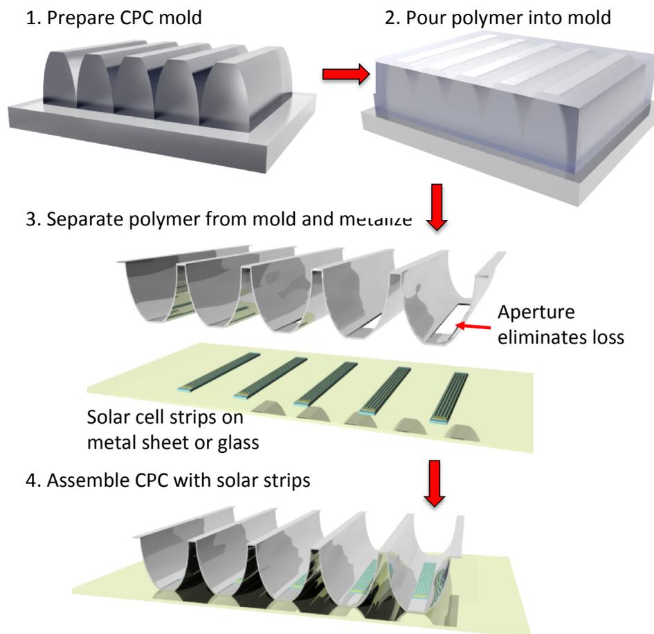
**Fig. 9.4:** One of two methods for fabricating and integrating compound parabolic concentrators (CPC). 1. Prepare a mold, for example by etching the appropriate pattern in glass using photolithographic patterning. 2. Pour polymer into mold to form concentrator shape. 3. Remove concentrator (along with window apertures) and metalize interior surface with Ag. 4. Attach solar cell array to CPC by cold weld bonding forming contact fan out.
