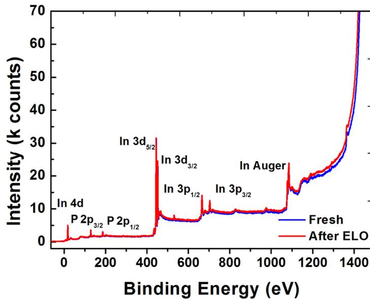
**Fig. 4.4:** X-ray photoelectron spectra from the fresh and the ELO processed substrate surfaces.
