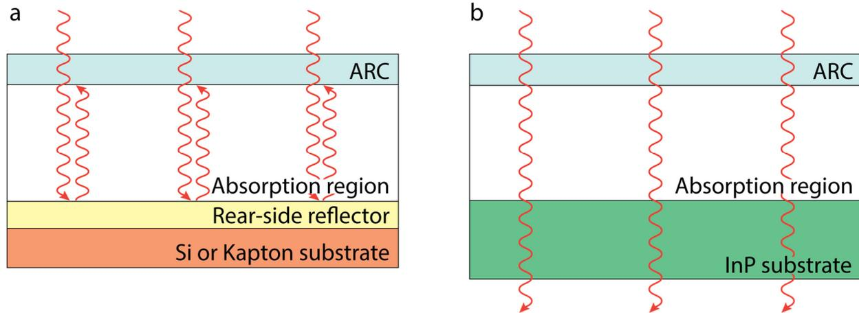
**Fig. 5.3:** Schematic demonstration of light absorption in (a) thin-film devices and (b) substrate devices with and without light trapping mechanism.
