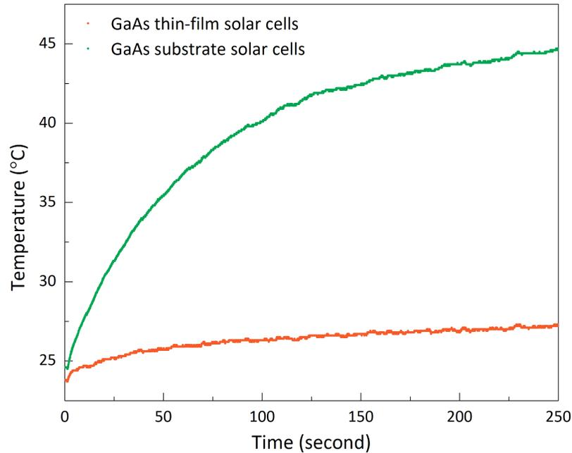
**Fig. 7.9 Operating temperature of thin-film and substrate GaAs solar cells.** Time dependent temperature measured by IR imaging under 1 sun illumination ( $100\text{mW}/\text{cm}^2$ ).
