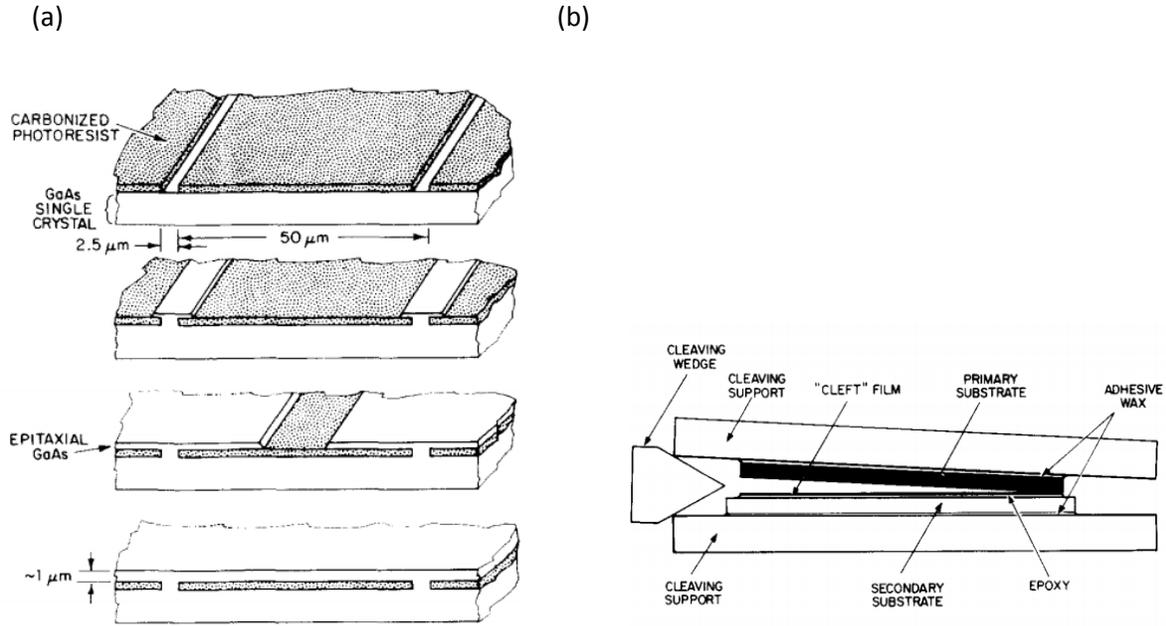
**Fig. 2.35:** Schematic illustration of cleavage of lateral epitaxial films for transfer (CLEFT) process. (a) Fabrication flow for CLEFT process. The photoresist is patterned on a GaAs substrate, then the GaAs layer is grown together laterally from the narrow slot to form a continuous single crystalline film. (b) Cross-sectional view of thin-film transferring process to a host substrate. A small force is applied to cleave the sample. Reproduced from ref. 4.
