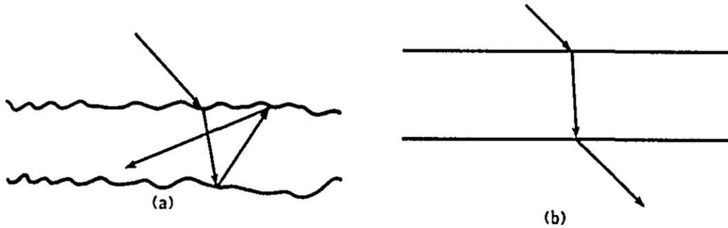
**Fig. 2.13:** The schematic illustration of light absorption in thin-film. (a) The light trapping structure using textured surface. (b) The thin-film without light trapping structure. Reproduced from ref. 9.
