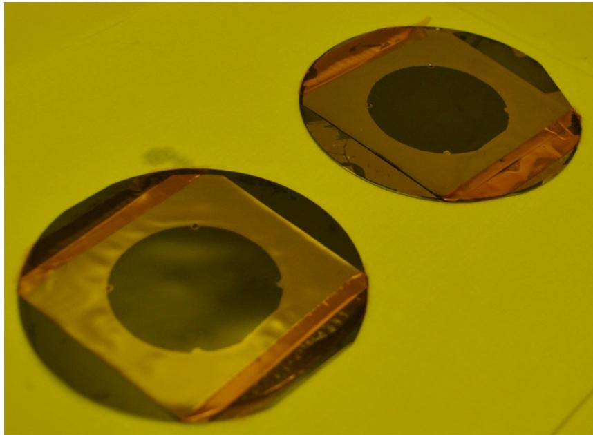
**Fig. 3.2:** ELO processed 2 inch diameter GaAs thin-film after bonded onto plastic substrate via thermally-assisted cold-weld bonding under vacuum. (Lifted-off from fresh wafer (left) and reused-wafer (right))
