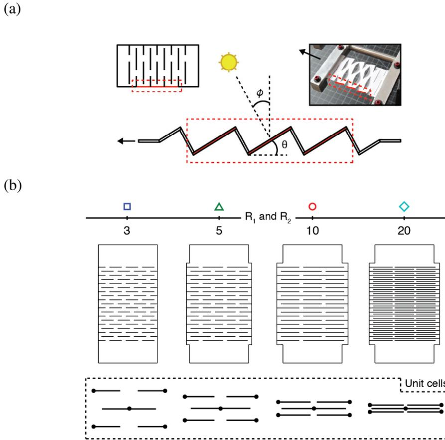
**Fig. 8.5:** (a) A kirigami tracking structure that, upon stretching, simultaneously changes the angle of the elements comprising the sheet. By incorporating thin film solar cells into this structure, it may be used as a low-profile alternative to conventional single-axis solar tracking mechanisms. (b) Schematics of four kirigami structures, where  $R_1 = R_2 = 3, 5, 10,$  and  $20$ , along with their corresponding units cells. Figure courtesy of Aaron Lamoureux
