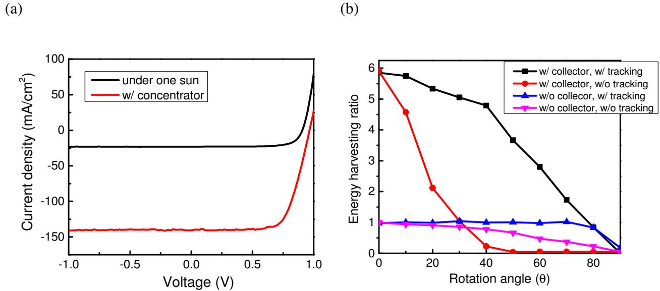
**Fig. 8.8:** Energy harvesting and GaAs solar cell characteristics. (a)  $I$ - $V$  characteristics of GaAs solar cell with and without the Ag-coated origami collector. (b) Comparison of energy harvesting ratio with and without the trackers and collectors. Figure courtesy of Chih-Wei Chien.
