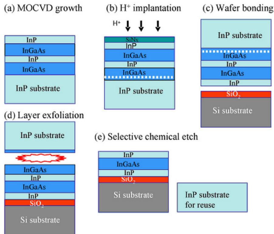
**Fig. 2.34:** Process flow chart for InP layer transfer via exfoliation process. (a) Heterostructure growth using MOCVD (b) Hydrogen ion implantation process (c) Wafer bonding process (d) Exfoliation process induced by thermal annealing (e) Selective chemical etching process of both samples. Reproduced from ref. 79.
