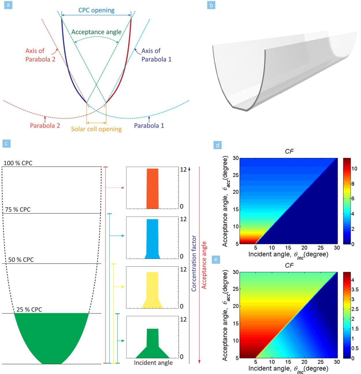
**Fig. 7.5 Two dimensional mini-compound parabolic concentrator (CPC) design.** Schematic illustration of the (a) CPC shape and (b) 2 dimensional CPCs. (c) Effect of CPC truncation on the acceptance angle and concentration factor. Contour plot of light incident angle dependent concentration factors for various shapes of (d) non-truncated, and (e) truncated CPCs.
