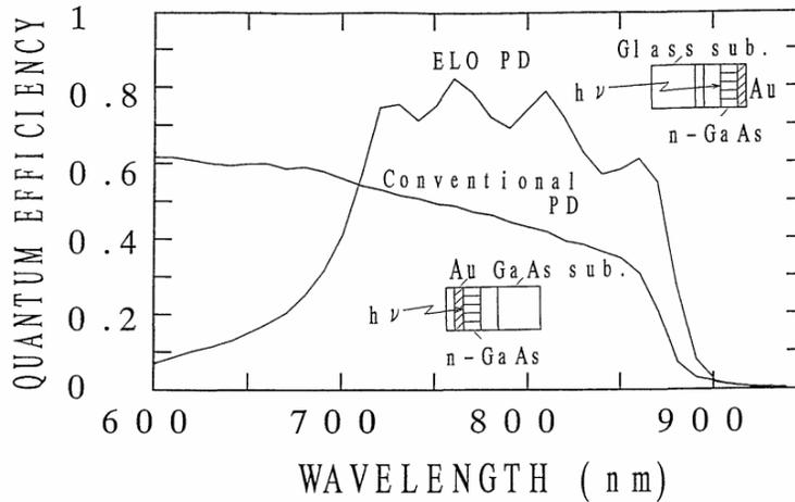
**Fig. 2.24:** Comparison of spectral response between substrate-based and ELO processed photodiode. Insets show a schematic of both device structure. Reproduced from ref. 58.
