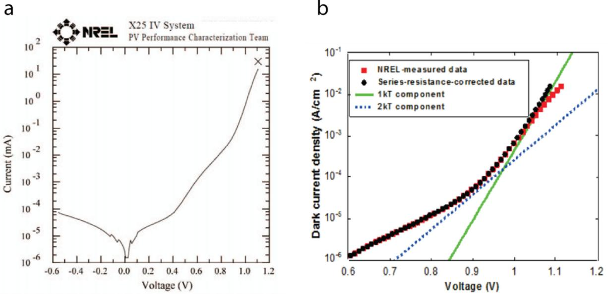
**Fig. 2.18:** Dark current density of Alta Devices' thin-film GaAs solar cells (a) measured by NREL and (b) fitted by double diode model. Reproduced from ref. 15.
