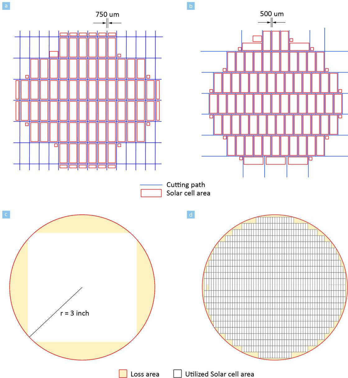
**Fig. 7.2 Laser dicing of thin-film GaAs solar cells on plastic sheet** (a) Linear cutting pattern with 750 μm spacings between solar cells. (b) Zig-zag cutting pattern with 500 μm spacing between solar cells. Schematic illustration of wafer utilization for (c) single square cut and (d) multiple small bar shape (2.5 mm × 6.5 mm) cut.
