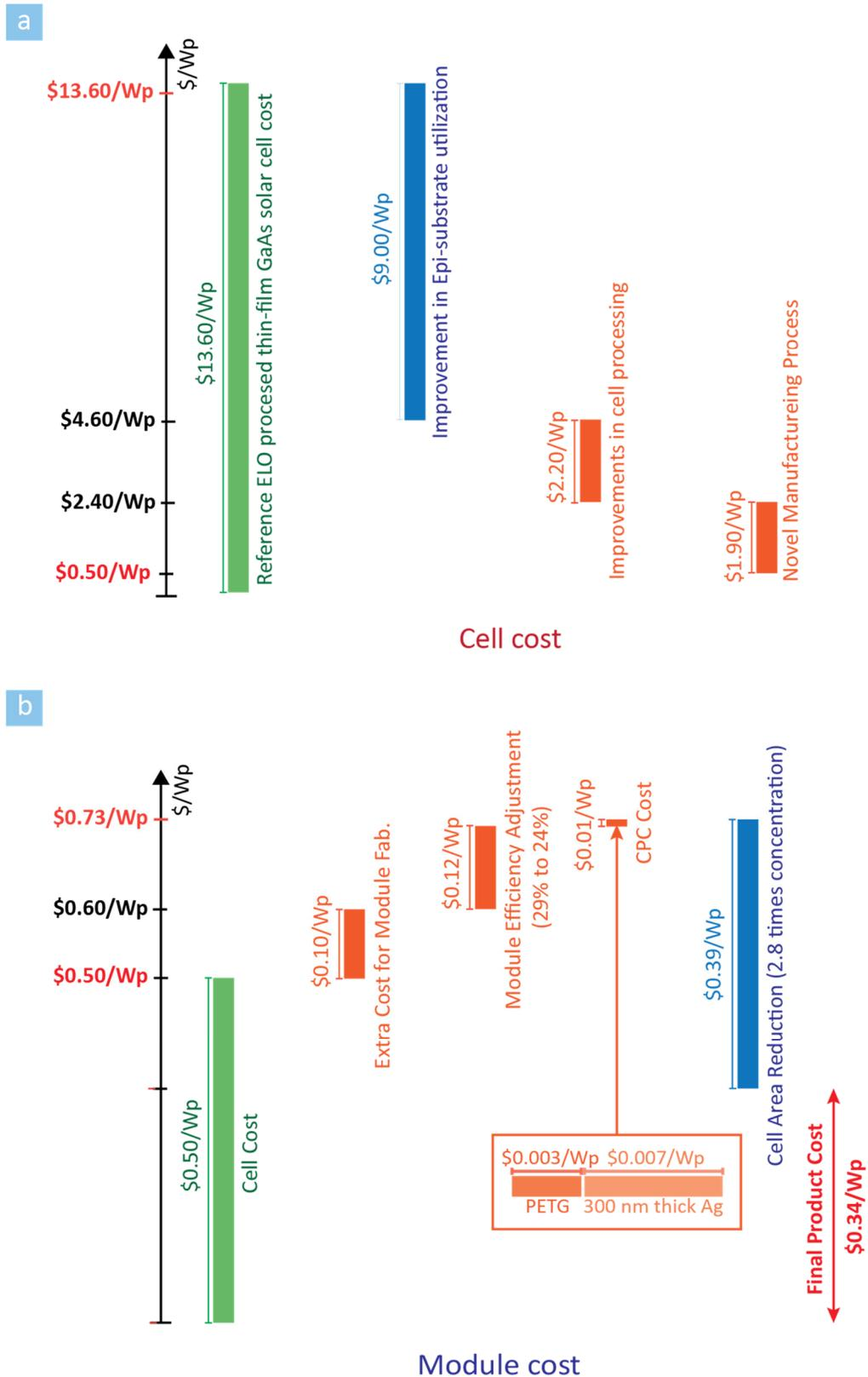
**Fig. 7.17 Production cost estimation** (a) Cost estimation for thin-film GaAs solar cells and (b) modules where the cells are integrated with plastic mini-CPCs.
