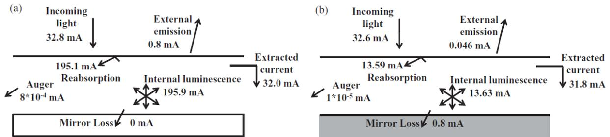
**Fig. 2.17:** Diagram of current at the operating point of photovoltaic cell (a) with a perfect mirror and (b) with an absorbing substrate. Both cells provide a comparable current, however, the significant incensement of internal luminescence via perfect mirror results in the improved  $V_{oc}$ . Reproduced from ref. 11.
