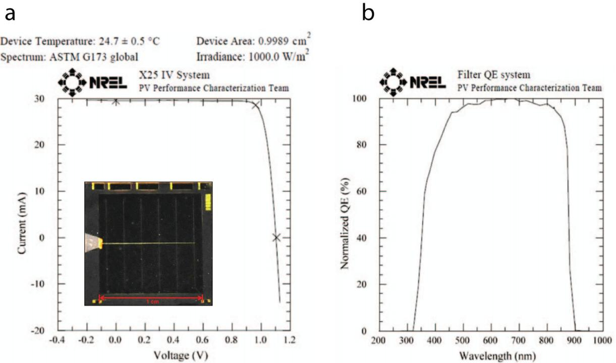
**Fig. 2.21:** Characteristic of Alta Devices' GaAs thin film solar cell certified by NREL (a) *J-V* characteristic under simulated AM1.5G 1 sun illumination. Inset: Photograph of device. (b) EQE of solar cell. Reproduced from ref. 15.
