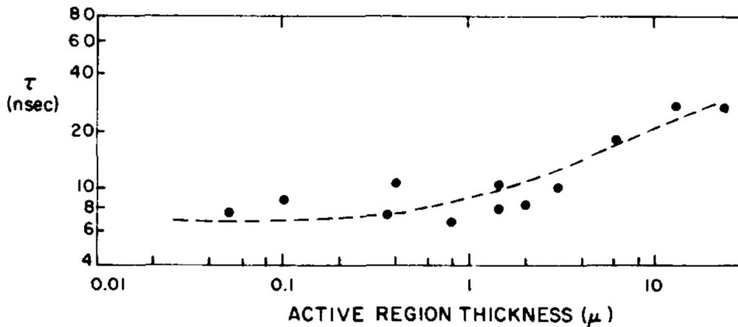
**Fig. 2.14:** Recombination lifetime vs. active layer thickness. The dots represents experimental data, and the dashed curve is the theoretical values. Reproduced from ref. 10.
