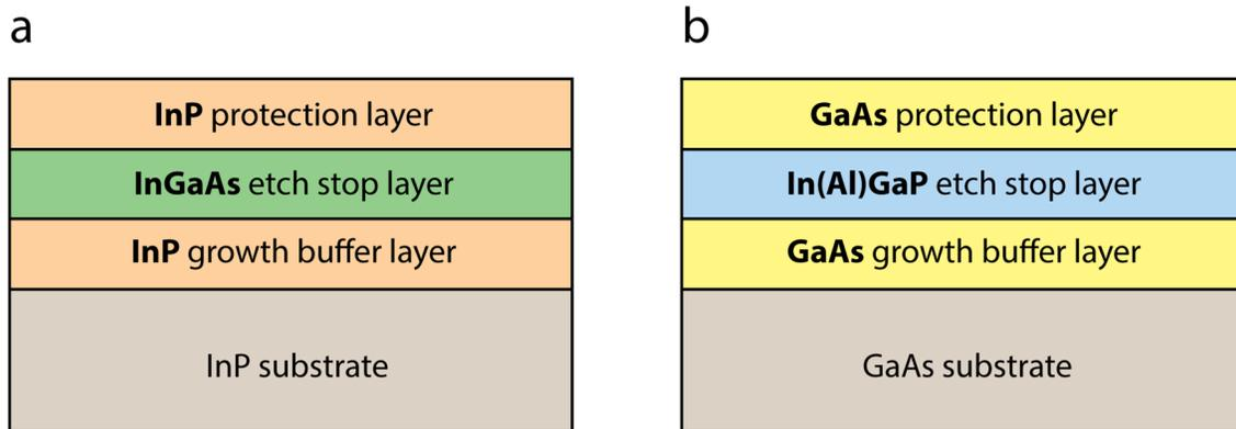
**Fig. 3.4:** Epitaxial protection layers schemes. (a) InGaAs/InP and (b) In(Al)GaP/GaAs protection layers employed for non-destructive ELO process to preserve the InP and GaAs wafer surface quality, respectively, from the dilute HF.
