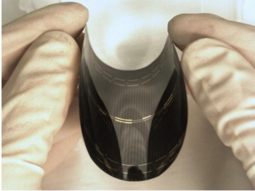
**Fig. 2.22:** Picture of ELO processed InGaP/GaAs double junction photovoltaic cells from 4 inch substrate. Reproduced from ref. 52.
