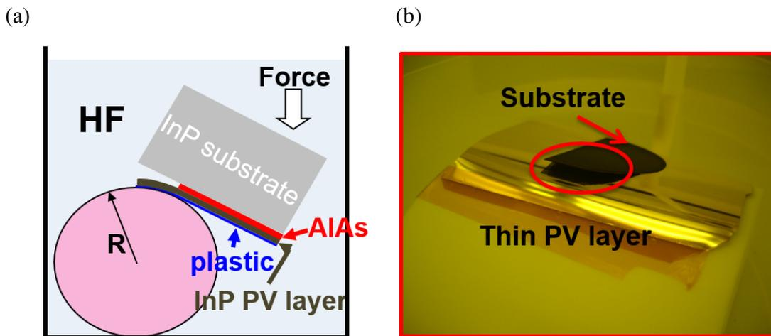
**Fig. 4.2:** (a) Schematic of weight-induced ELO set-up (b) Image of ELO process for half 2-inch-diameter epitaxial layer.
