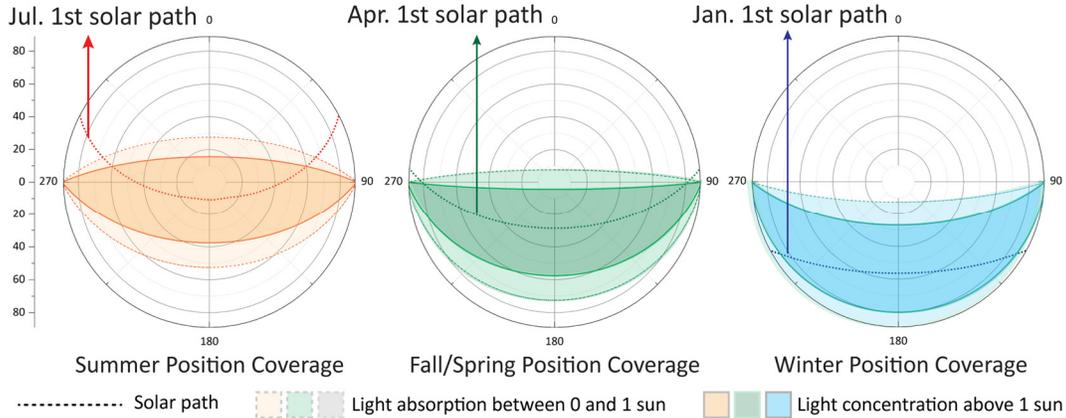
**Fig. 7.12: Optimum alignment of CPCs for maximum annual energy harvesting.** Polar plots showing coverage of CPC at its optimum seasonal positions.
