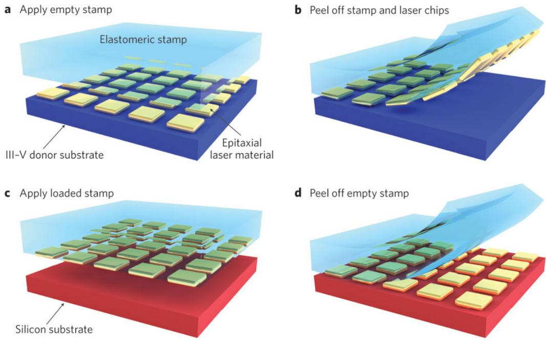
**Fig. 2.12:** Schematic illustration of transfer printing process.<sup>35</sup> The elastomeric stamp is used to pick up the lifted-off thin-film layers and transfer them to the host substrate. Reproduced from ref. 32.
