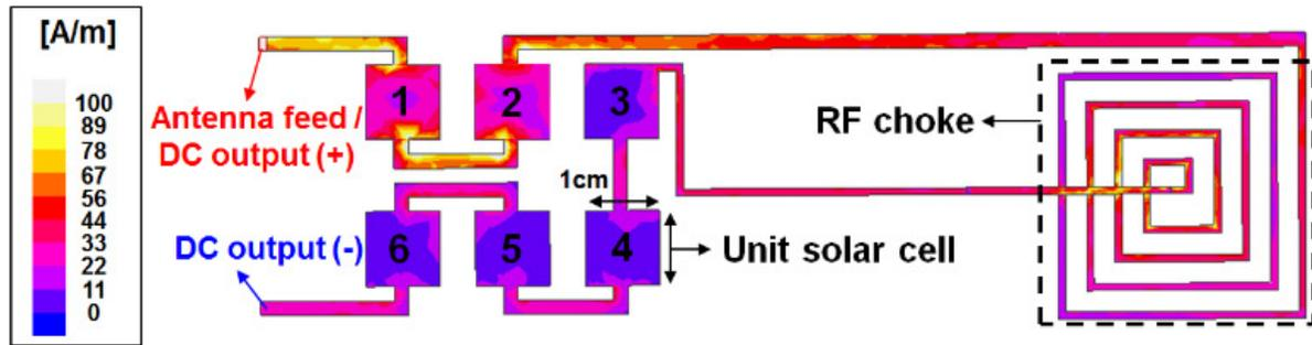
**Fig. 8.3:** Thin-film solar cells working as part of a UHF antenna, their current distribution at 350 MHz and the whole antenna topology integrated with a RF choke.
