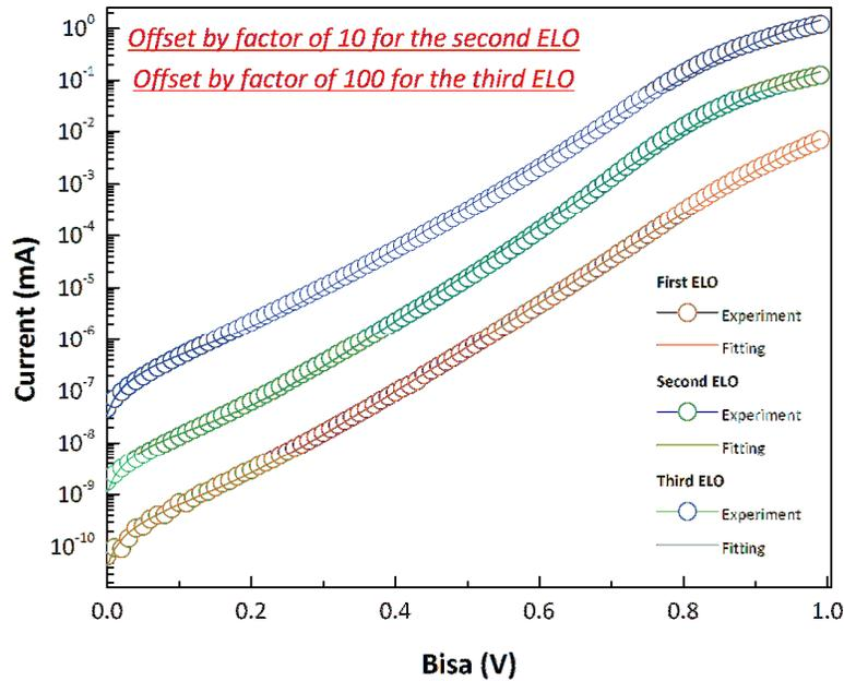
**Figure 6.13.** Current density-voltage ( $J$ - $V$ ) characteristics of photovoltaic cells in the dark. Measured and fitted  $J$ - $V$  characteristic of the first, second and third ND-ELO processed solar cells. The second ELO is offset by a factor of ten and the third ELO by a factor of hundred for clarity.
