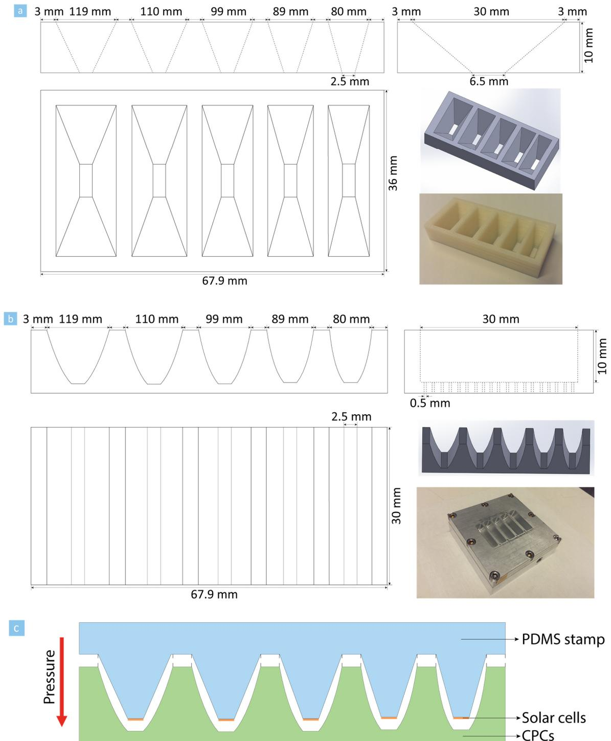
**Fig. 7.3 Self-aligned transfer printing process** (a) Mold design for the PDMS stamp. Image shows a 3D printed mold. (b) Mold design for the plastic CPCs. Image shows a mold made from a metal block. (c) Schematic illustration of the fit between the PDMS stamp and the plastic CPCs for solar cell transfer printing.
