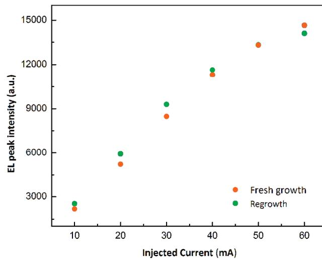
**Figure 6.16. Comparison of LEDs performance.** Comparison of peak intensity vs applied current density extracted from LED electroluminescence characteristics.
