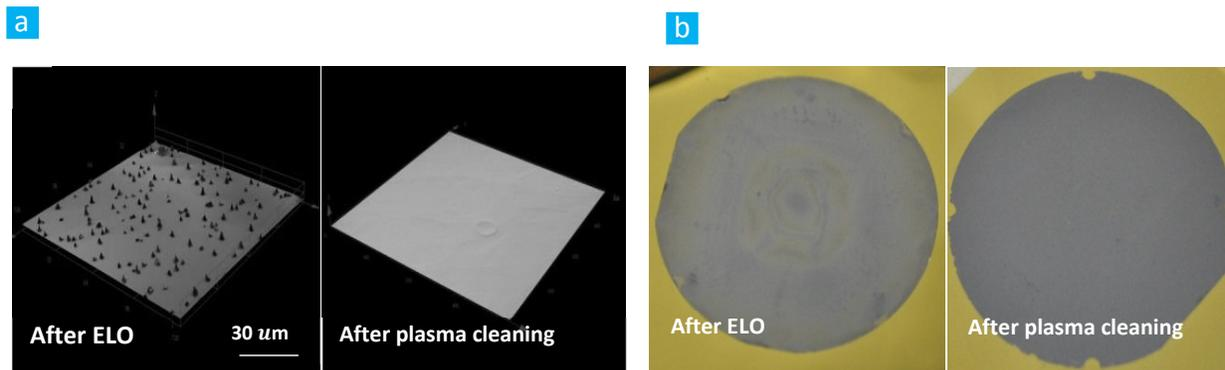
**Figure 6.5:** Comparison of wafer surface morphology before and after ELO. (a) Three dimensional laser microscope image of the surface immediately following ELO (left), and after plasma cleaning (right). (b) The thin-film surface following ELO (left), and after plasma cleaning (right).
