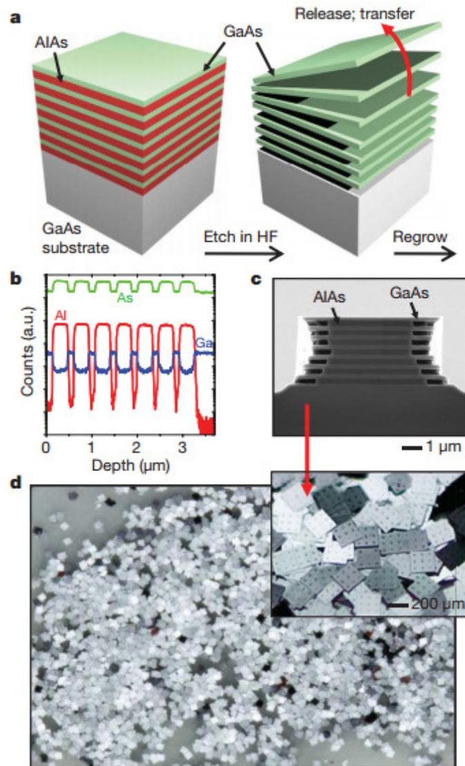
**Fig. 2.36:** The multiple layer release process. (a) Schematic of epi-layer structure and fabrication flow for the multiple layer release process. (b) SIMS profile and (c) SEM image of epitaxial structure. (d) Photograph of a collection of GaAs solar cells produced by a multiple layer release process. Reproduced from ref. 8.
