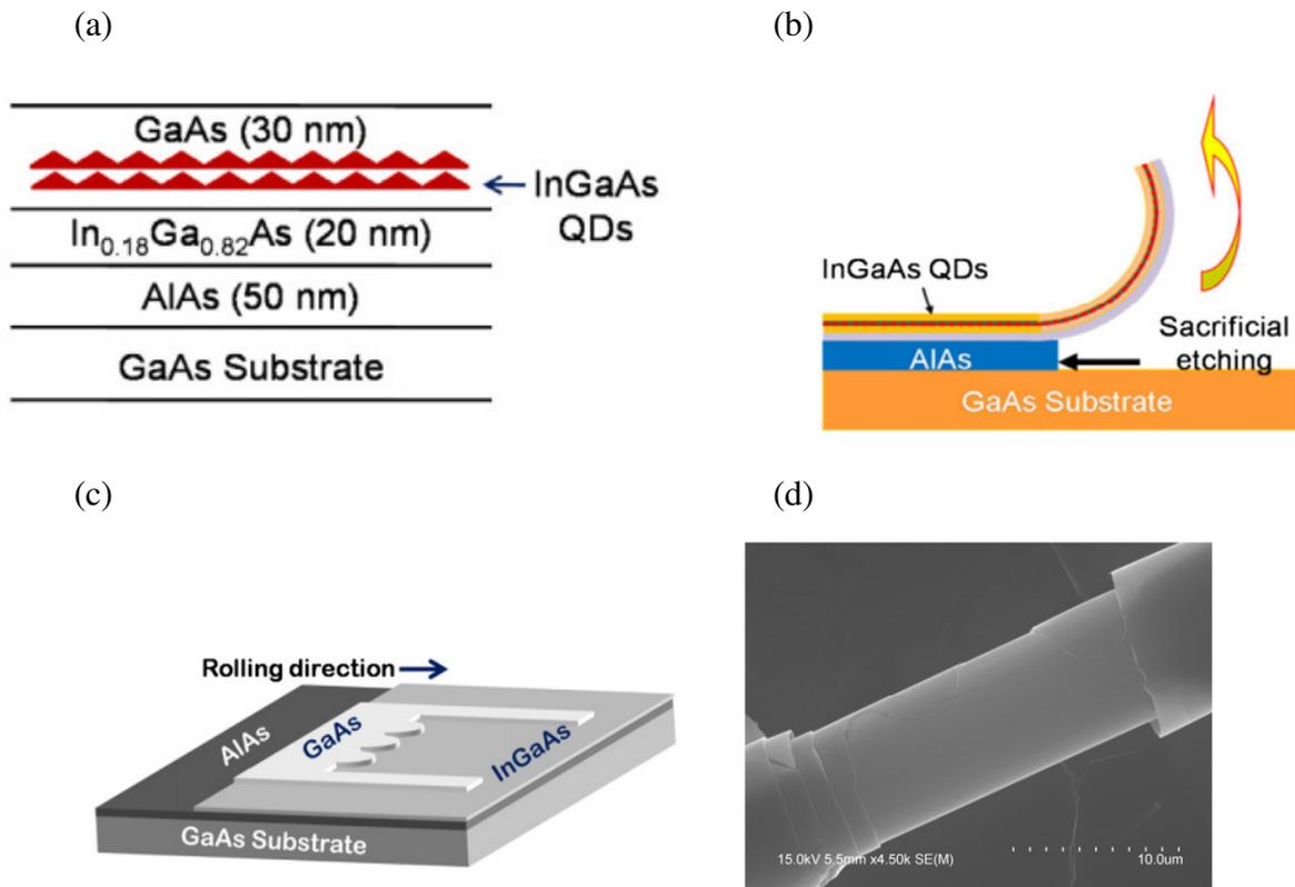
**Fig. 2.27:** Schematic and image of lift-off process of rolled-up quantum dot microtube. (a) The growth structure of InGaAs/GaAs quantum dot heterostructure for lift-off process. (b) Schematic illustration of fabrication process for microtube ring resonators. (c) The schematic of an etched U-shaped mesa (d) Scanning electron microscopy image of lifted-off rolled up microtube. Reproduced from ref. 63.
