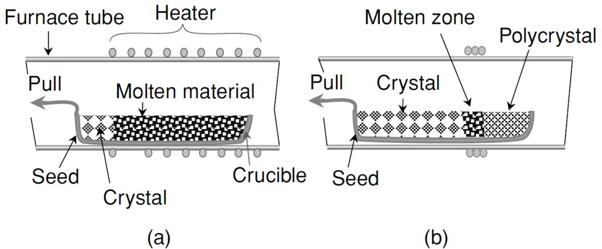
**Fig 1.5:** Schematic of horizontal bridgeman and gradient-freeze growths. Crystal growth by slowly lowering the boat temperature from the end with the seed by (a) moving the hot zone of furnace along the tube (horizontal bridgeman growth) or (b) slowly pulling out the boat (gradient-freeze growth). Reproduced from reference 3.
