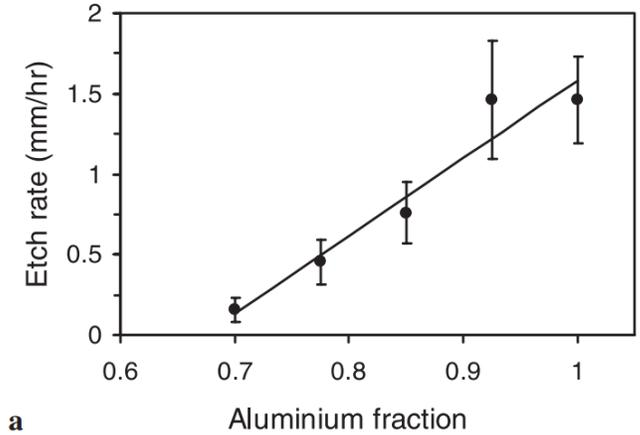
**Fig. 2.6:** Lateral etch rate depending on the Al composition of AlGaAs sacrificial layer. Reproduced from ref. 20.
