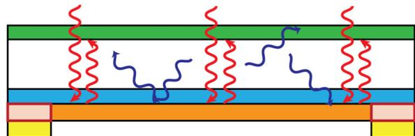
**Fig. 9.5:** Comparison of absorption processes between conventional substrate/thin film solar cells and bi-facial GaAs solar cells with rear NIR reflecting distributed Bragg reflecting mirrors. High reflectance of the DBR and minimum absorption losses by the patterned back ohmic contact layer enhance the photon recycling.
