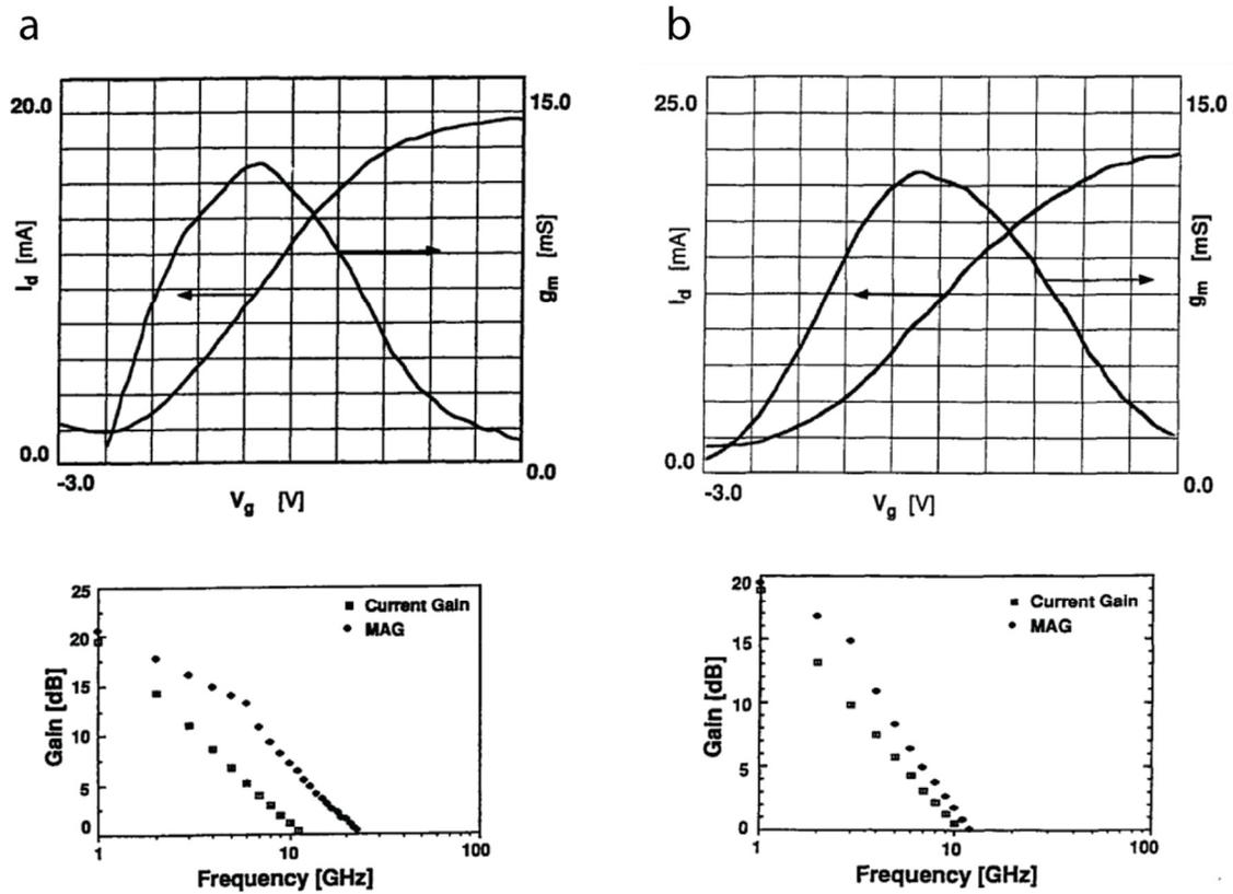
**Fig. 2.28:** Characteristic of GaAs HEMTs. DC transfer (top) and RF characteristic of (a) an on wafer GaAs HEMTs and (b) an ELO processed GaAs HEMTs. The HEMTs on wafer shows an  $f_t = 11.5$  GHz and  $f_{max} = 23$  GHz, and ELO processed HEMT shows an  $f_t = 10.5$  GHz and  $f_{max} = 12$  GHz. Reproduced from ref. 64.
