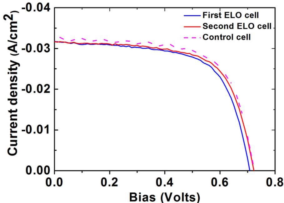
**Fig. 4.7:** Current density versus voltage characteristics of the first and the second ELO processed ITO/InP and the control solar cells bonded to a Kapton® sheet, all measured under 1 sun, AM1.5G simulated solar illumination.
