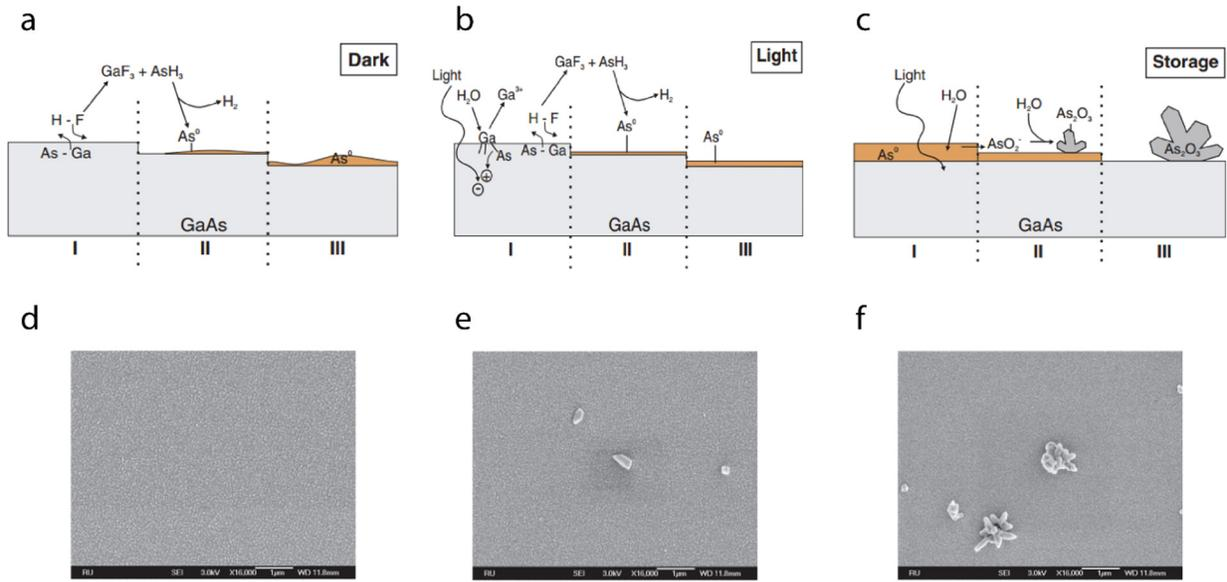
**Fig. 2.31:** Reaction of GaAs in HF etchant under dark and illumination condition. Schematic overview of reaction process on GaAs surface (a) during exposed to HF under dark condition, (b) under illumination and (c) during storage in ambient environment. SEM images of etched GaAs surface by HF (d) immediately after the etching, (e) after storage of sample for 3 hours and (f) for 4 weeks. Reproduced from ref. 22.
