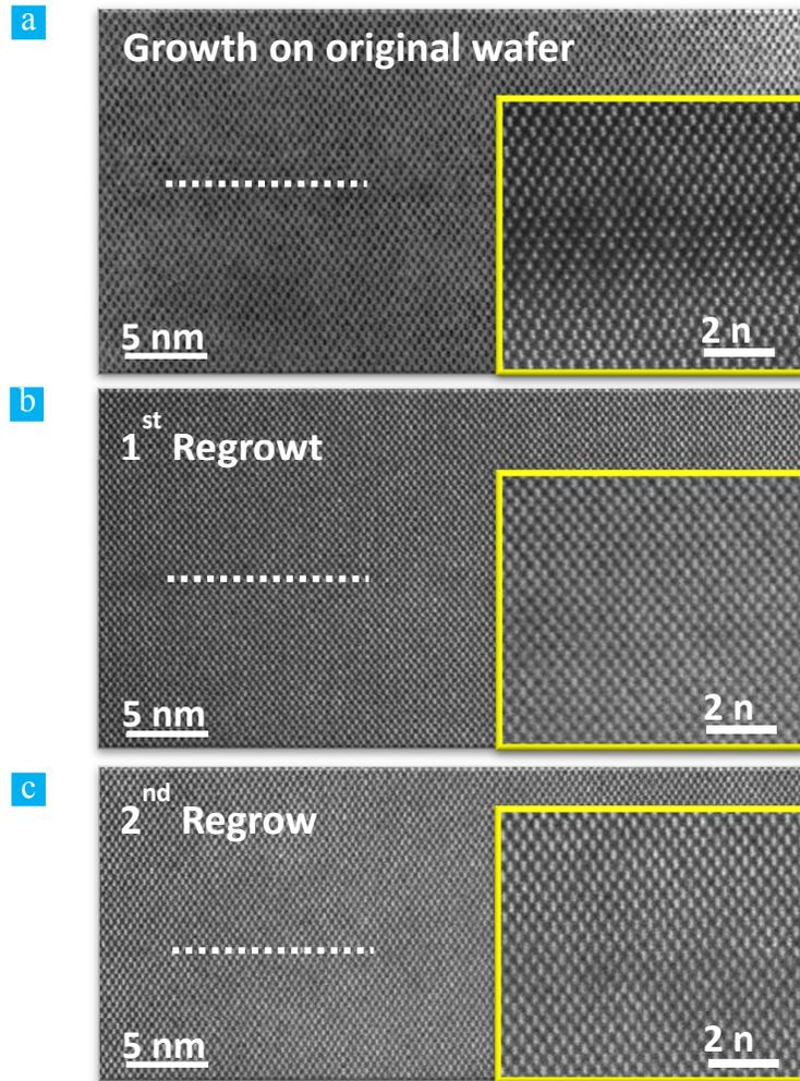
**Figure 6.9:** Atomic resolution cross-sectional transmission electron microscope images of the growth interface between the wafer and epitaxial GaAs layer grown on (a) original, (b) first epitaxial and (c) second epitaxial growth steps. Dotted lines indicate the starting growth interfaces. Insets show details of the growth interfaces.
