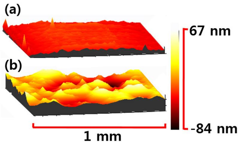
**Fig. 4.6:** Surface morphology of the original substrate (a) after ELO and protection layer removal and (b) after the ELO without the protection layer.
