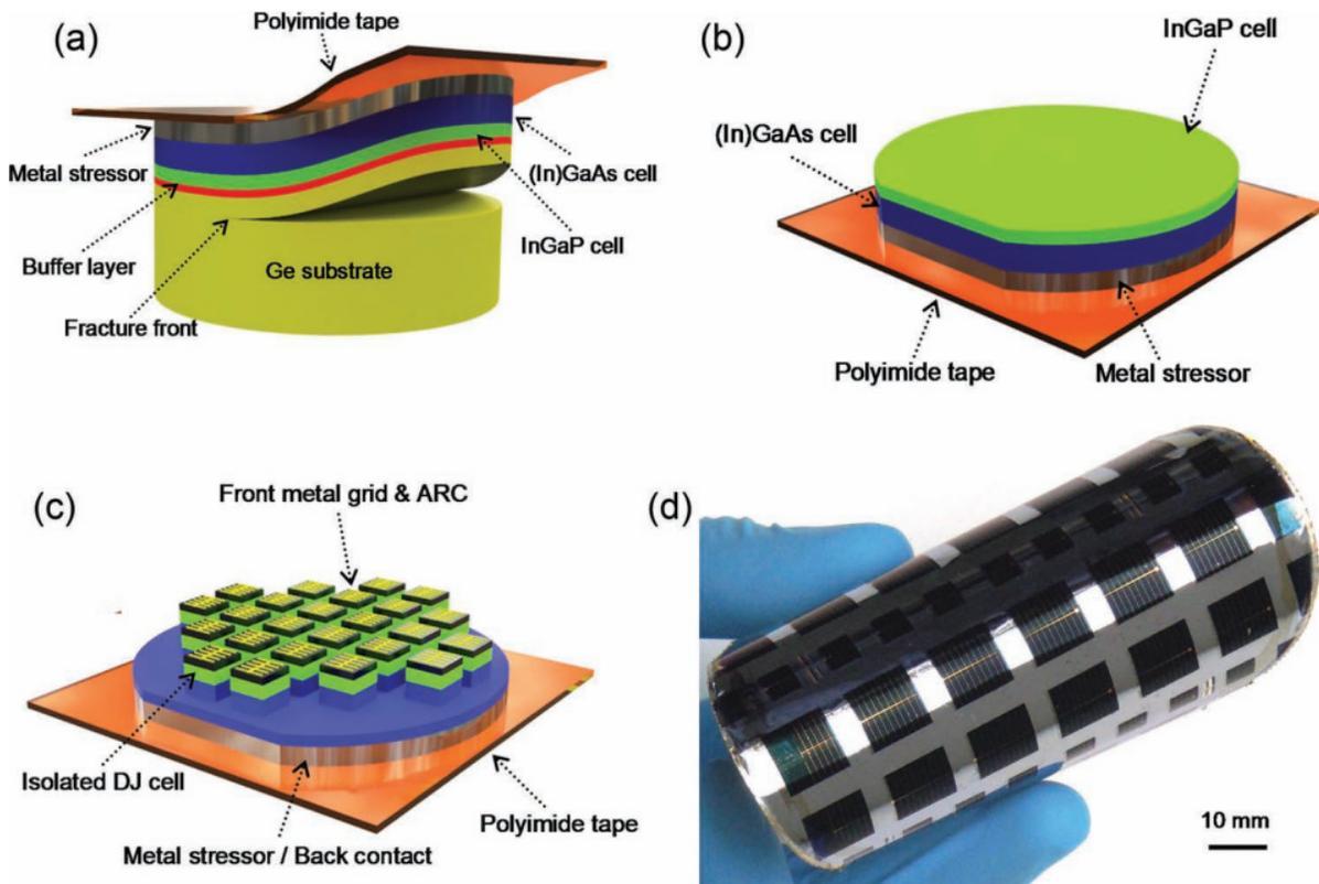
**Fig. 2.33:** Illustration of controlled spalling process and image of fabricated thin-film solar cells. (a) The schematic of structure used in controlled spalling process. (b) Schematic of lifted-off thin-film active layers bonded on polyimide tape. (c) Schematic of fabricated thin-film solar cells on flexible substrate. (d) Photograph of fabricated thin-film tandem solar cells on plastic substrate. Reproduced from ref. 78.
