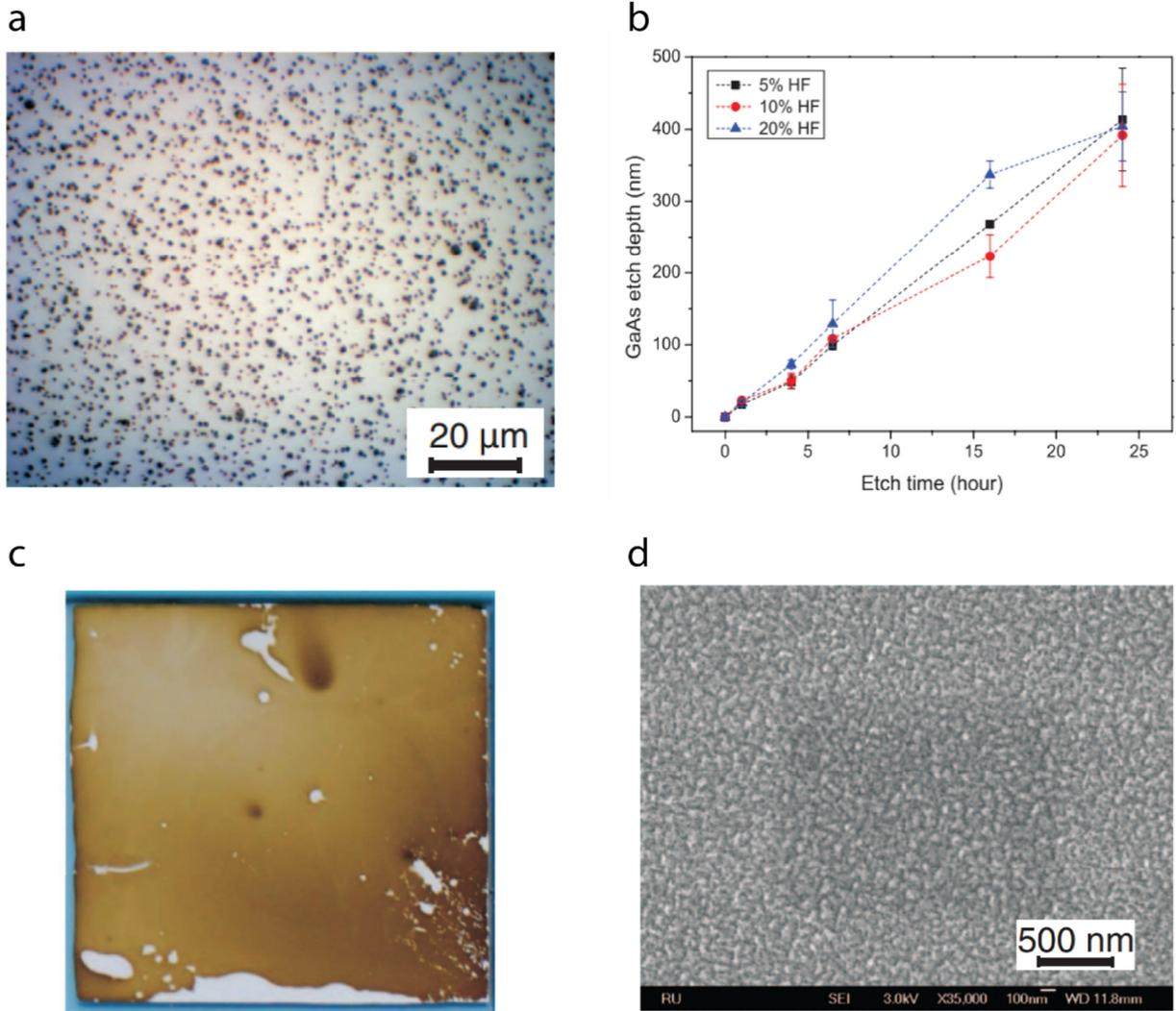
**Fig. 2.30:** Reaction of GaAs in HF etchant (a) Optical microscope image of GaAs surface after exposed to HF, and stored in ambient air. (b) Etch rate of GaAs in dilute HF etchant. (c) Optical microscope image of GaAs surface after exposed to HF while it is kept in dark during etching. (d) SEM image of the brown haze in fig. 2.15(b). Reproduced from ref. 22.
