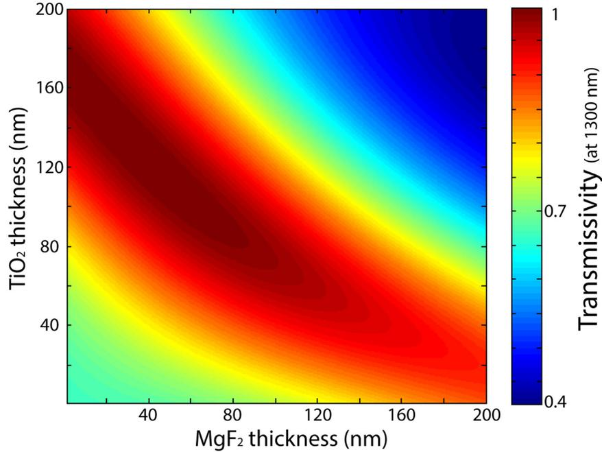
**Fig. 5.6:** Simulated transmission contour plot of 1300 nm light in-coupled into the photodiode by employing MgF<sub>2</sub> and TiO<sub>2</sub> bi-layer ARC structure with different layer thicknesses. 100% transmission is achieved when 40 nm thick MgF<sub>2</sub> followed by 123 nm thick TiO<sub>2</sub> are employed. 37 nm thick MgF<sub>2</sub> followed by 127 nm thick TiO<sub>2</sub> are measured on actual devices, providing a theoretical value of 99.996% light transmission.
