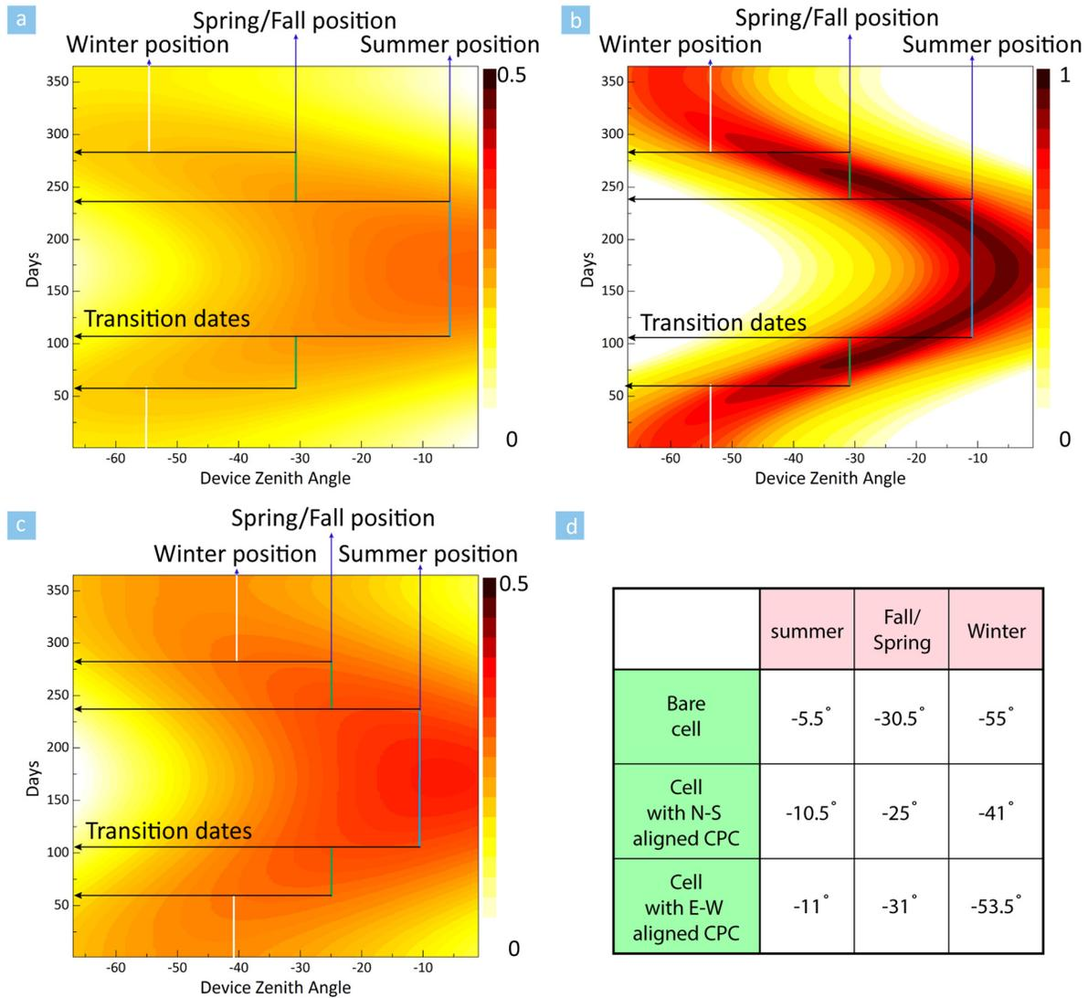
**Fig. 7.11 Optimum alignment of CPCs.** Contour plot of energy harvesting for each day, depending on the CPC tilt angle of (a) non-concentrated cell, (b) east-west axis and (c) north-south aligned CPC. Solid lines indicate optimum seasonal CPC positions and transition dates for maximum yearly energy harvesting. (d) Summary of optimum seasonal facing angles for each case.
