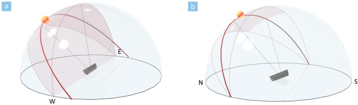
**Fig. 7.10 Alignment of CPCs.** Schematic of the CPC longitudinal axis aligned along an (a) east-west axis and (b) north-south axis.
