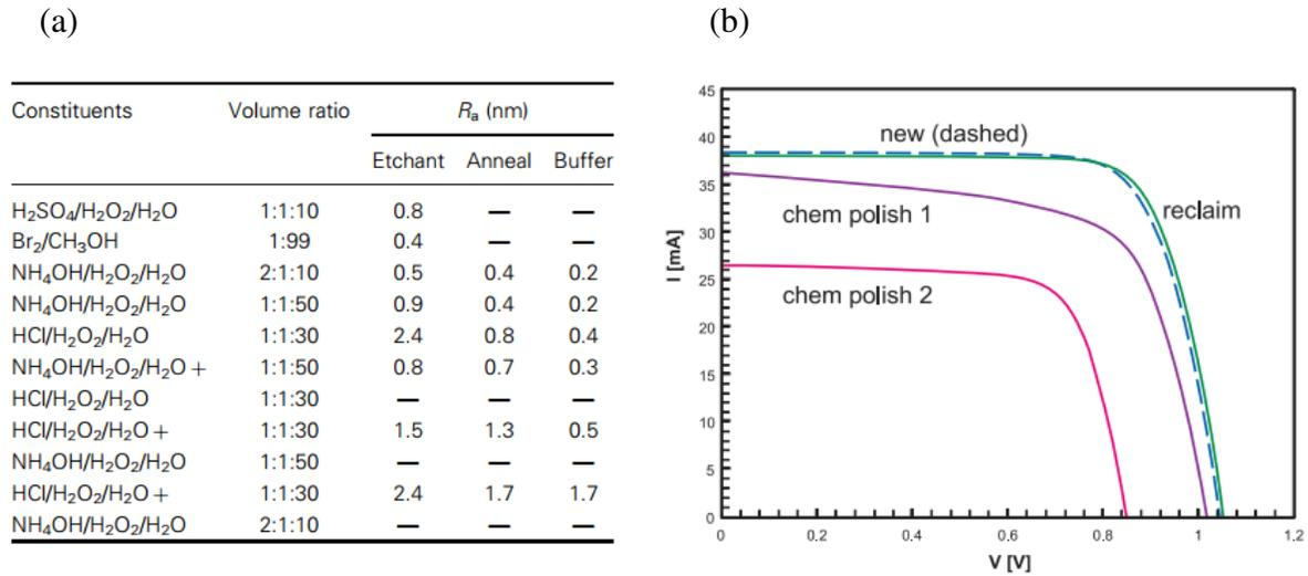
**Fig. 2.32:** Parent substrate recycling after ELO process (a) Test of various etchants for chemical polishing of an ELO processed GaAs wafer surface. (b) Comparisons of  $IV$ -characteristics between thin-film GaAs solar cells grown on fresh, chemical polished and chemo-mechanical polished substrate. Reproduced from ref. 17.
