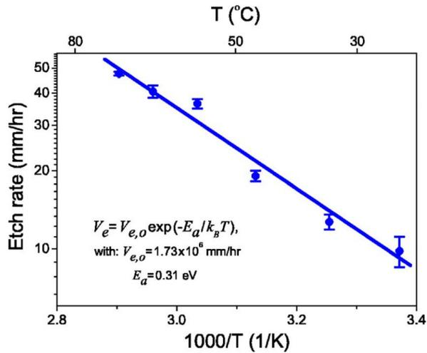
**Fig. 2.7:** Lateral etch rate depending on the process temperature. Reproduced from ref. 24.
