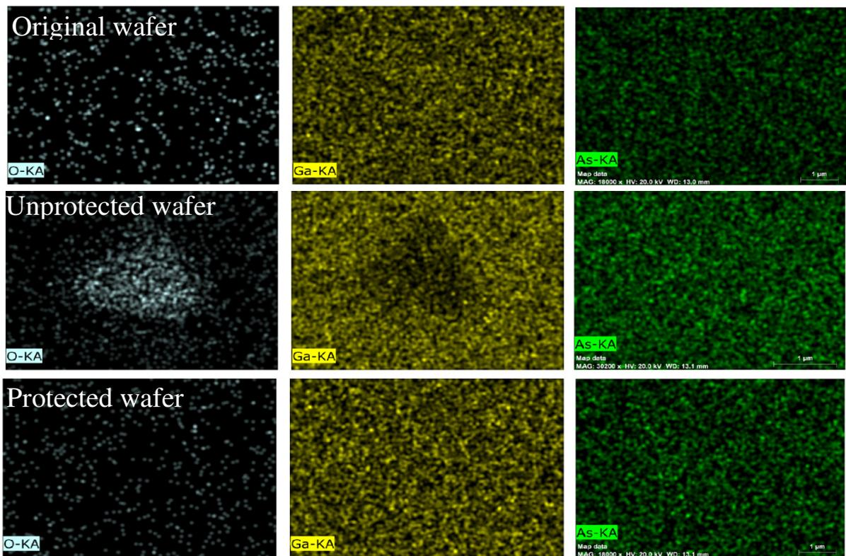
**Figure 6.6:** Hybrid mapping of elemental oxygen, gallium, arsenic near the surface of original, surface protected, and unprotected wafers after the protection layers were removed. The elemental compositions are shown in each image.
