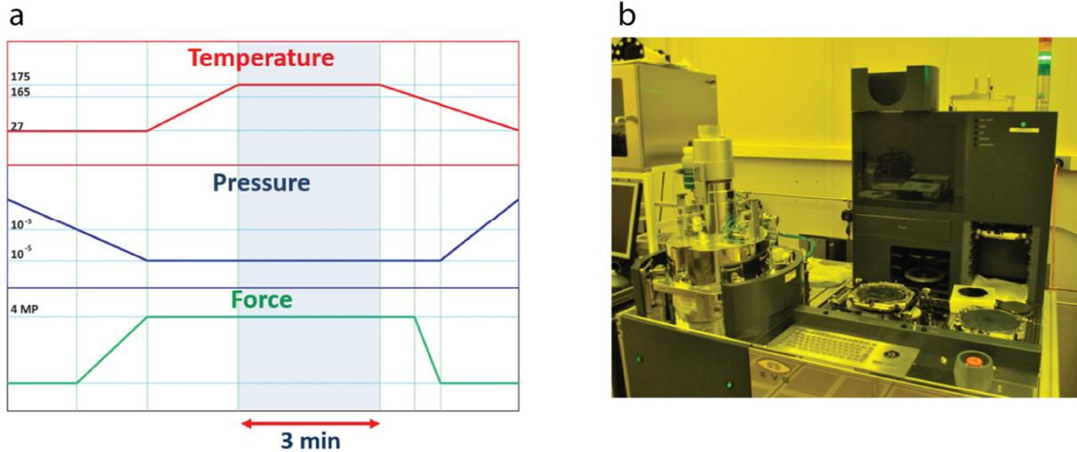
**Fig. 3.3:** Thermally-assisted cold-welding process (a) Detailed bonding procedure including stage temperature, chamber pressure and applied force vs. time. (b) Photograph of bonding tool (EAG 520) used in this work.
