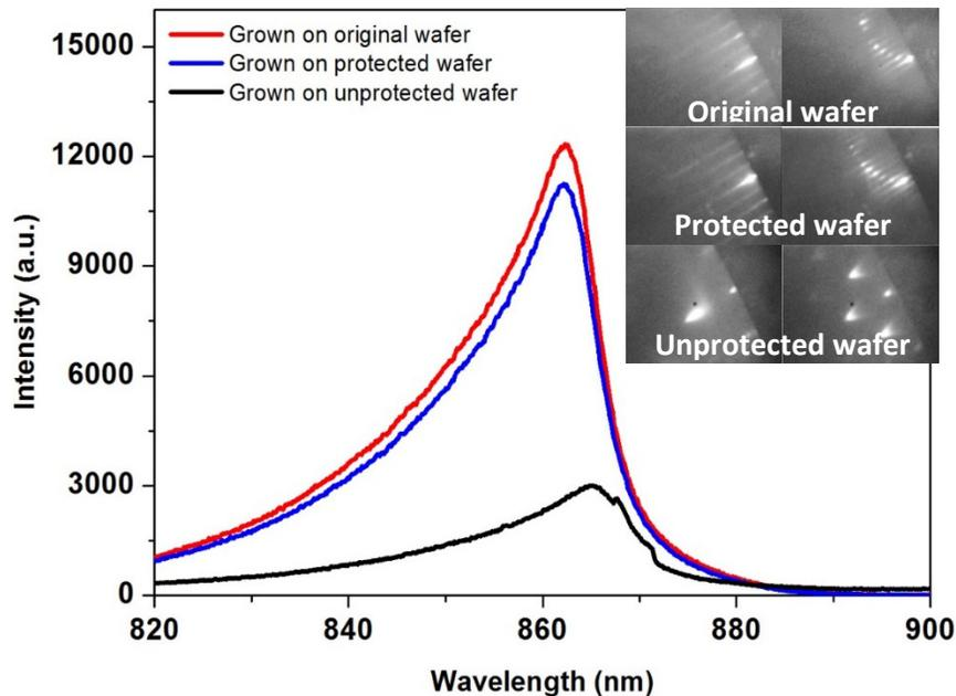
**Figure 6.10:** Photoluminescence spectra at room temperature (300K) from an  $\text{Al}_{0.7}\text{Ga}_{0.3}\text{As}/\text{GaAs}/\text{Al}_{0.7}\text{Ga}_{0.3}\text{As}$  heterostructure on original and reused wafer. Insets: The  $2\times$  and  $4\times$  surface reconstruction patterns obtained by reflection high-energy electron diffraction for the original and etched substrate surfaces with and without a protection layers.
