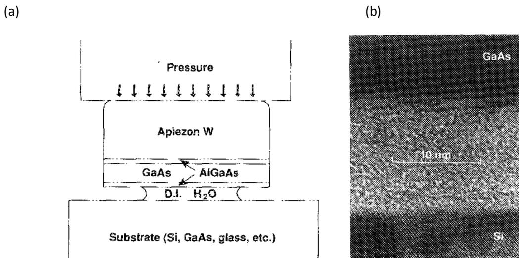
**Fig. 2.11:** Van der Waals bonding process. (a) Schematic illustration of van der Waals bonding of ELO processed film to the arbitrary substrate. (b) Cross-sectional transmission electron microscope image of bonded interface. Reproduced from ref. 13.
