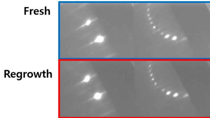
**Fig. 4.5:** The 2x and 4x surface reconstruction patterns obtained by reflection high-energy electron diffraction for the fresh and the ELO-processed substrate after eliminating oxide layer.
