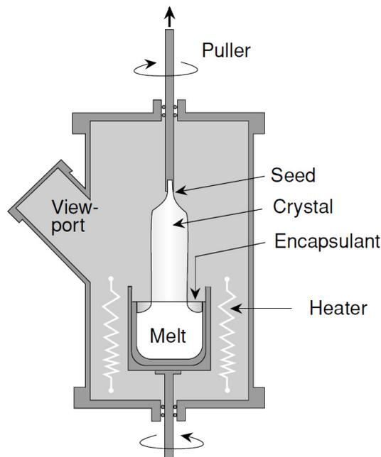
**Fig 1.4:** Schematic of Czochralski process. Ingots of crystalline semiconductor, such as Si, GaAs and InP are grown using the Czochralski process. Reproduced from reference 3.
