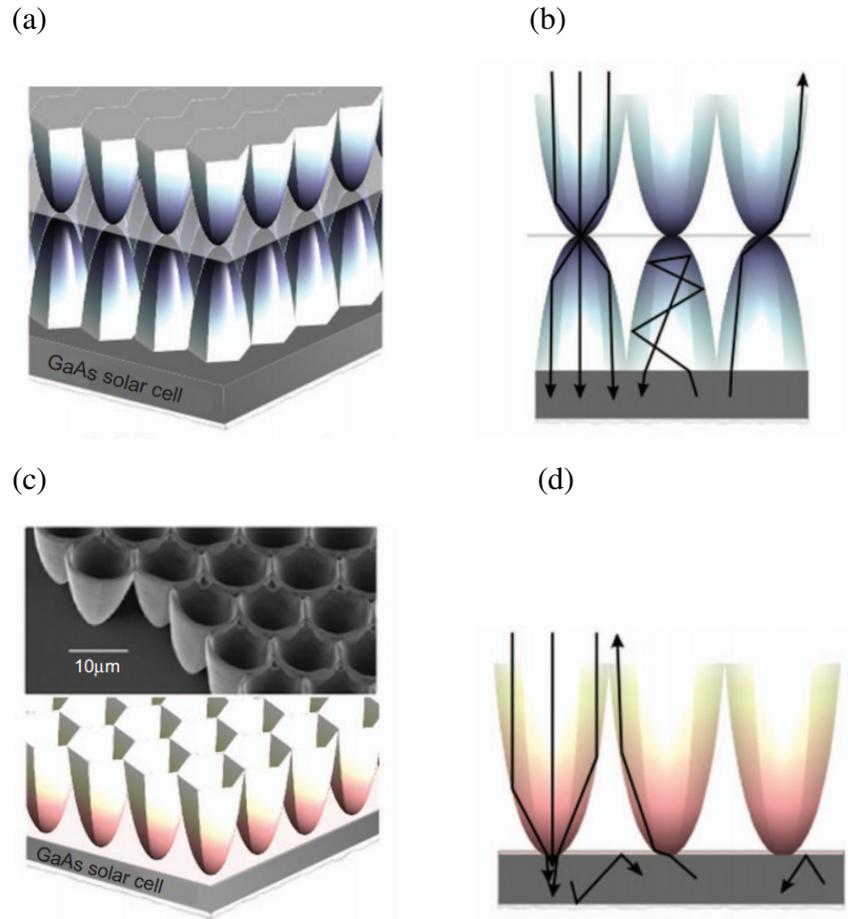
**Fig. 2.19:** Schematic illustration for a coupler structure enhancing photon recycling (a) Dielectric coupler consists of a double array of cone-like structures. The cone-like structures have a light trapping, randomizing back reflector. (b) Illustration of rays in a dielectric coupler structure in fig 2.19(a). (c) Schematic of a metal array coupler combined with GaAs solar cells. (d) Illustration of rays in metal array coupler structure in fig 2.19(c). Reproduced from ref. 47.
