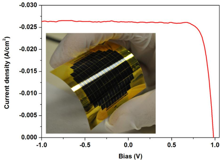
**Fig. 8.1:** The current density-voltage characteristics and (inset) image of flexible GaAs thin-film solar cells on a  $50 \mu\text{m}$ -thick Kapton® sheet
