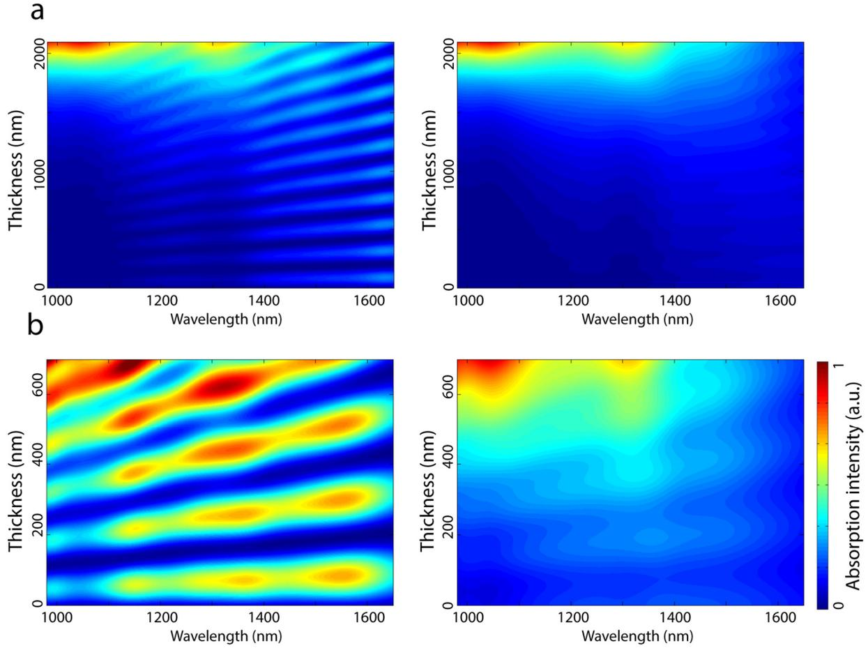
**Fig. 5.4:** (a) The simulated absorption intensity distribution within a thin-film device (L), compared with that within a substrate device (R). The InGaAs absorption layer thickness is 2.1  $\mu\text{m}$ . (b) The simulated absorption intensity distributions for an absorption layer thickness of 0.7  $\mu\text{m}$ . The bi-layer ARC of  $\text{MgF}_2$  (37 nm) and  $\text{TiO}_2$  (127 nm) is employed for all simulated structures.
