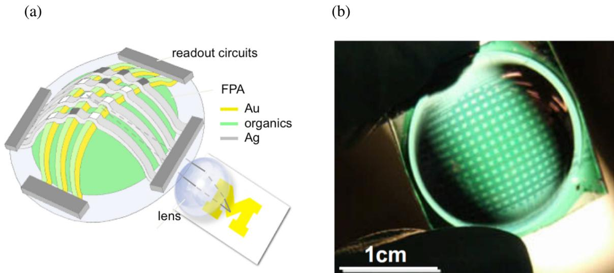
**Fig. 9.1:** The hemispherical focal plane array (HFPA) imaging systems (a) conceptual diagram of a HFPA. (b) an example 20x20 HFPA.
