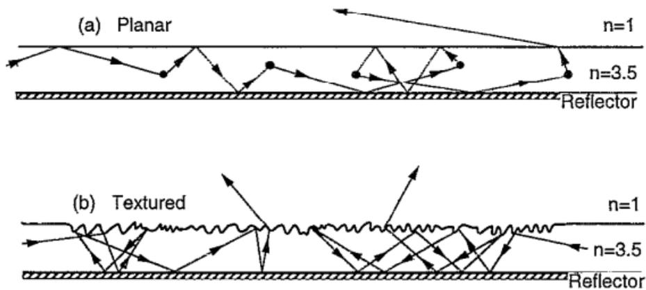
**Fig. 2.25:** The illustration of rays in thin-film light emitting structures (a) with planar surface and (b) with textured surface. The EQE is enhanced in thin-film structures with rear-side reflectors by self-absorption and re-emission processes, and further improvement can be achieved using angular randomization by strong surface scattering via a textured surface. Reproduced from ref. 39.
