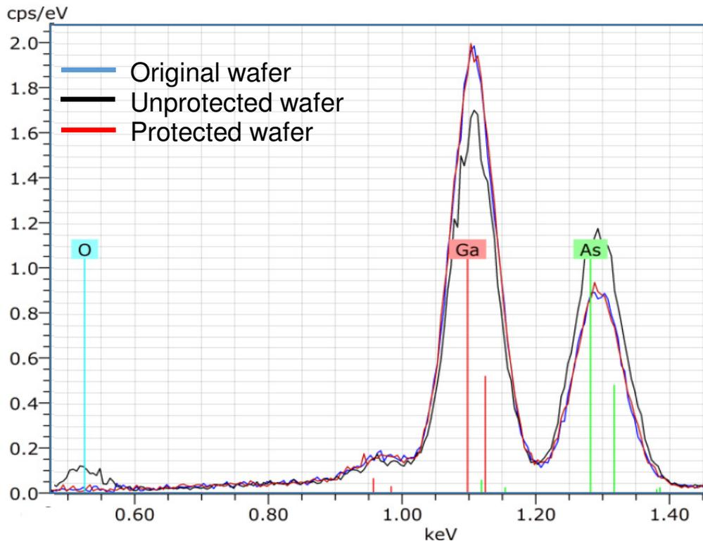
**Figure 6.7:** Energy dispersive spectra of wafers in Figure 6.3.
