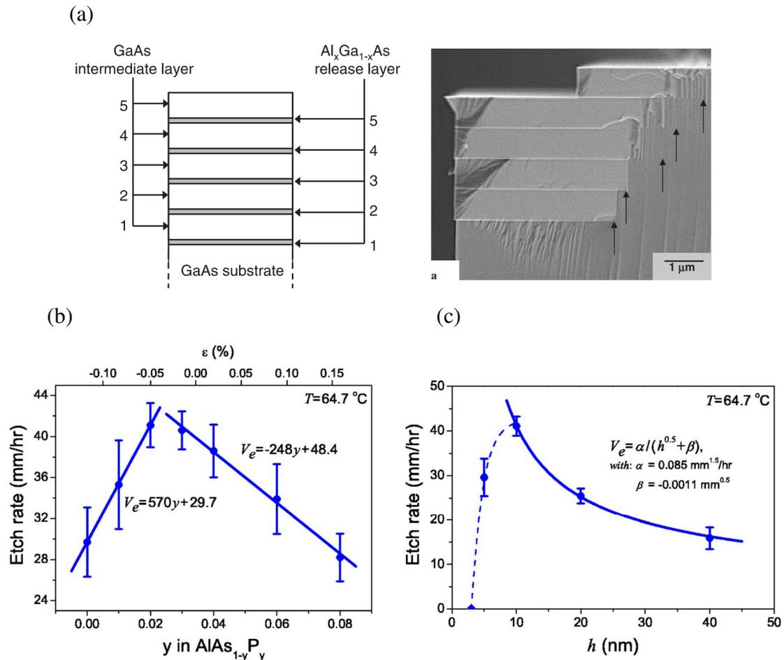
**Fig. 2.4:** Multi release layer etch test (a) Schematic of multi release layer etch method (left) and cross-sectional scanning electron microscope (SEM) image of sample (right). (b) Lateral etch rate depending on the strain of sacrificial layer. The strain was controlled by varying P composition. (c) Lateral etch rate depending on the sacrificial layer thickness. Reproduced from refs. 20 and 24.
