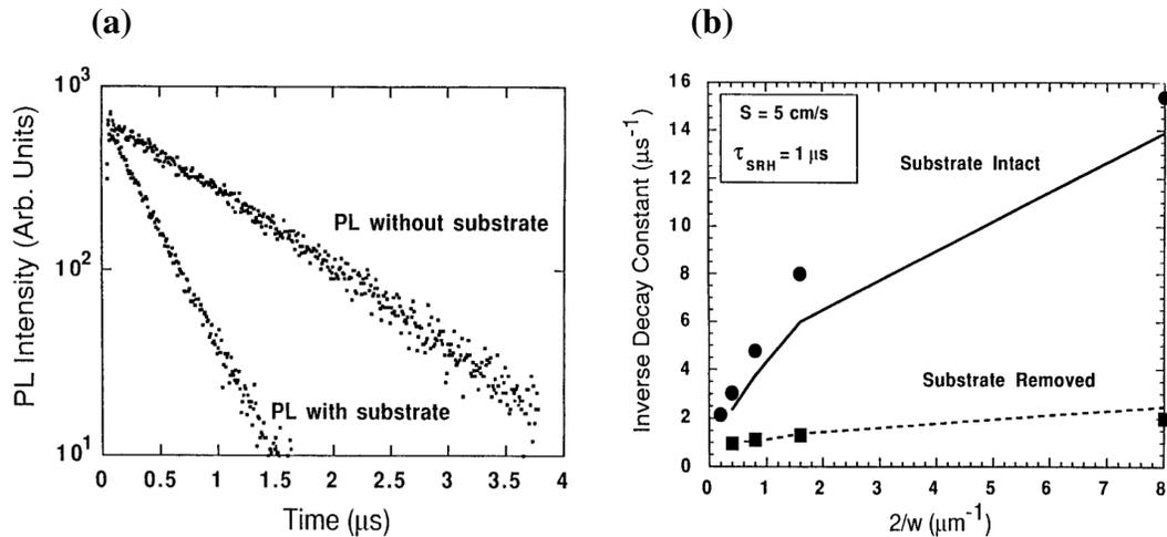
**Fig. 2.16:** Effect of substrate removal on minority carrier lifetime. (a) TRPL measurement on GaAs/AlGaAs thin film with and without substrate. (b) Inverse decay constant extracted from TRPL measurement dependence on active layer thickness. Reproduced from ref. 45.
