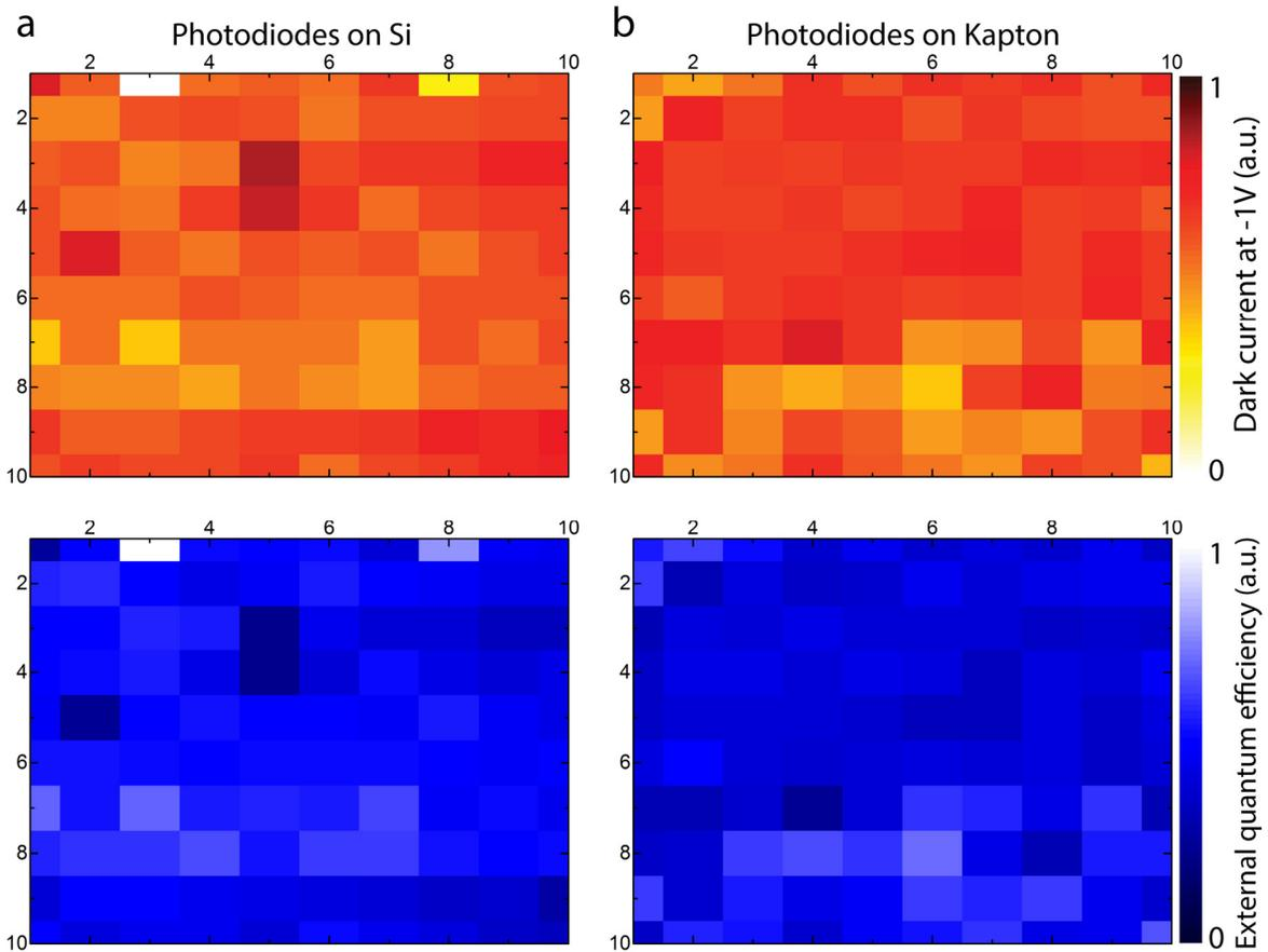
**Fig. 5.8:** Thin-film device fabrication yield. Dark current (top) and EQE (bottom) mapping of all individual photodiodes showing the fabrication yield of  $10 \times 10$  thin-film InGaAs photodiode array on (a) Si substrate and (b) Kapton substrate.
