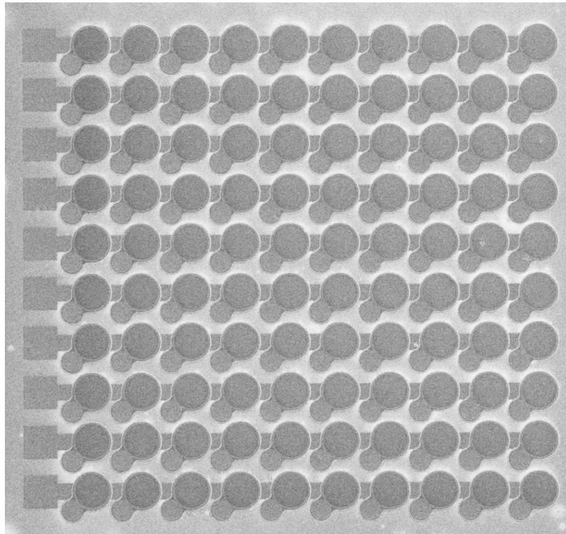
**Fig. 5.2:** SEM image of linearly connected 10×10 photodiode array fabricated on the lifted-off epi-layers on Kapton host substrate.
