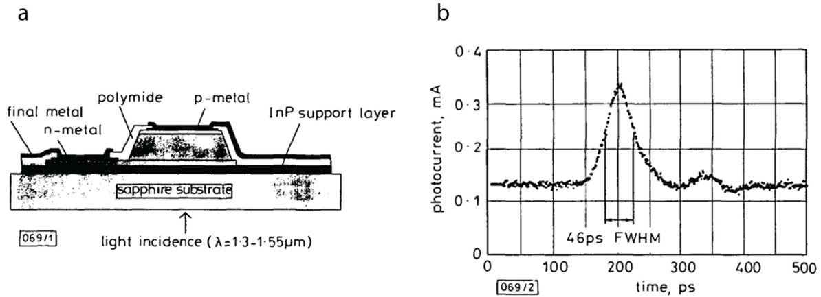
**Fig. 2.23:** ELO processed InGaAs *p-i-n* photodiode. (a) Schematic cross-section of fabricated device structure and (b) Pulse response of InGaAs *p-i-n* photodiode. Measurement shows 46 ps FWHM, and THE estimated intrinsic impulse response was 23 ps FWHM. Reproduced from ref. 56.
