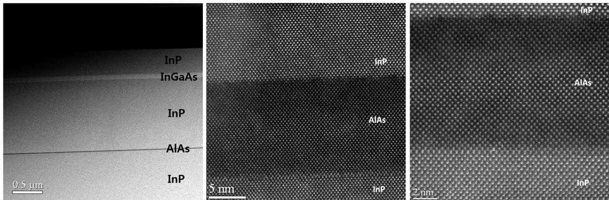
**Fig. 4.1:** Growth quality of lattice mismatched InP on AlAs layer (a) Test growth structure for InP/AlAs heterostructure (b) Atomic resolution cross-sectional transmission electron microscope images of the growth interface between the InP and (b) 3 nm thick and (c) 12 nm thick AlAs sacrificial layer with various resolution.
