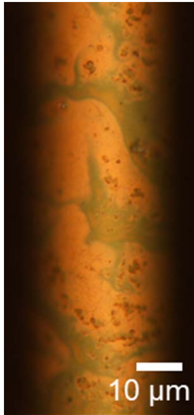
Figure 8-2. Darkfield optical microimage of drawn-capillary OFRR with C8 MPN coating.
