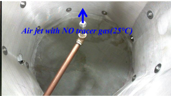
(b) Jet nozzle inside the duct
