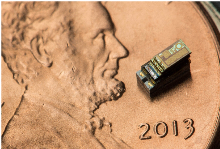
Figure 1.2: A modular 1mm 3 sensing platform [7]
