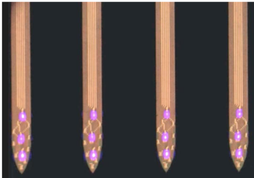
Figure 4.13: All 12 \mu LEDs lighting captured by low magnification microscope.
