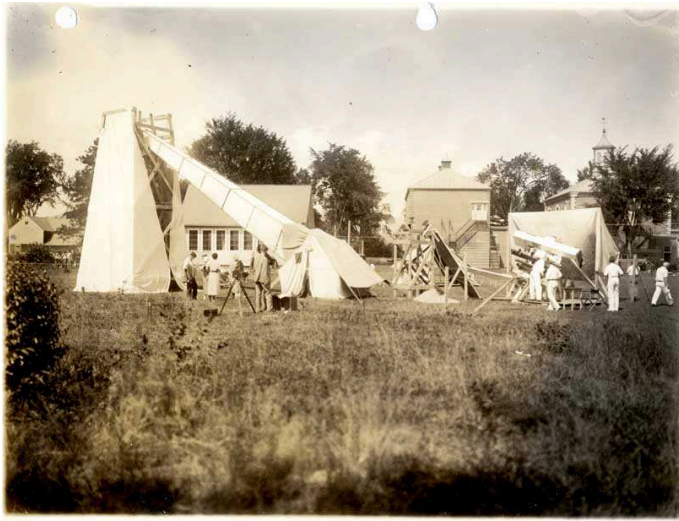
Equipment used for eclipse expedition, Fryeburg, Maine. A 40-foot portable telescope is depicted in this image.
