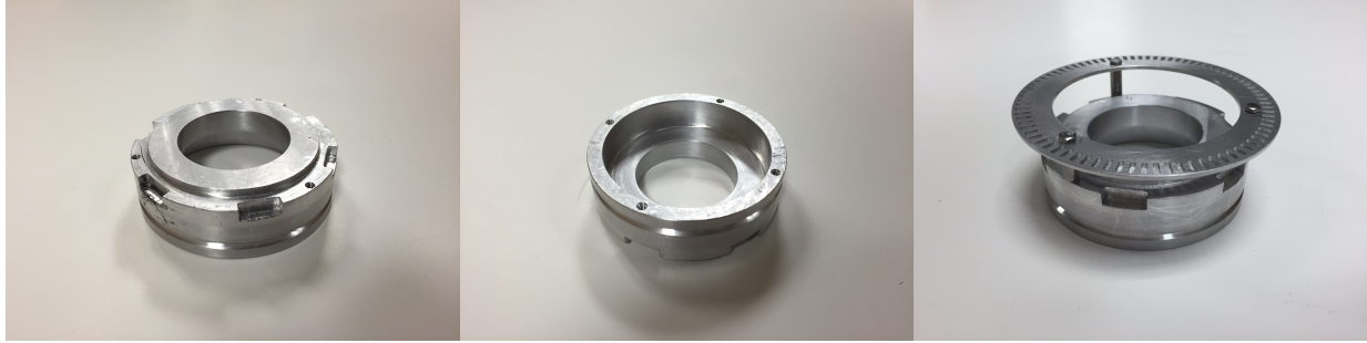
Figure 4: Left: Top of the rotor for the cryogenic model. There are six rectangular recesses for the drive magnets. Middle: Bottom of the rotor. The recess is to hold the ring magnet for the superconducting bearing. Right: Cryogenic rotor with the photo-encoder installed. The spacers raise the photo-encoder above the stator.
