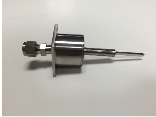
Figure 8: Stainless steel bellows for the locking mechanism. The arm on the right side tapers to a point to fit in the groove on the rotor. The left side is an adapter to fill the bellows with nitrogen gas.
