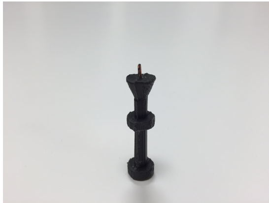
Figure 6: Cryogenic solenoid bobbin. The bobbin is made of stycast 1266 epoxy.
