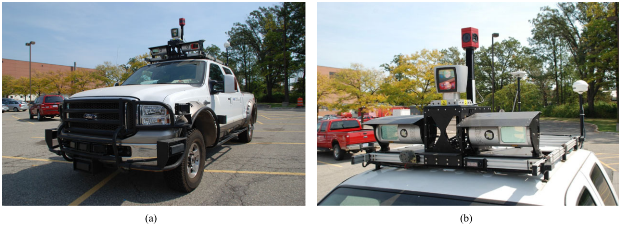
Figure 8. (a) The modified Ford F-250 pickup truck with sensor configuration as described in Pandey et al. (2011b). (b) The Velodyne HDL-64E 3D laser scanner (Velodyne, 2007) and the Point Grey Ladybug3 omnidirectional camera (Point Grey Research Inc., 2009) are mounted on the roof of the vehicle.
