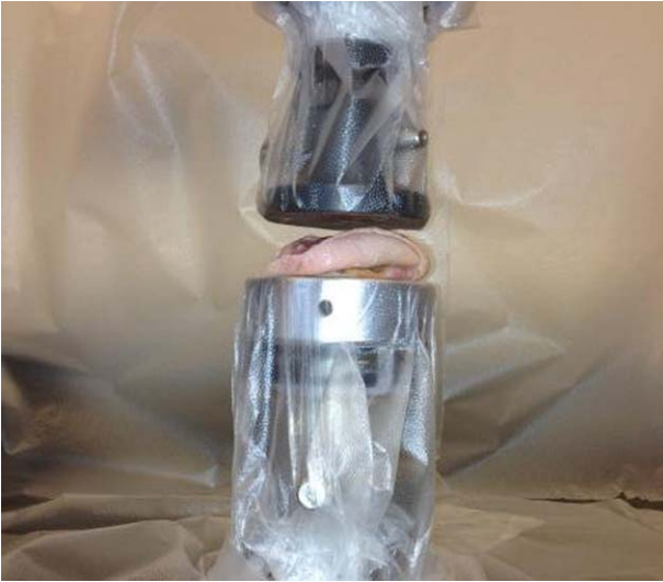
Fig. 2. The MTS Alliance RT/30 machine setup. Whole human cadaveric ears were subjected to a whole-ear helix-down compression test.
