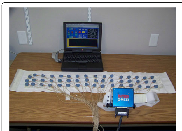
Figure 1 Multidirectional vibrotactile feedback system.
