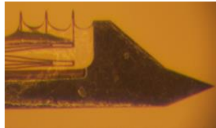
Figure 62: Images of silicon springs after four repeated starch gel dip-coats a).right after coating, during dehydration b) after dehydration
