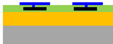
b) LPCVD polysilicon between two stacks of silicon oxide and silicon nitride. Sputter metals to form electrodes and contact pads.
