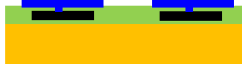
b) LPCVD polysilicon between two stacks of silicon oxide and silicon nitride. Sputter metals to form electrodes and contact pads.
