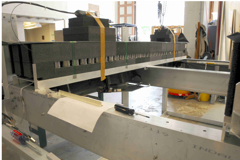
Figure 3.6: One fully assembled crystal C-channel rests on top of CREST's aluminum chassis. Picture courtesy of R. Northrop. Each silver tube is one crystal/PMT assembly.
