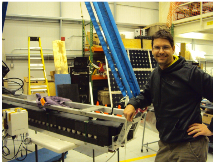
Figure 5.53: Professor Scott Wakely of University of Chicago pauses while examining a CREST C-channel on the ground level of Hangar 096 at the LDB facility near McMurdo Station, Antarctica. The aluminum jig used to lift the channel was designed by Alex Shroyer. This allowed us to safely and quickly remove the C-channels from the instrument for maintenance.
