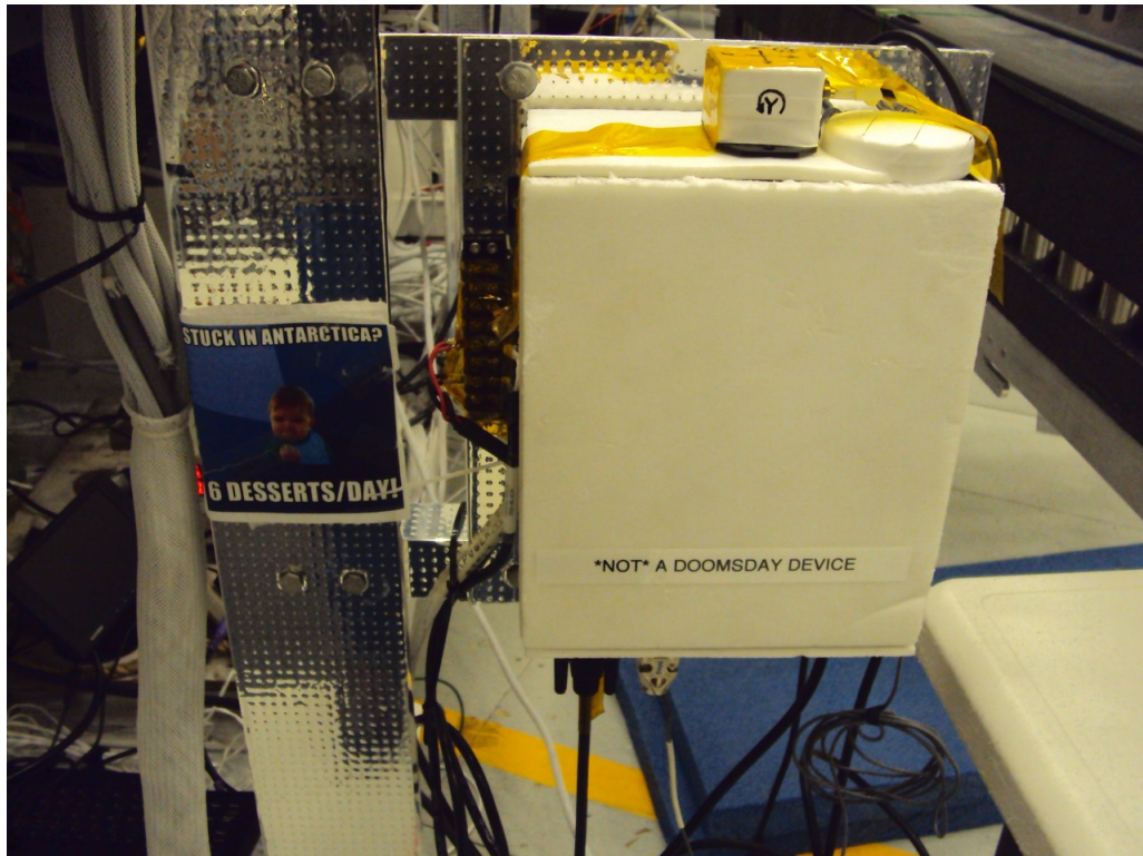
Figure 3.39: The magnetic field sensor provided by the University of Michigan Atmospheric Oceanic and Space Sciences department. It flew on board CREST and recorded the three local components of magnetic field strength.
