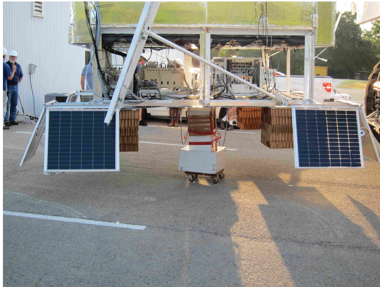
Figure 5.28: CSBF personnel fit CREST with crush pads (stacks of cardboard tubes), the ‘skirt’ of solar panels that will power the SIP and the ballast container (center). The SIP is shown here mounted in the lower right portion of the instrument. The white-bearded fellow at far left facing the camera is CSBF’s Dave Sullivan, who ran LDB during most of our time in McMurdo and was of immense help to CREST in many ways during our time in Palestine and in Antarctica. Photo by M. Geske.
