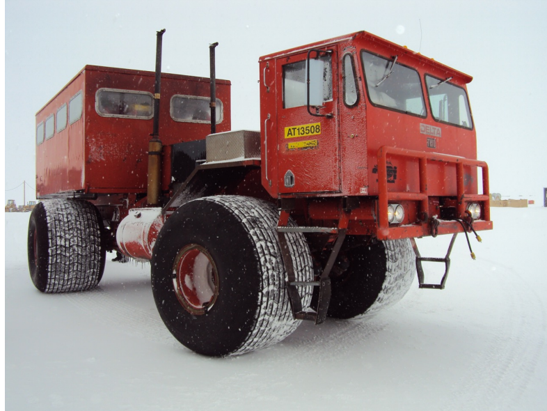
Figure 5.63: A ‘Foremost Delta Two’ transport vehicle. Supposedly the safest transportation vehicle for ice roads, its light weight and immense tires make it susceptible to getting stuck in ice potholes in warmer temperatures, or whenever the driver spins the tires too quickly (see the next Figure). Riding in the undulating toolshed hitched back of one is a rapid way to lose your lunch. If one had to sprint 100 meters to steal your buddy’s seat aboard Ivan the Terra Bus thereby dooming them to a ride aboard the Delta, one did so without regret. Overall, McMurdoans least-favorite mode of transportation vehicle, barely beating out “on foot.”
