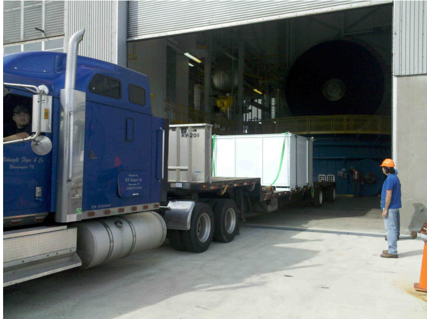
Figure 5.5: CREST is delivered via flatbed truck to the Plum Brook testing site on 6/14/2011. The white box is the aluminum shipping container constructed and painted at Indiana University. Visible in the background is the upper section of the vacuum chamber with the mushroom hatch in the open state.
