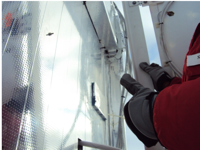
Figure 5.109: The foam block covering the power cable pass-through hole during our first launch attempt.
