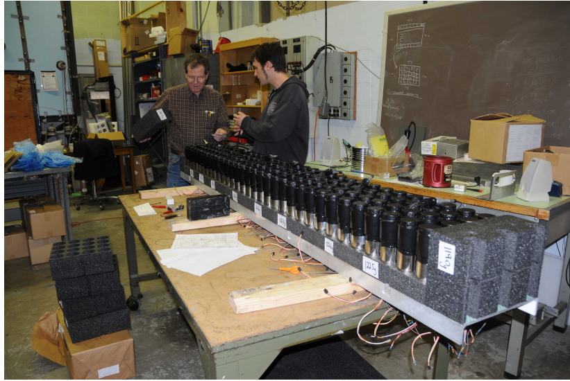
Figure 3.5: Chuck Boyer and Alex Shroyer assembling a crystal C-channel at the Indiana University high bay in Fall 2010. On the blackboard to Alex's right the hexadecimal numbering scheme for tubes within a Sedecim has been drawn.
