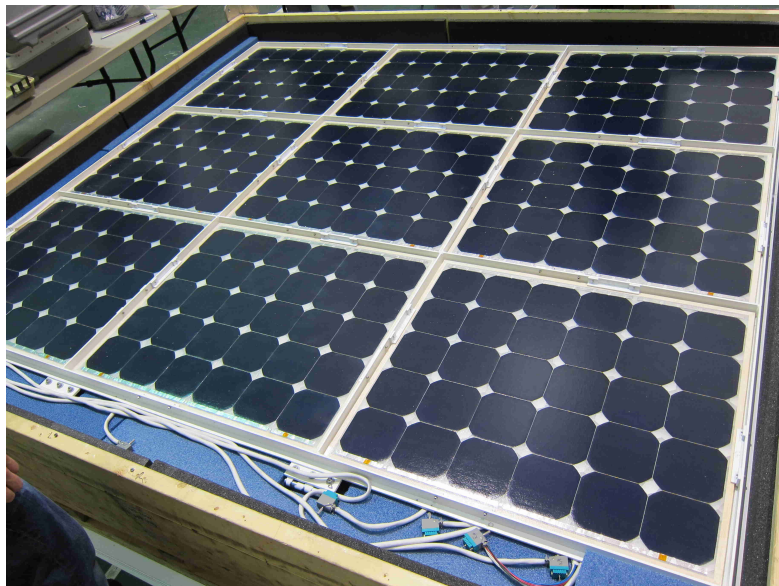
Figure 5.25: One of CREST's solar panel wings awaits attachment to the instrument in its shipping container. Photo by M. Geske.
