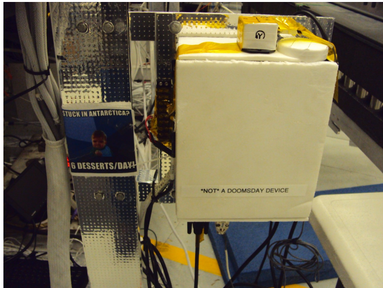
Figure 5.67: The magnetic field sensor supplied by the University of Michigan Department of Space Science. Data taken by this device is presented in Section 5.4.8.
