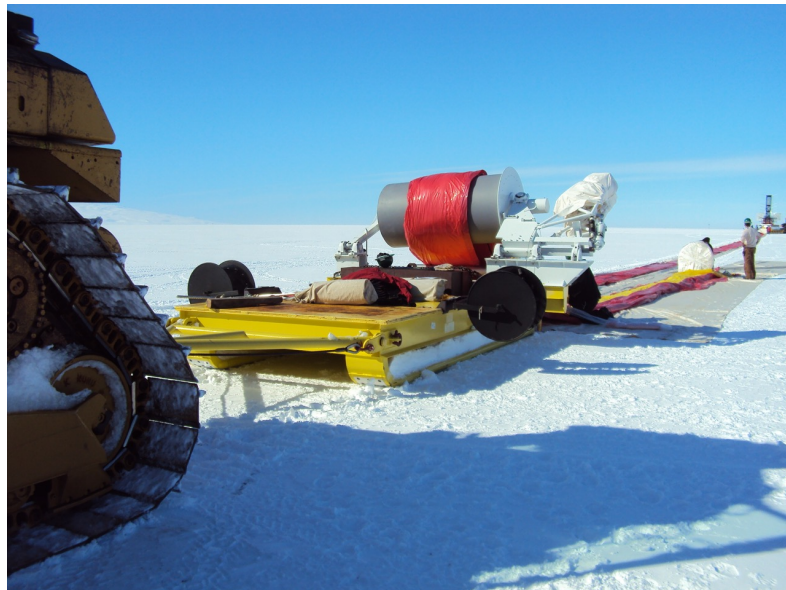
Figure 5.126: A massive spool unwinds the tether that will connect CREST to its host balloon.
