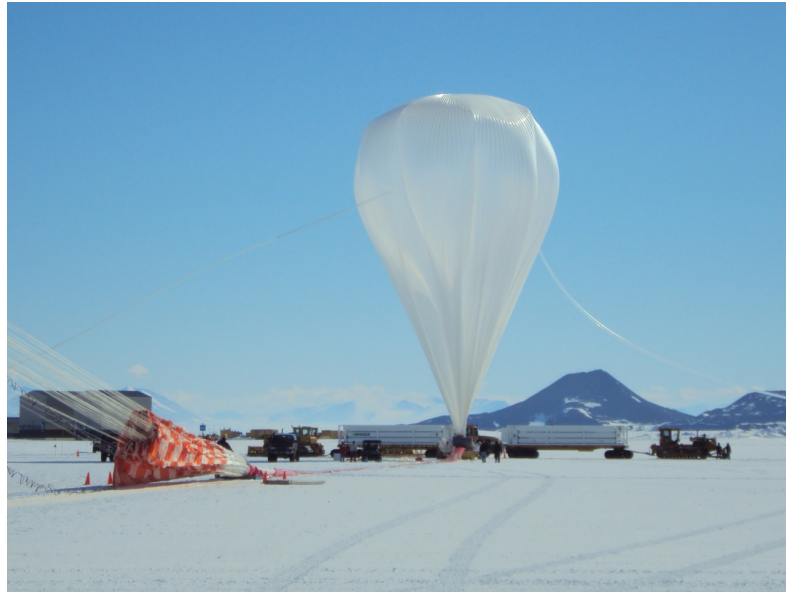
Figure 5.134: The balloon continues to inflate via the fill tubes (white wisps coming out either side of the inflated portion of the balloon). The loud ‘whoosh’ of rushing helium dominates the scene. At left, CREST’s orange and white parachute lies in wait.
