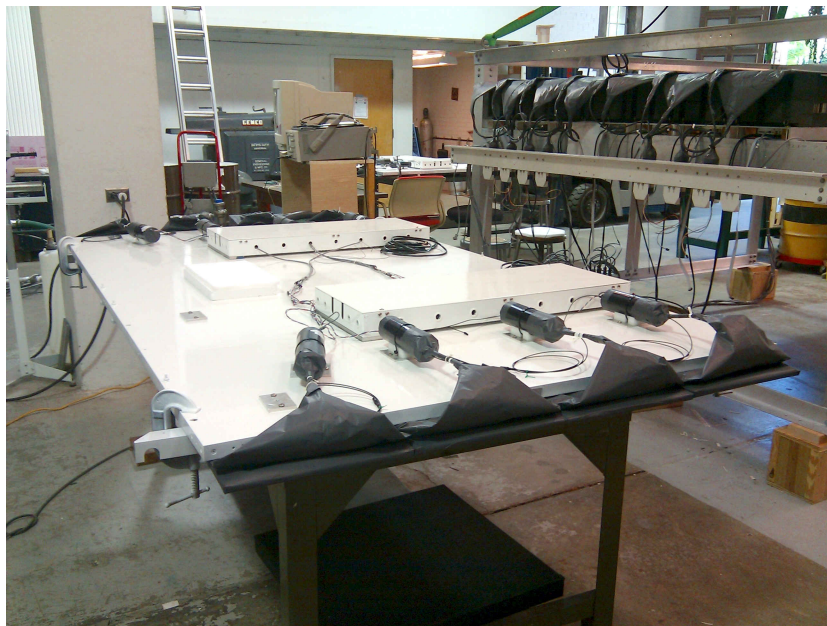
Figure 3.28: The veto “honeycomb” before mounting to the instrument, upside-down, supporting four of nine bottom veto paddles with FOLGA’s mated to their PMTs. The white veto boxes are the veto system’s equivalent of the crystal C-channels; each would later hold four STAC/AFE/SVI electronics modules. Picture by R. Northrop.
