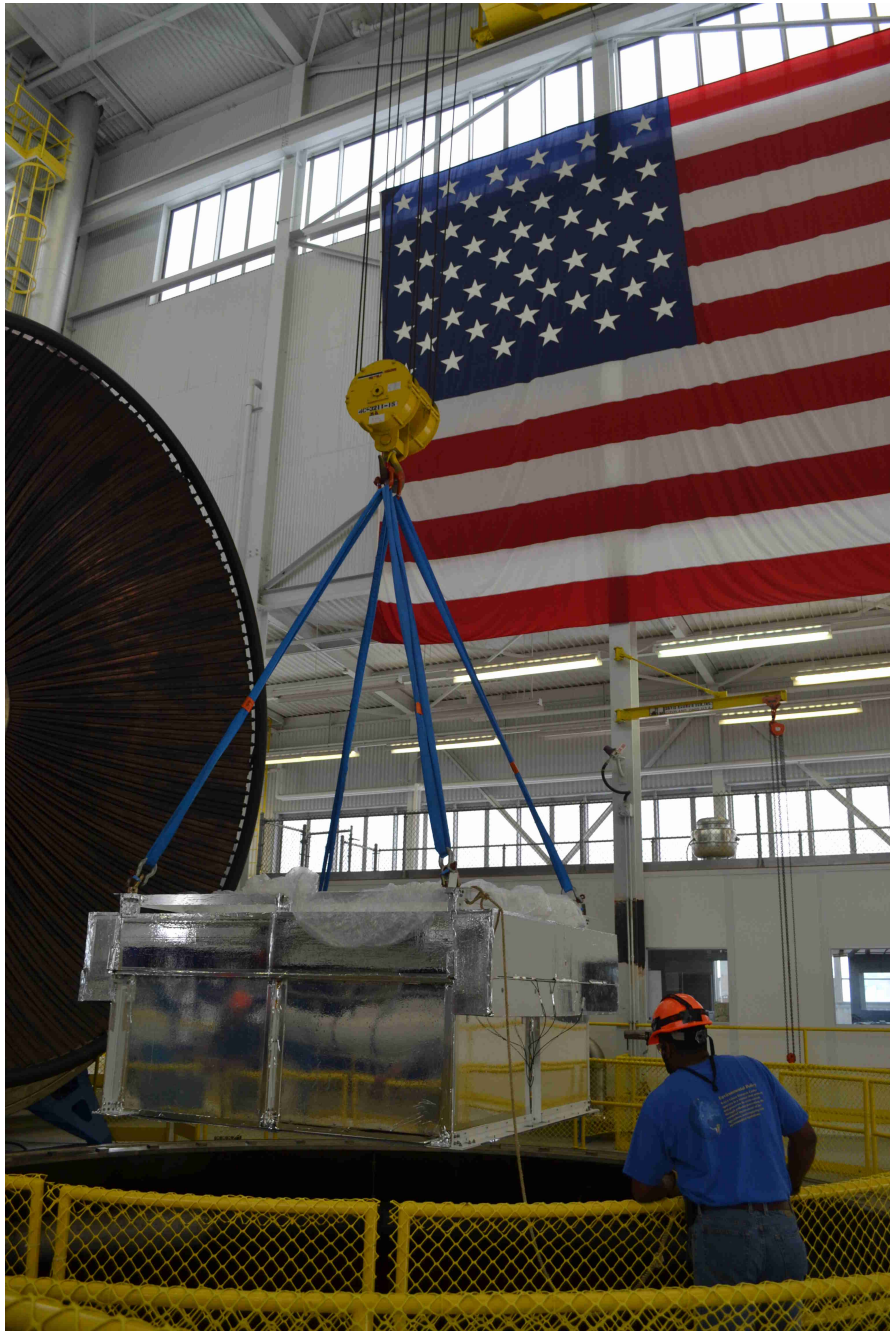
Figure 5.7: CREST is lowered via crane (a Critical Lift Procedure) into the testing chamber at Plum Brook on 6/15/2011.
