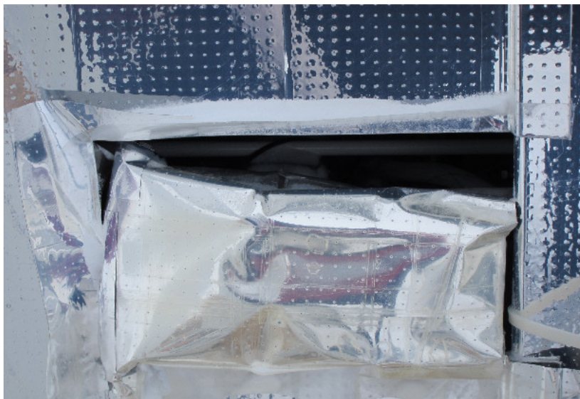
Figure 5.94: The foam block used to cover the power cable access did in fact shrink during flight. Photo by J. Ameel (during recovery).
