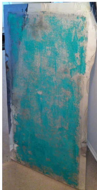
Figure 5.3: A ruined panel not used in the Plum Brook test constructed by laminating aluminized mylar sheeting onto foam backing. When applied prematurely (before allowing the glue to dry) a reaction between the aluminum, glue and/or foam occurs resulting in the formation of an intriguing green pattern. J. Musser dubbed this beautiful mistake “RTFM.”
