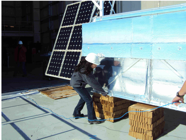
Figure 5.54: Nahee Park inspects CREST's thermal outer covering during a rollout test at LDB. Visible in the foreground is CREST's flight computer's umbilical (ethernet) cord, which we had to subsequently wean ourselves off of prior to flight.
