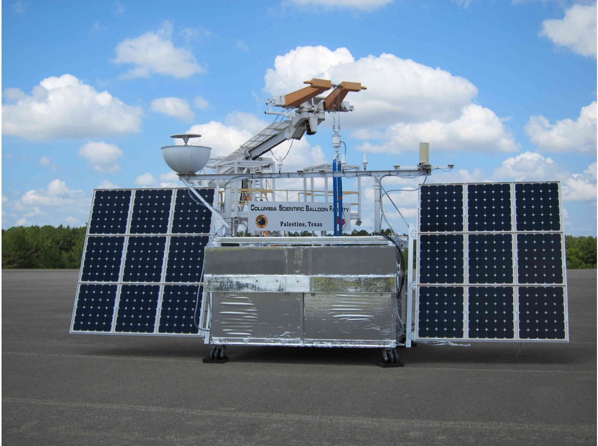
Figure 5.33: CREST on the flight pad at CSBF following our successful hang test. Clearly visible on the lower lefthand thermal panel is a circular region of the aluminized mylar sheeting which bubbled off of the panel's surface during the low pressure portion of the Plum Brook thermal/vacuum test. These panels were replaced in McMurdo, along with most of the rest of CREST's thermal shield. The new panels were laminated with perforated silverized teflon tape rather than aluminized mylar sheeting, both to avoid this failure mode and for improved thermal performance.
