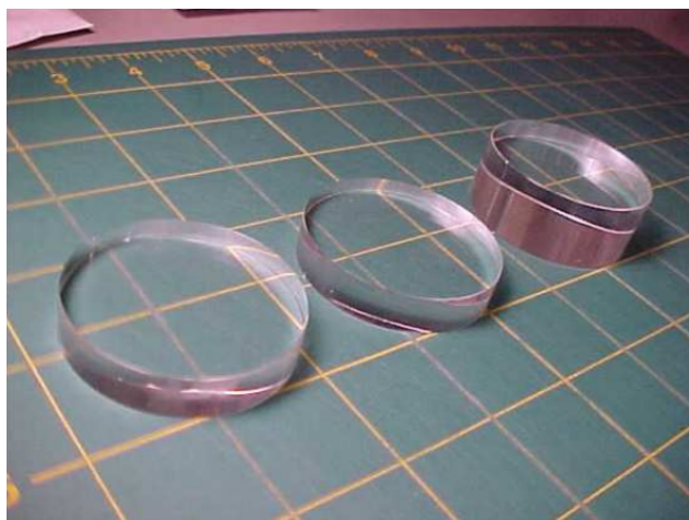
Figure 3.7: Picture of two 1 cm thick and one 2 cm thick BaF 2 crystals supplied by Proteus. Picture by A. Yagi [66].
