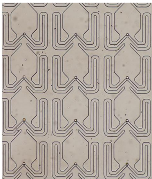
Figure 17: Single cell microwell subset with capture SKOV3 single cells.
