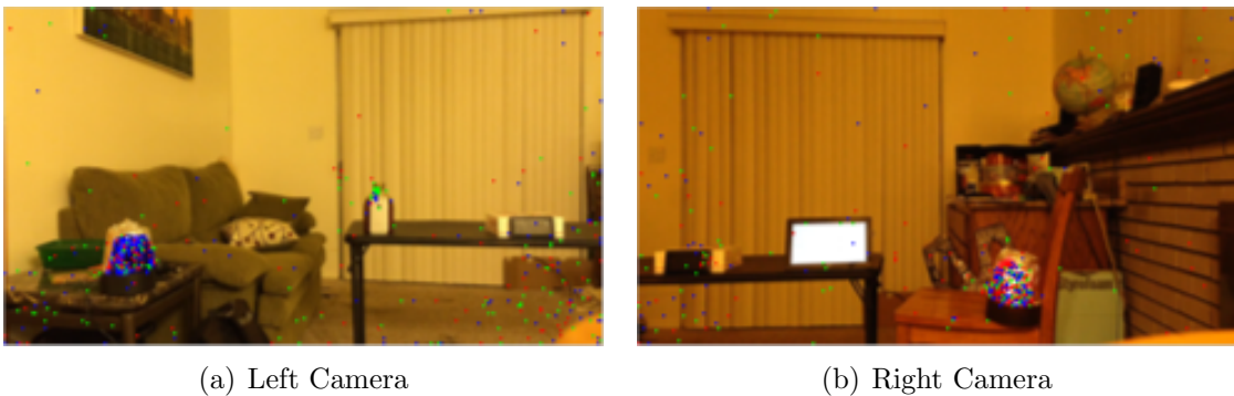
Figure 4.12: Top 3 thresholded empirical CCA canonical vectors overlaid on the original scene after 800 frames as computed in (4.9). The red pixels correspond to the vector with the highest correlation, the green pixels correspond to the vector with the second highest correlation, and the blue pixels correspond to the vector with the third highest correlation. We use a threshold of \log(p)/\sqrt{p} where p = 32400 pixels.
