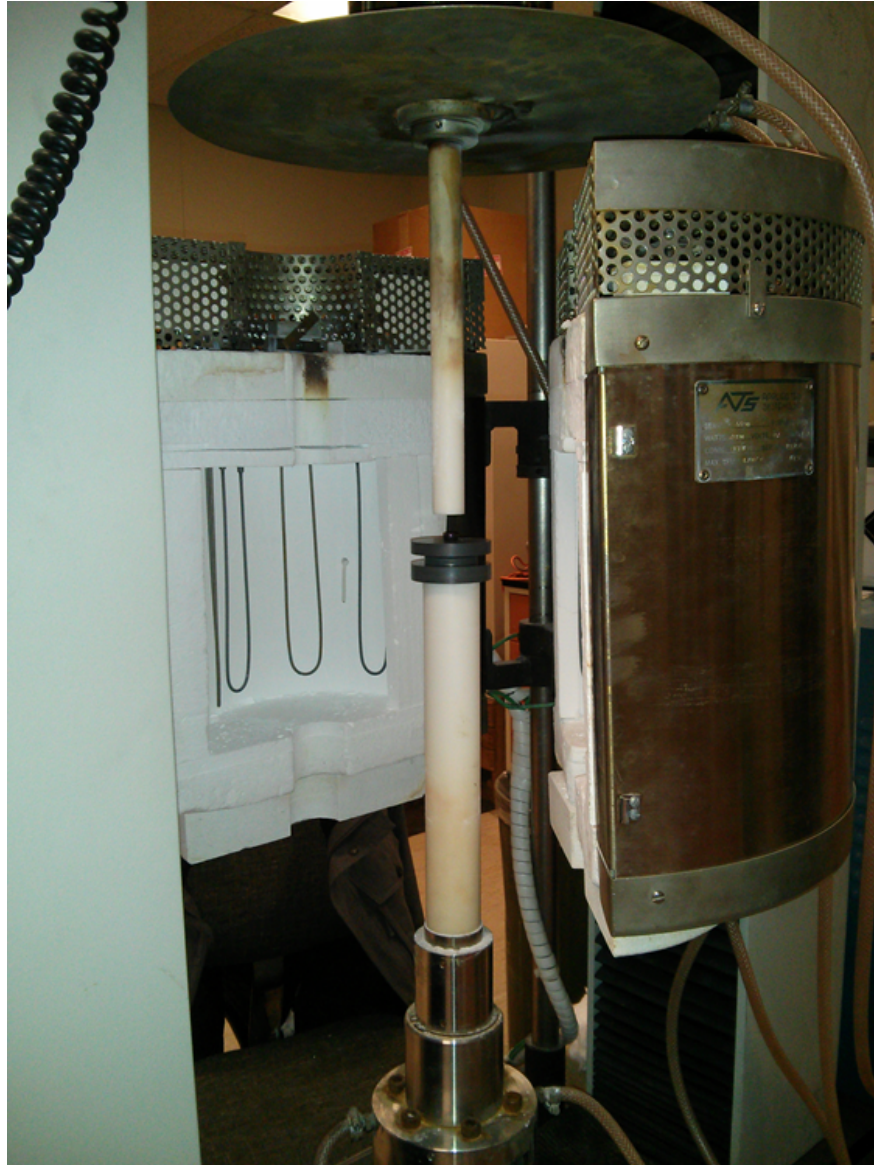
Figure 5.18: Testing apparatus used for elevated temperature ring-on-ring biaxial flexure.
