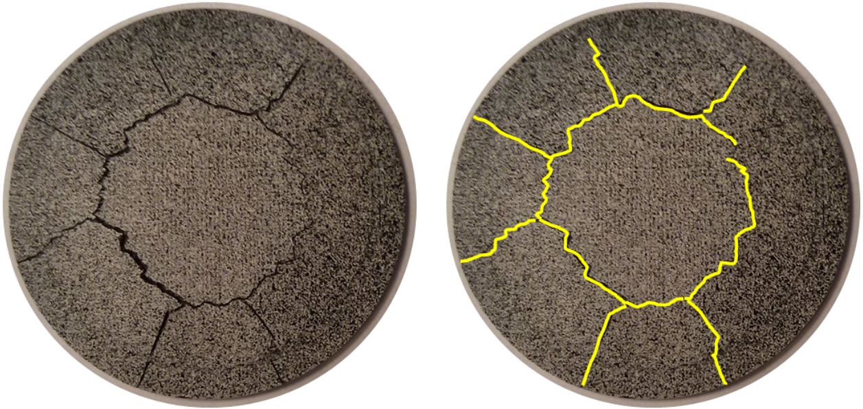
Figure 5.10: Tension side of a room temperature specimen, exhibiting a central punch-out failure mode
