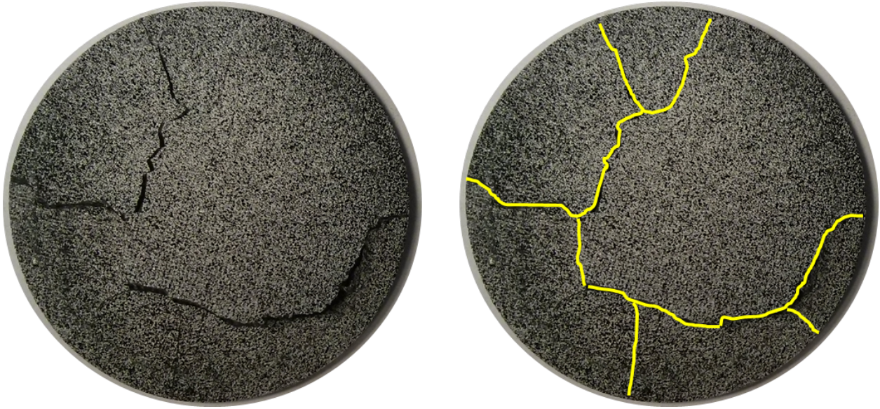
Figure 5.12: Tension side of a room temperature specimen, exhibiting a flap-like punch-out failure mode
