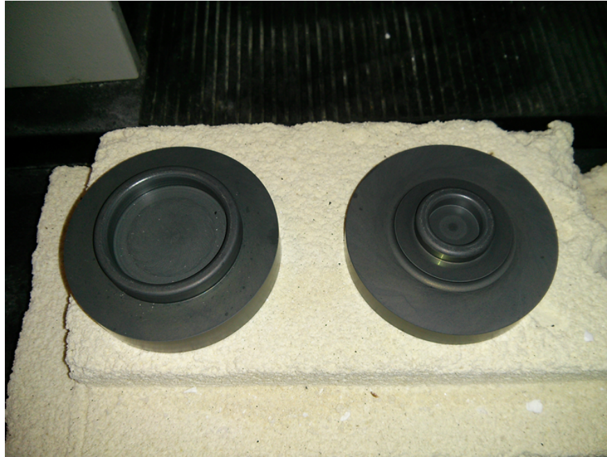
Figure 5.19: Close-in view of the elevated temperature ring-on-ring biaxial flexure fixtures.
