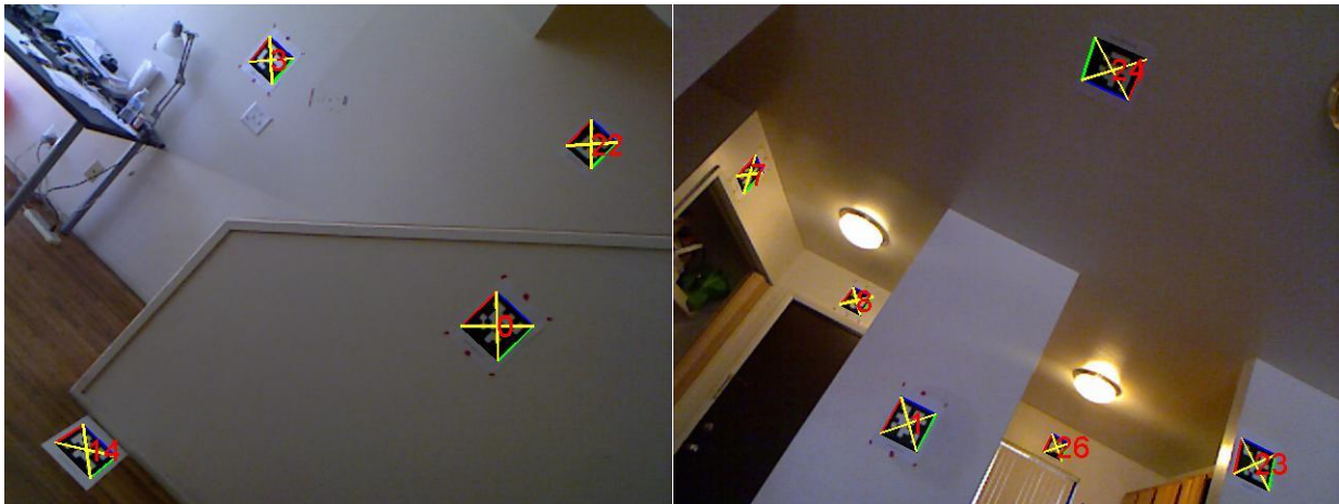
Figure 8-2: Example photos and corresponding marker detections for as-built modeling.
