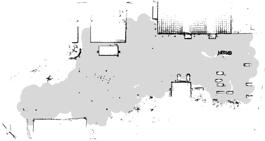
Figure 2.1: Rasterized map of Keswick Barracks. The 180 x 100 m map was produced with a mean processing time of 1.3 seconds on a single 2.53 GHz core. Permanent structure is shown in black; known free space in gray; unobserved in white.
