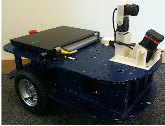
Figure 4.2: Sensor configuration. Co-location of the LIDAR and camera enables co-registration of both data streams.
