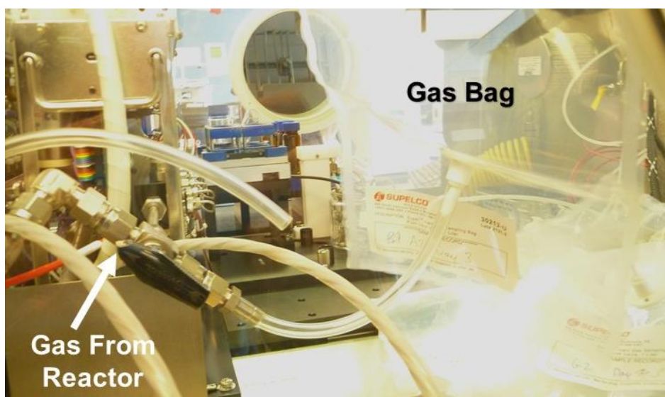
Figure 4.5. Sampling of Reaction Headspace from Parallel Reactor to Gas Bag
