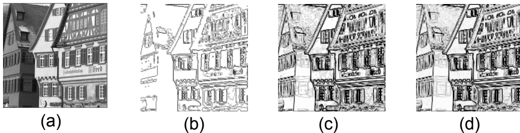
Figure 6.5: Progressive precision results for edge detection: (a) input image; output image after (b) 4, (c) 32, and (d) 256 clock cycles.
