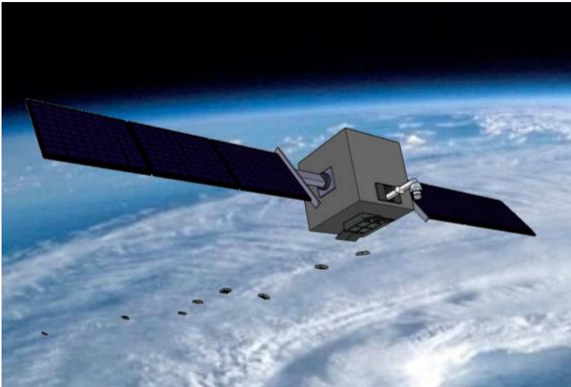
Figure 1.1: Visual illustration of small satellites being deployed from a larger satellite in Earth orbit. The background image is a photograph of hurricane Isabel taken from the International Space Station (ISS) [10]. Photo courtesy of NASA.
