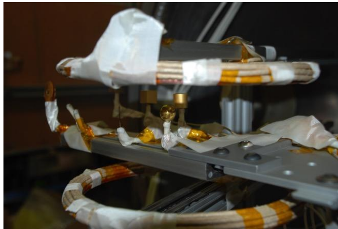
Figure 4.10: Picture of the probes in the Helmholtz coil in Test 3. The coil radius was 7.6 cm.
