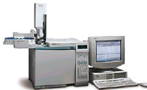
Fig. 1.2: (a) Schematic of conventional GC [Blu12]. (b) A commercial benchtop GC model (Agilent 6890) [Sci15].
