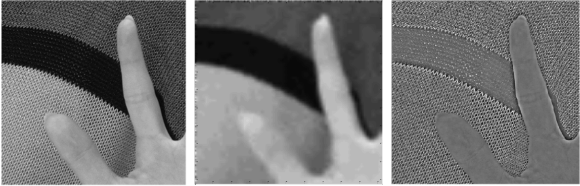
Figure 7.7: Left image: Original Image. Middle image: Low frequency component (coded at 0.0374 bpp). Right image: High frequency component.
