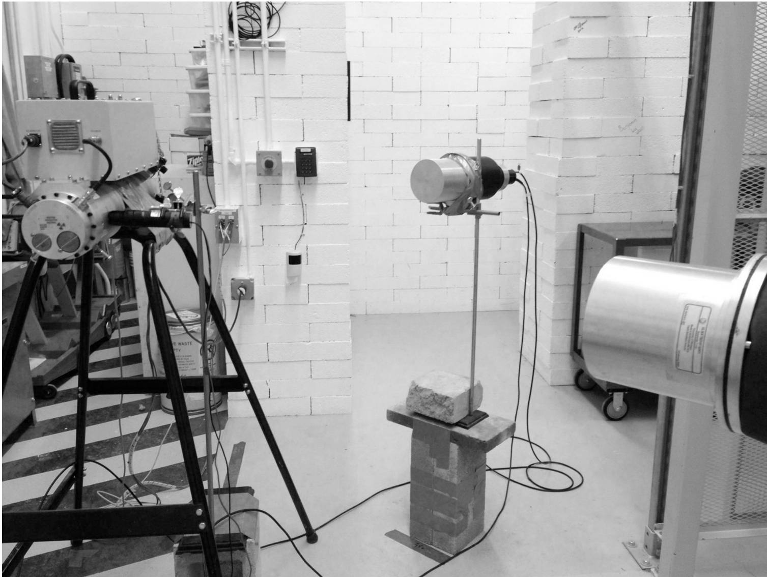
Fig. 7.4: A picture of the laboratory setup for the unattenuated neutron transmission measurements, with the stop-1 detector in the foreground and start detector and D-D generator to the left.
