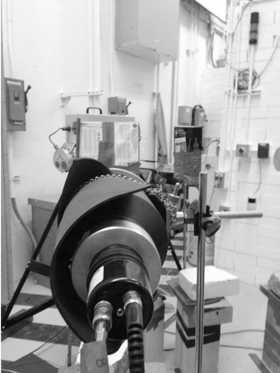
Fig. 7.5: A picture of the laboratory setup for the paper neutron transmission measurements, behind the stop-1 detector, facing the paper transmission target and D-D generator.
